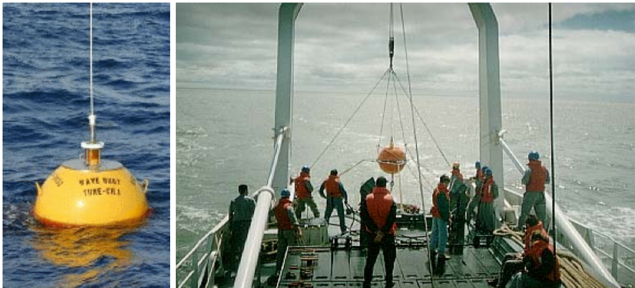
Figure 1. Wave rider buoy, left, and release of buoy, right, in October 1996 [8].
