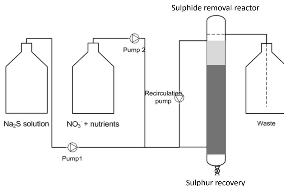
Figure 1. Schematic laboratory scale EGSB reactor
