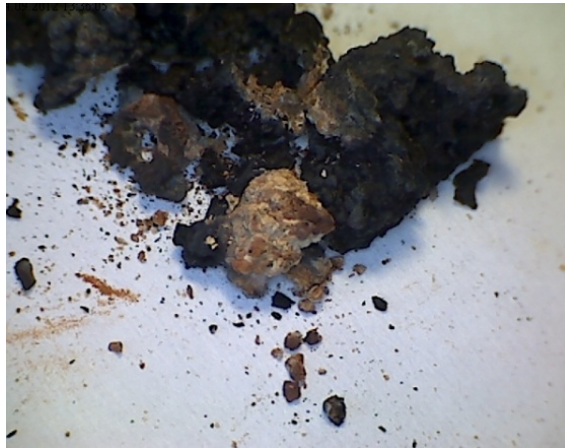
Figure 4. Elemental sulphur recovered at the bottom of the reactor, after the ignition of settled sludge at 550 °C
