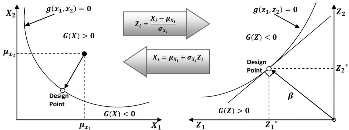
Figure 1. Failure surface transformation from physical ( $X$ ) to standard normal space ( $Z$ ) for a non-linear safety margin involving two independent Gaussian variables
