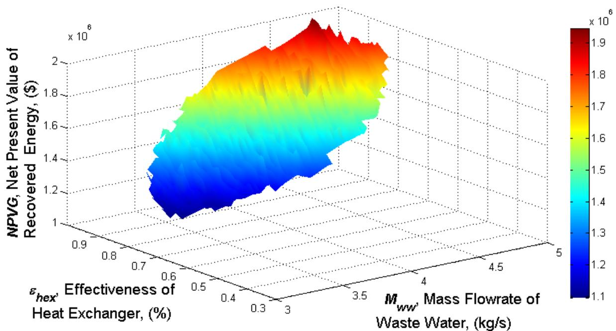
Figure 3. Overall performance space showing the expected net present value of the recovered energy during the life cycle of a heat exchanger
