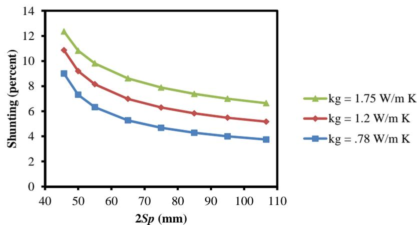
Figure 6. Loop thermal shunt between legs as function of spacing and grout conductivity
