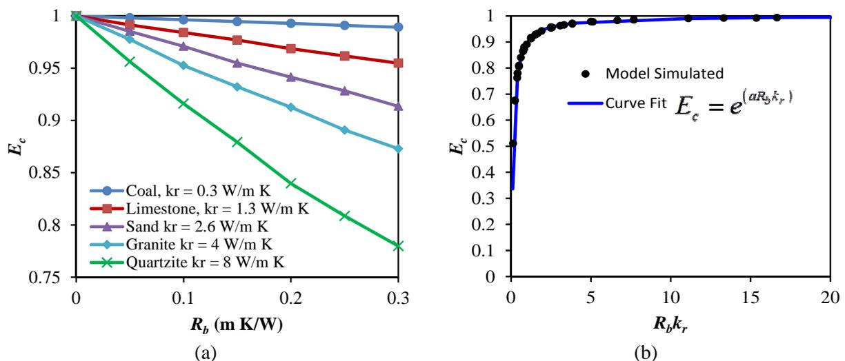
Figure 5. Thermal well efficiency ( $E_c$ ) as a function of borehole thermal resistance ( $R_b$ ) and the thermal conductivity of the surrounding geologic formation ( $k_r$ )
