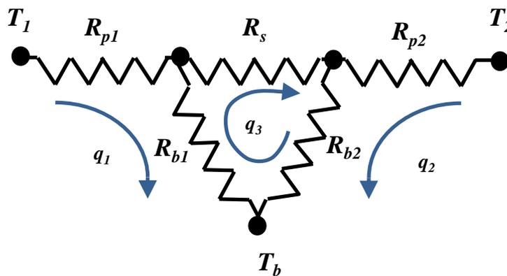
Figure 2. Resistance network model representing wellbore heat transfer
