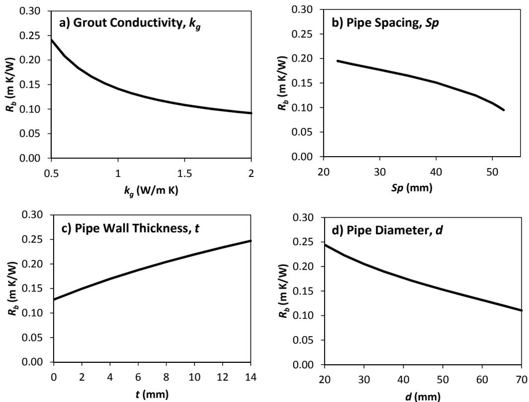
Figure 4. Borehole thermal resistance predicted by the model as a function of grout thermal conductivity, pipe spacing, pipe wall thickness, and pipe diameter
