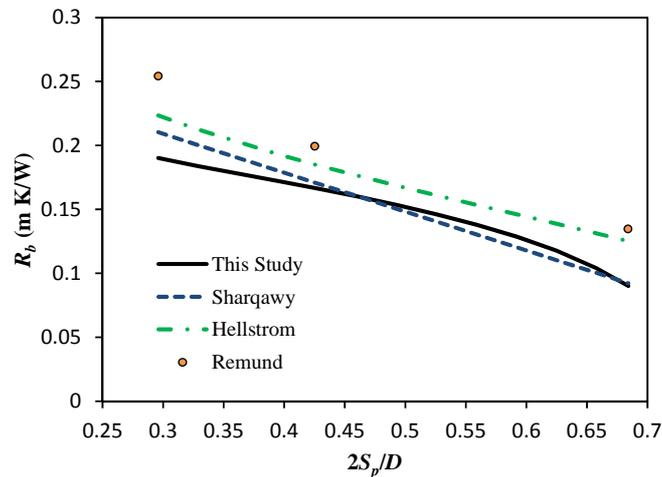
Figure 3. A comparison of effective borehole resistance ( $R_b$ ) predicted by this study, a finite-element model (Sharqawy [4]), an semi-infinite analytical model (Hellström [6]), and empirical observations (Remund [1])
