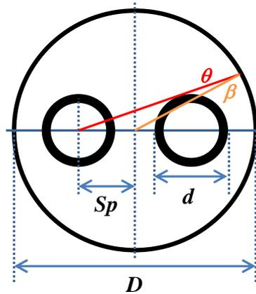
Figure 1. Cross-section geometry of a typical closed-loop heat exchange well. Dimensional parameters  $D$ ,  $d$ , and  $Sp$  refer to the borehole diameter, pipe exterior diameter, and pipe spacing, respectively. The occultation angles  $\theta$  and  $\beta$  are also shown
