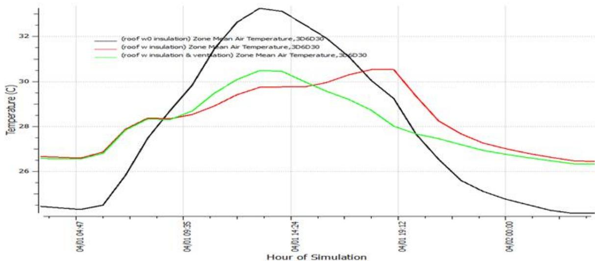
Figure 8. Simulation data shows the improvement of internal air temperature by implementing the retrofit design
