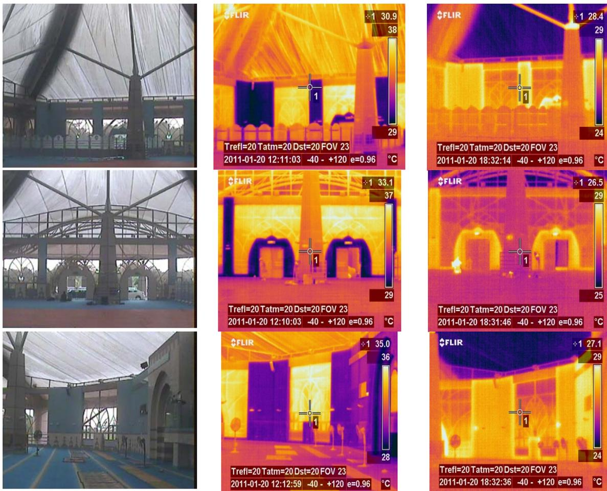
Figure 6. the thermal images of different surfaces at 12 noon compared to 6 pm
