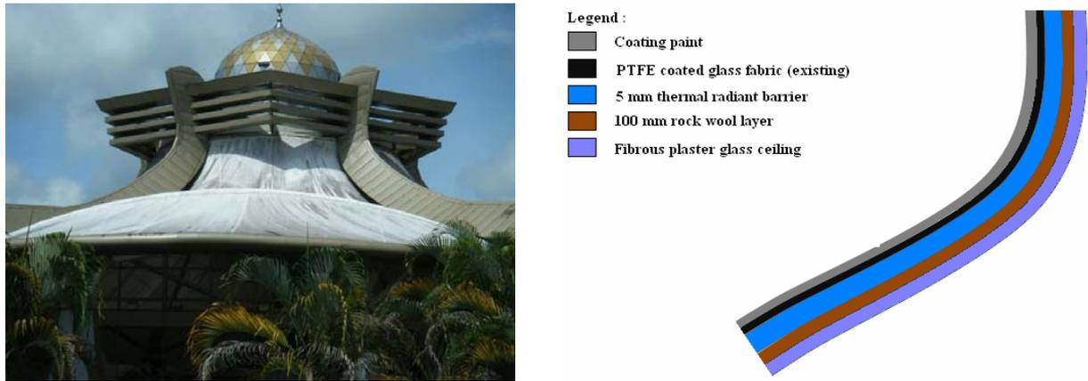
Figure 7. Proposed insulation materials for the roof
