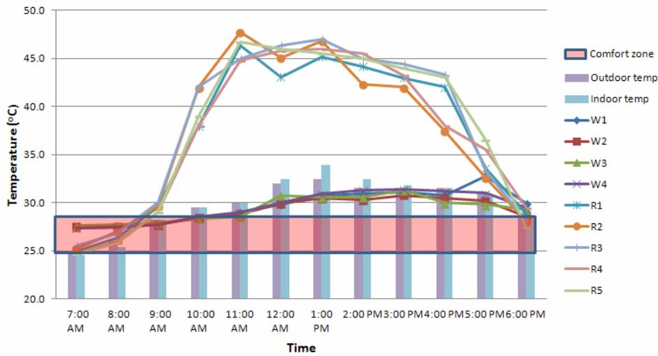
Figure 3. Surface temperature of the mosque
