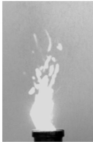
Figure 7. Combustion of olive cake particles having sizes ranging between 200 $\mu$ m and 350  $\mu$ m
