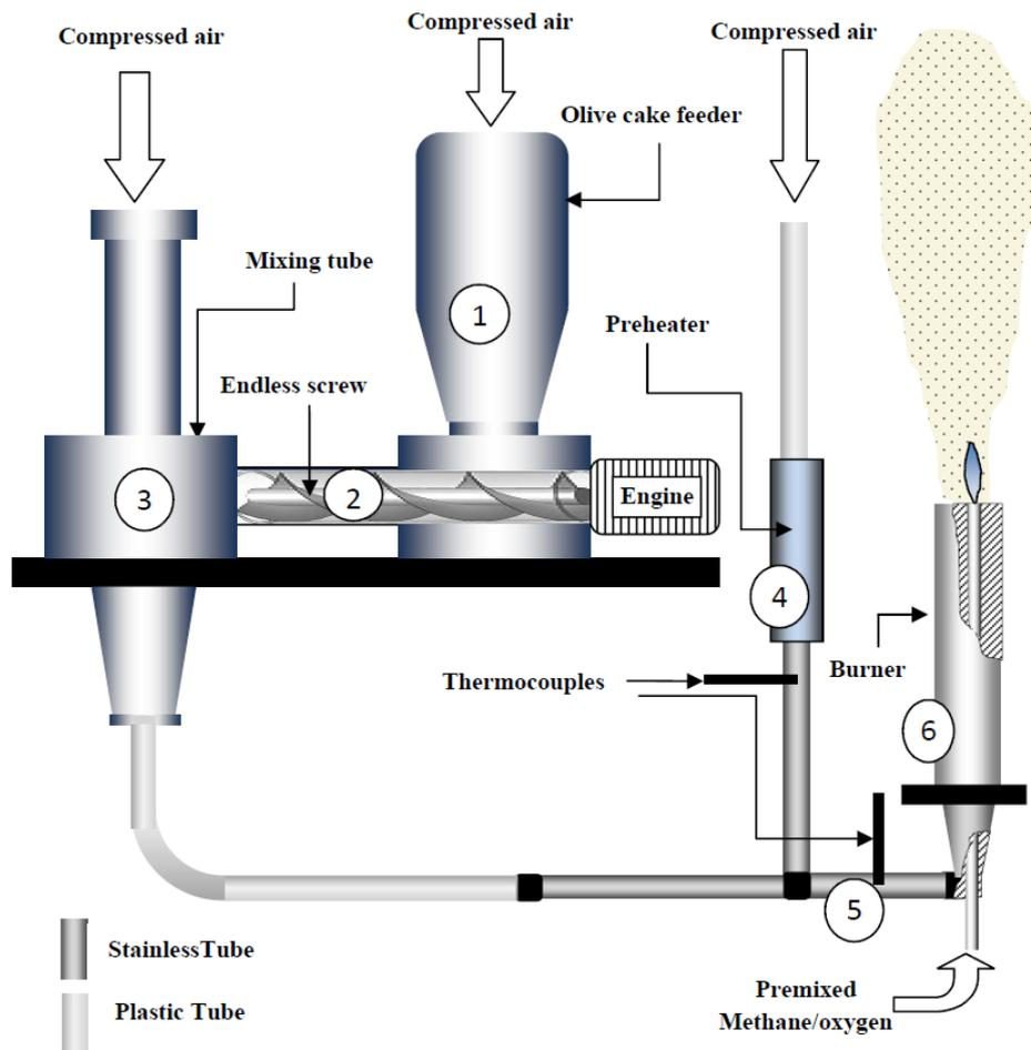
Figure 1. Schematic diagram of the pilot plant used for pulverized olive cake combustion
