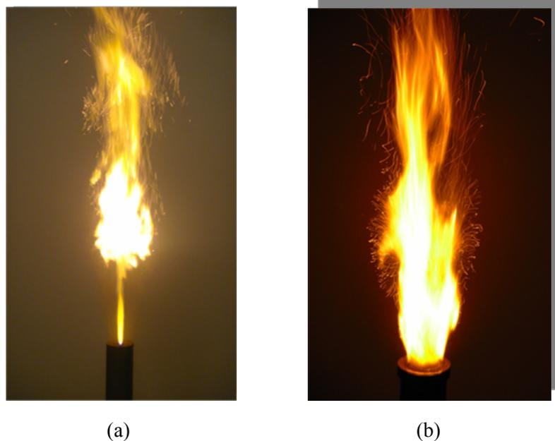
Figure 5. Olive cake flame controlled by a central pilot flame (a), Olive cake flame controlled by an annular pilot flame (b)
