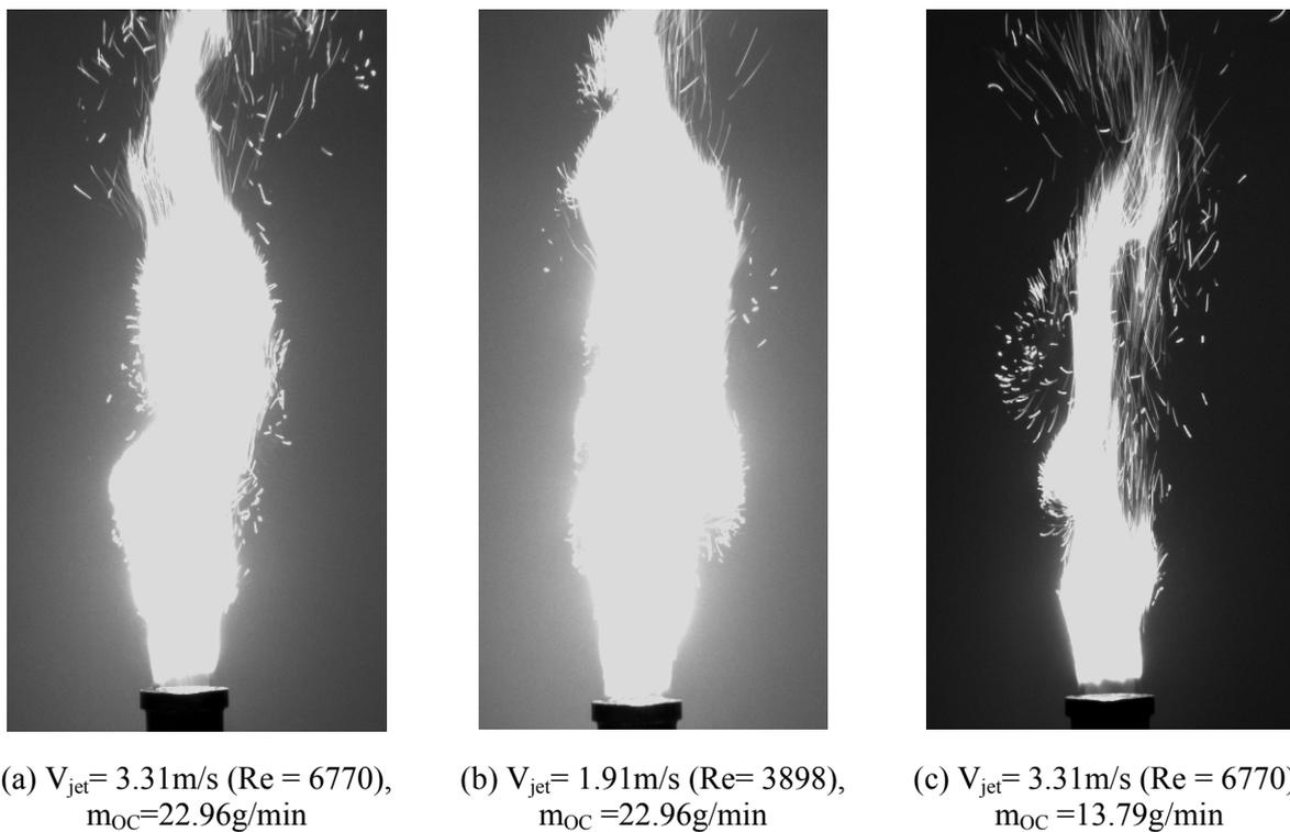
Figure 6. Direct photographs of olive cake flame for various input conditions
