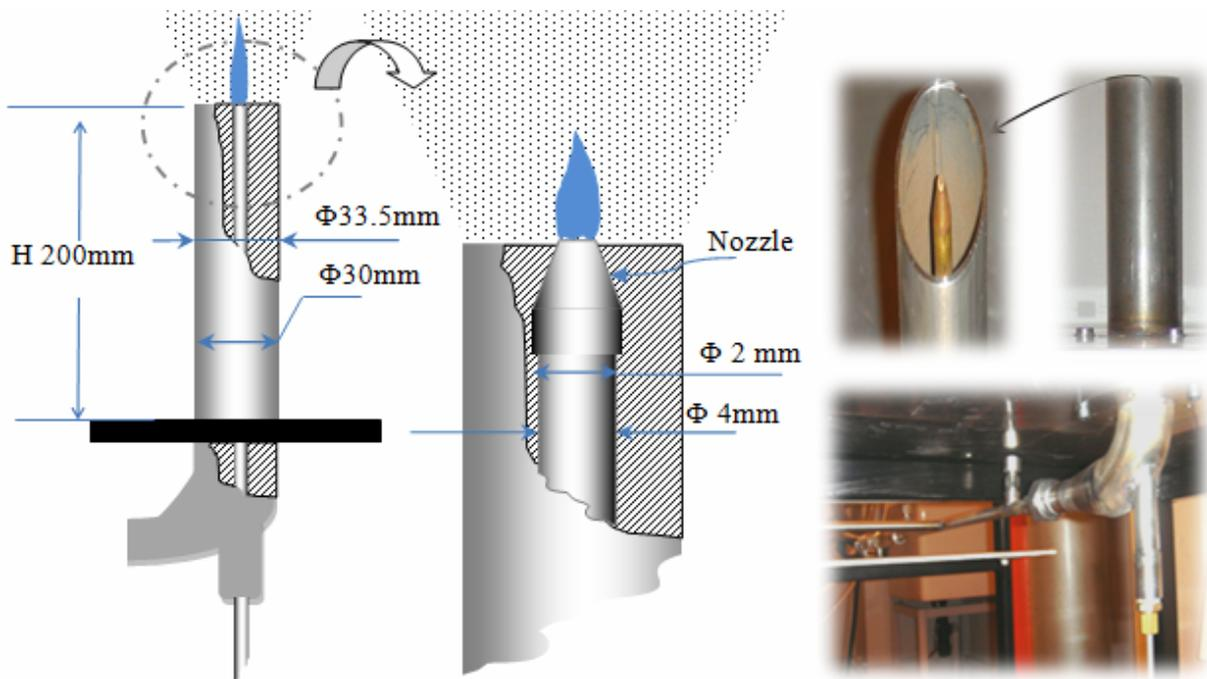
Figure 2. Dimensional details of the main burner and the central premixed pilot flame
