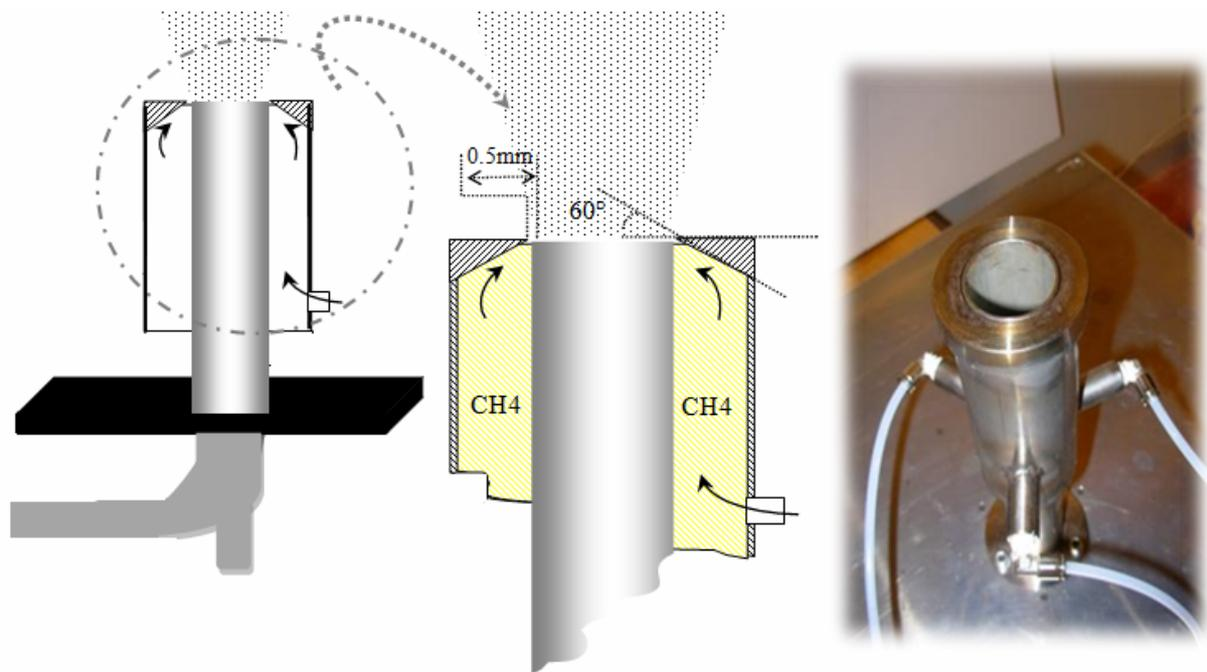
Figure 3. Schematic of the annular diffusion pilot flame
