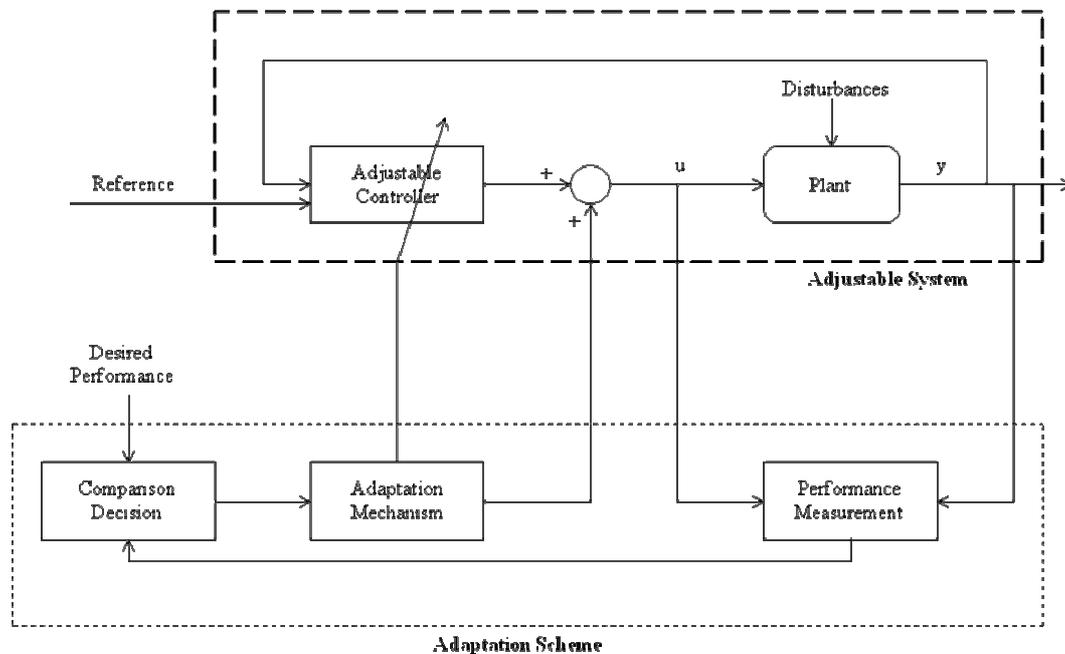
Figure 1. Basic configuration of adaptive control system [38]
