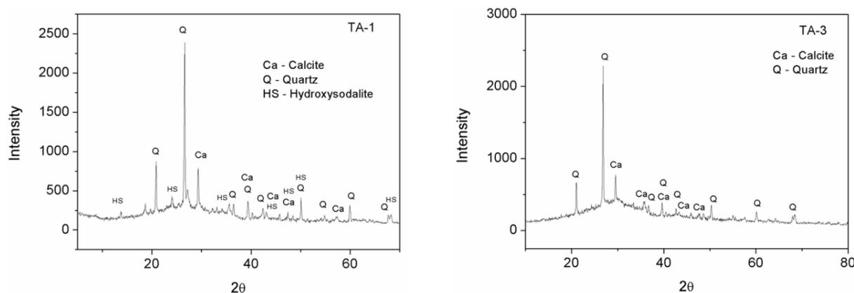
Figure 4. XRD patterns of the synthesis products obtained by hydrothermal treatment of sugarcane straw ash: TA-1 and TA-3
