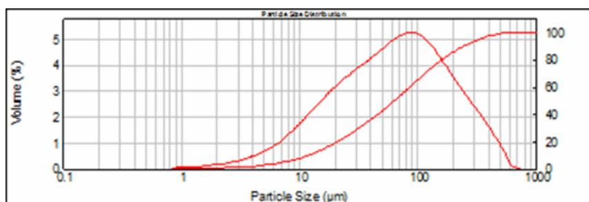
Figure 3. Particle size distribution of the sugarcane straw ash
