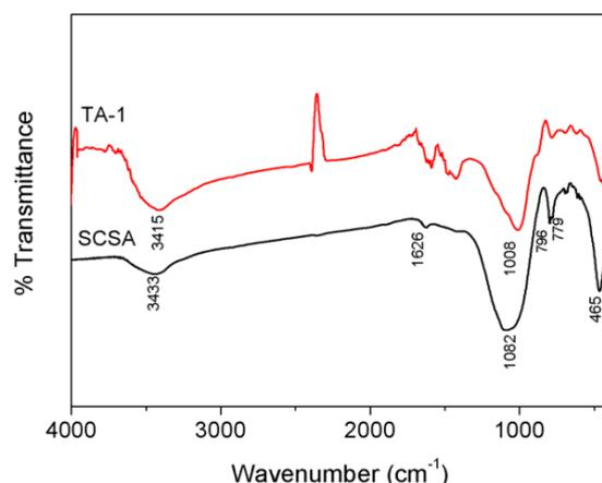
Figure 5. FTIR spectra of untreated (SCSA) and treated sugarcane straw ash (TA-1)
