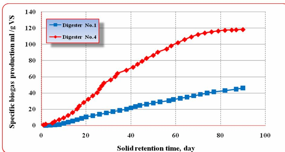
Figure 7. Specific and cumulative biogas production profiles in digesters No. 1 and 4
