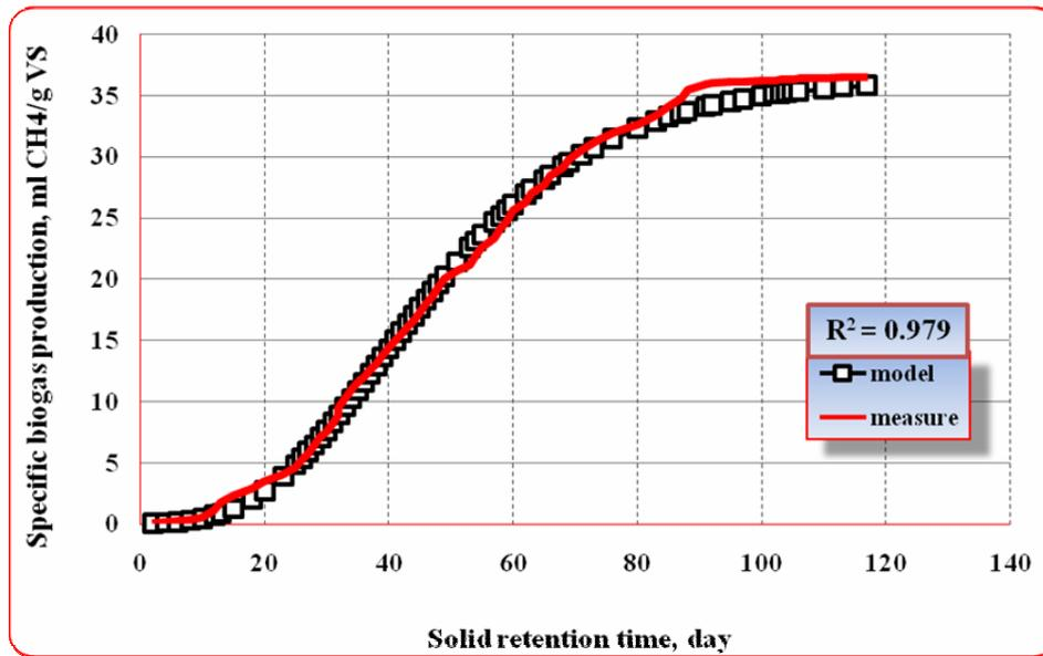
Figure 9. Measured and predicted results for biogas production from pretreated DPW
