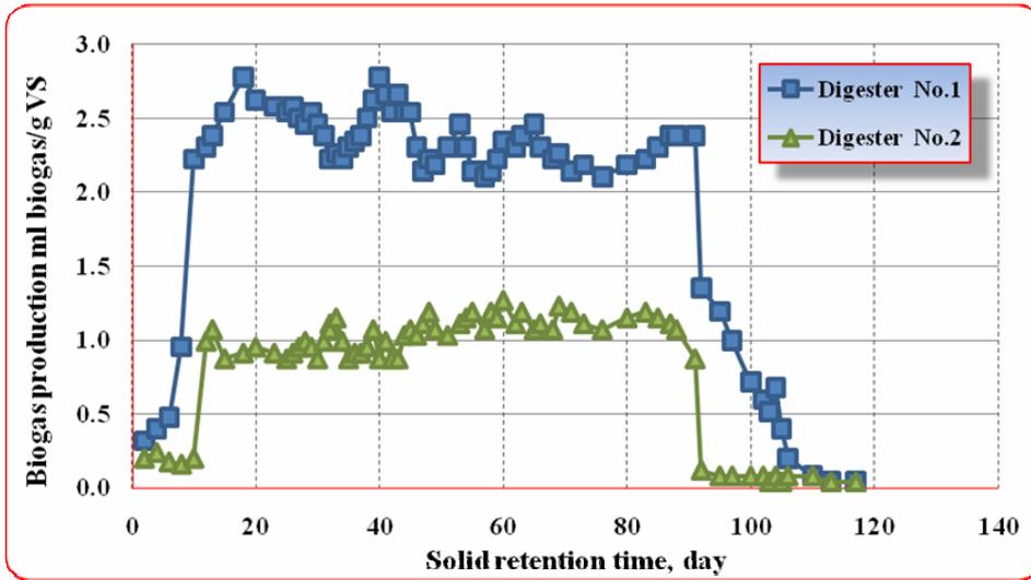
Figure 1. Biogas production profile for digesters No.1 and 2
