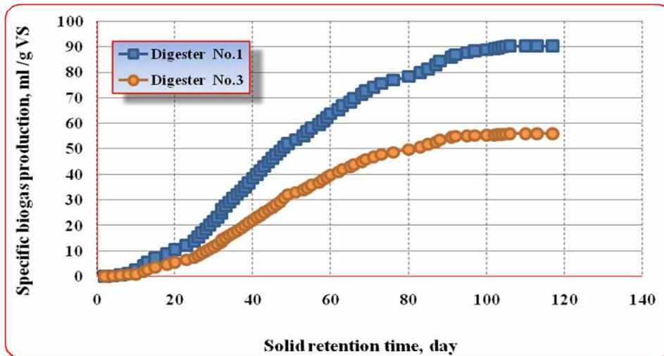
Figure 6. Specific and cumulative  $\text{CH}_4$  production profiles for digesters No. 1 and 3
