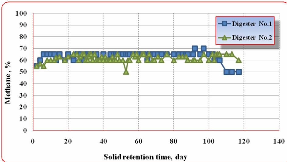
Figure 2. Percentages of CH<sub>4</sub> production for digesters No.1 and 2
