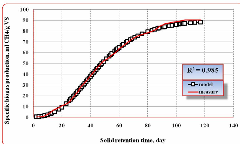
Figure 8. Measured and predicted results for biogas production from pretreated inoculated DPW
