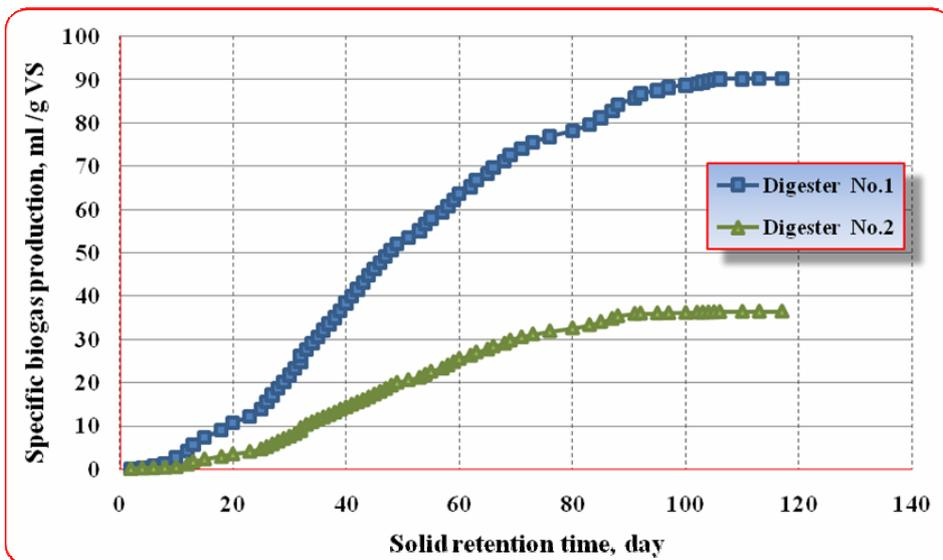
Figure 3. Specific cumulative biogas production profiles for digesters No. 1 and 2
