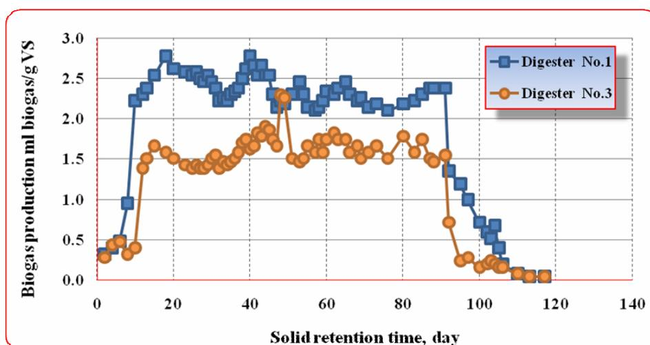
Figure 4. Biogas production profile for digesters No.1 and 3
