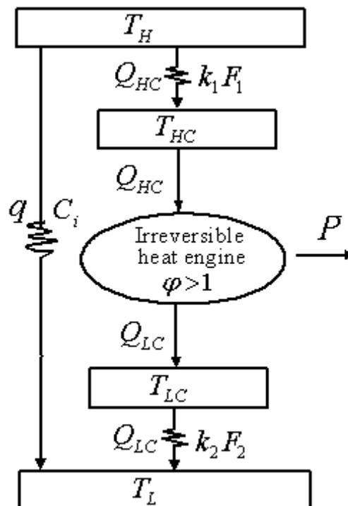
Figure 1. The generalized irreversible Carnot heat engine cycle model
