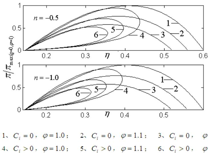
Figure 2. The influences of heat leak, internal irreversibility and heat transfer law on  $\pi - \eta$  characteristic for  $n < 0$
