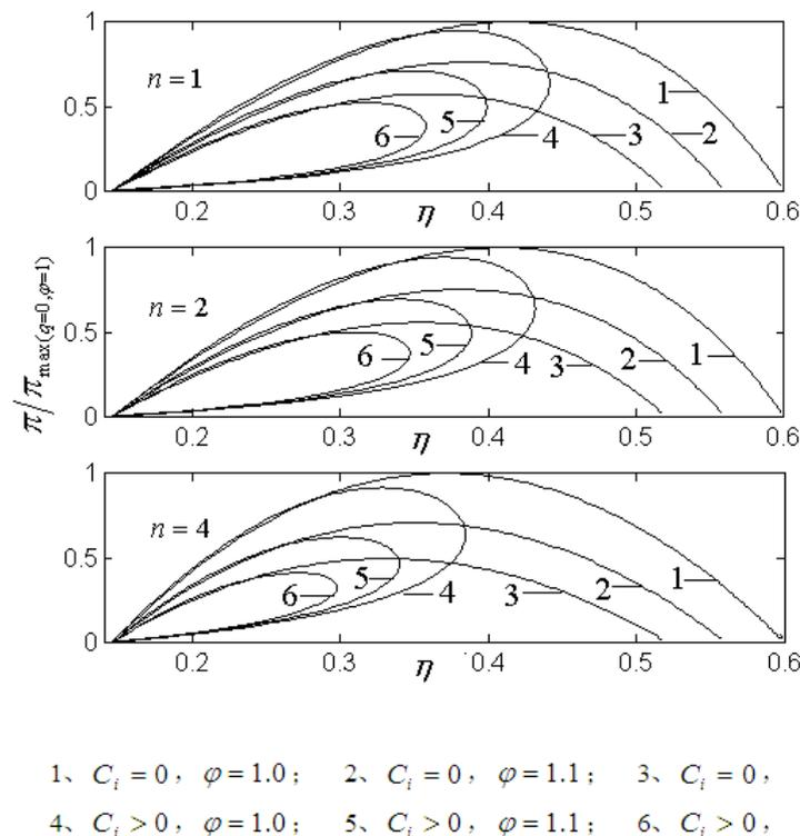
Figure 3. The influences of heat leak, internal irreversibility and heat transfer law on  $\pi - \eta$  characteristic for  $n > 0$
