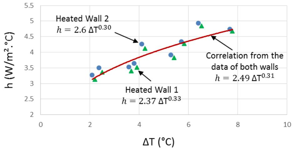
Figure 2. Correlation equations for heated walls (hot vertical walls)
