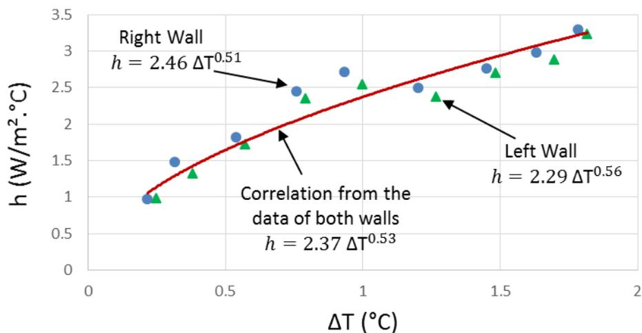
Figure 3. Correlation equations for right and left wall (cold vertical walls)
