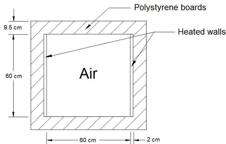
Figure 1. Schematic diagram of the enclosure
