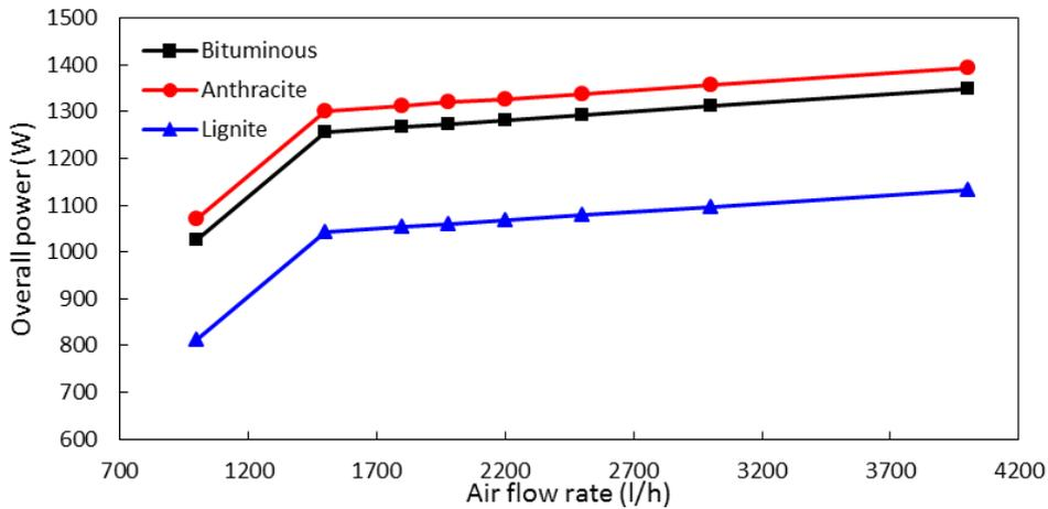
Figure 4. Overall energy output with increasing air flow rate using Co<sub>3</sub>O<sub>4</sub> as OC for 256 g/h of coal feeding rate
