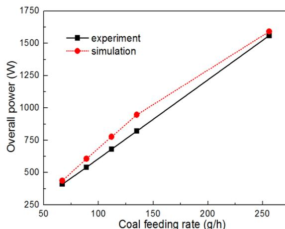
Figure 2. Comparison of overall power output between the simulation and the experiment
