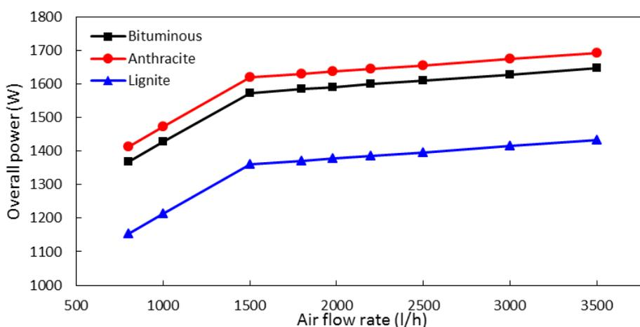
Figure 3. Overall energy output with increasing air flow rate using CuO as OC for 256 g/h of coal feeding rate
