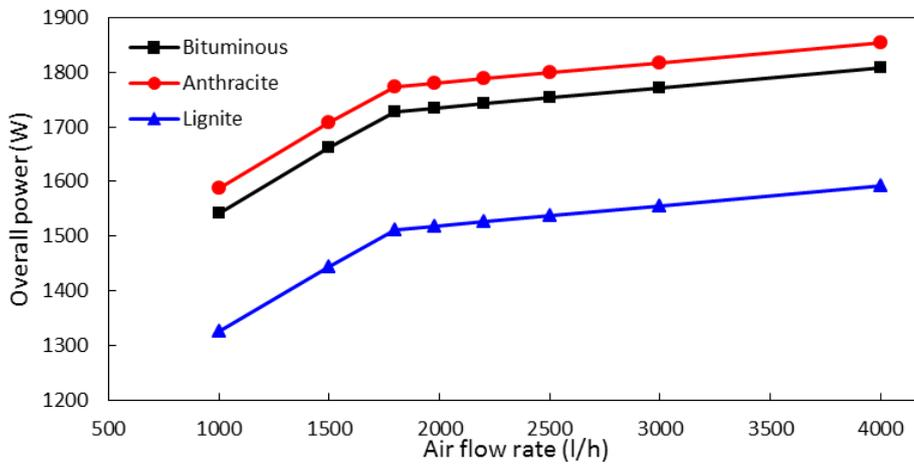
Figure 5. Overall energy output with increasing air flow rate using Mn<sub>2</sub>O<sub>3</sub> as OC for 256 g/h of coal feeding rate
