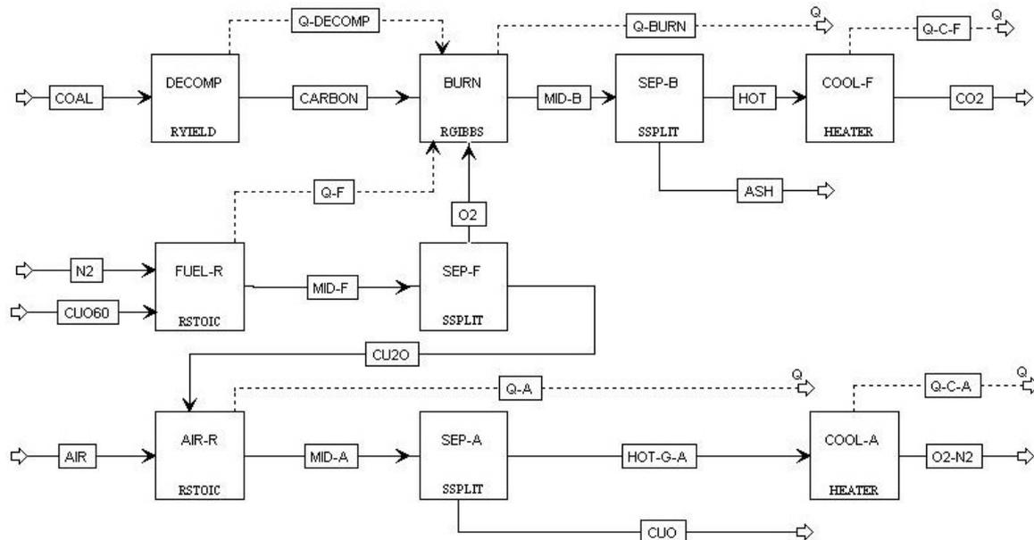
Figure 1. The flow sheet model of CLOU process in ASPEN Plus
