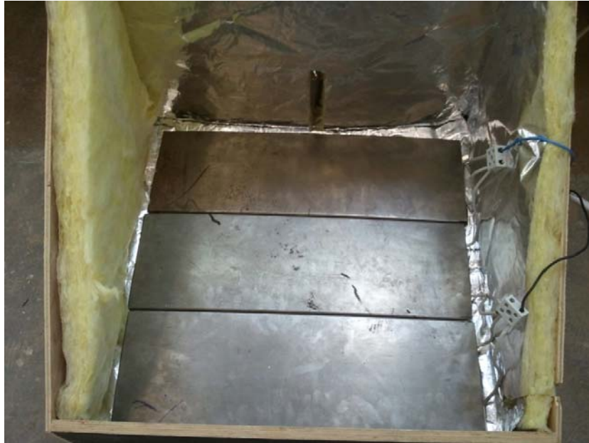
Figure 2. Three separate heaters connected in series at the base of the still
