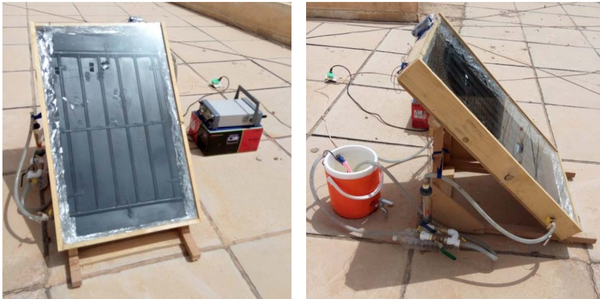
Figure 2. Experimental setup of flat plate solar collector
