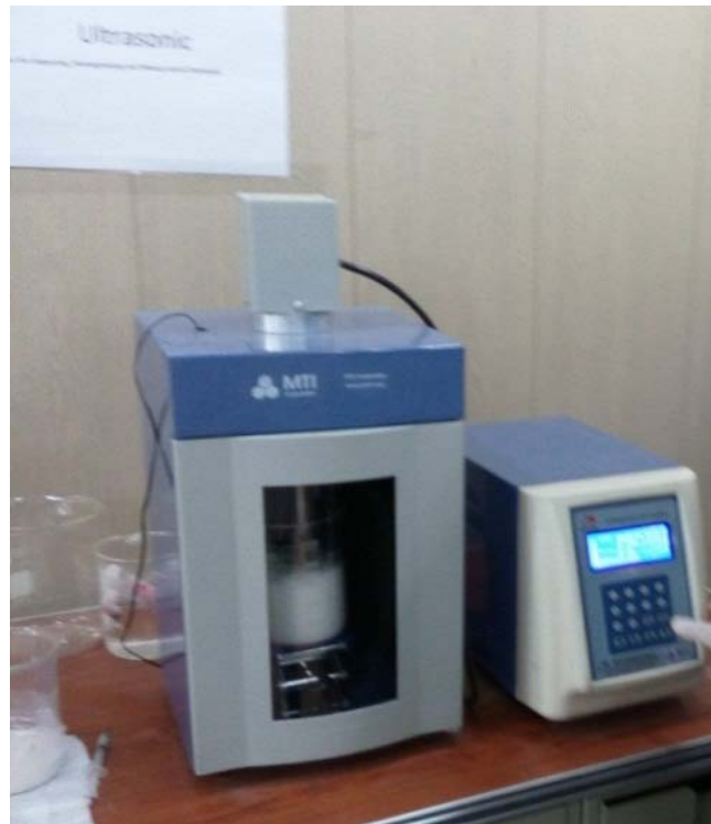
Figure 8. Ultrasonic cleaner apparatus for sonication process of \text{Al}_2\text{O}_3 -water nanofluids
