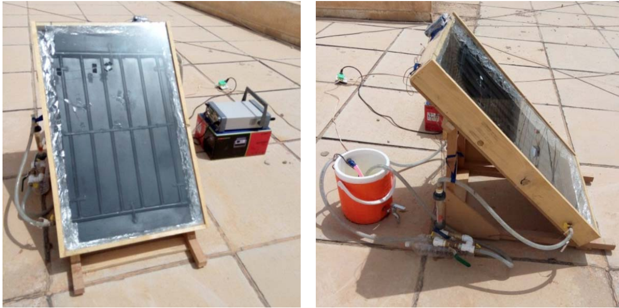
Figure 2. Experimental setup of flat plate solar collector
