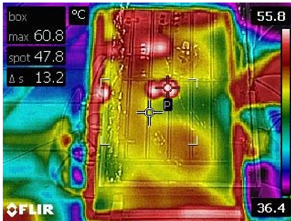
Figure 11. An infrared image of the solar collector with \text{Al}_2\text{O}_3 nanofluid as working fluid
