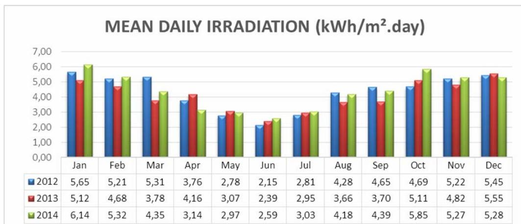
Figure 3. Mean daily irradiation on horizontal surface provided by INMET A807 station (kWh/m<sup>2</sup>.day). Source: The authors.
