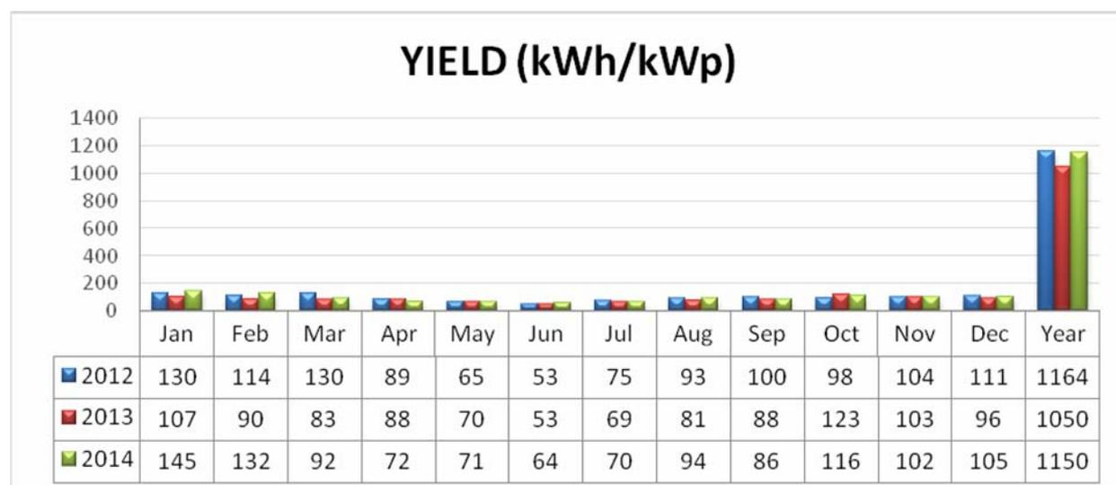
Figure 11. Monthly and annual Yield of the GO's grid-connect PV system of the UTFPR. Source: The authors.
