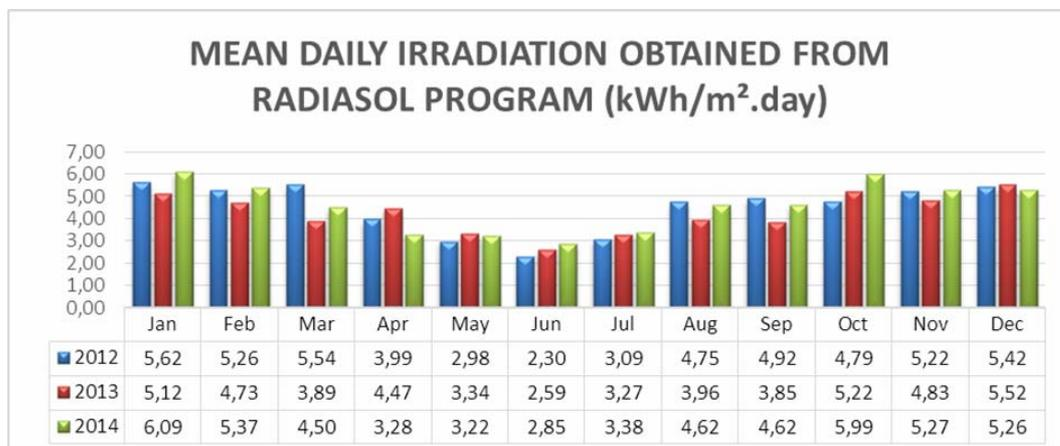
Figure 6. Mean daily irradiation on GO's PV panel surface obtained from RADIASOL software (kWh/m<sup>2</sup>.day). Source: The authors.
