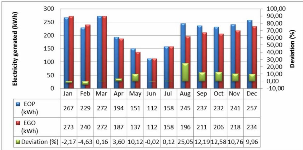
Figure 7. Comparison between the optimum grid-connected PV system and the real GO's grid-connected PV in 2012. Source: The authors.
