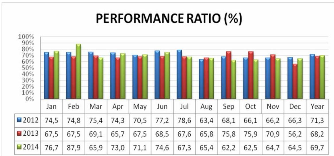
Figure 13. Monthly and annual Performance Ratio of the GO’s grid-connect PV system of the UTFPR. Source: The authors.
