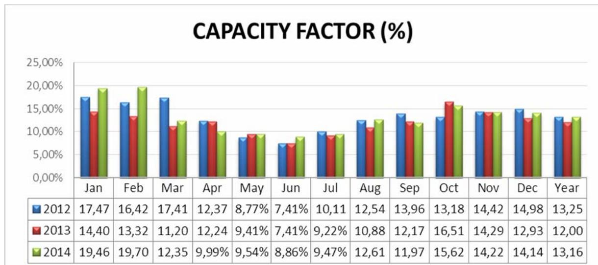
Figure 14. Monthly and annual Capacity Factor of the GO's grid-connect PV system of the UTFPR.
