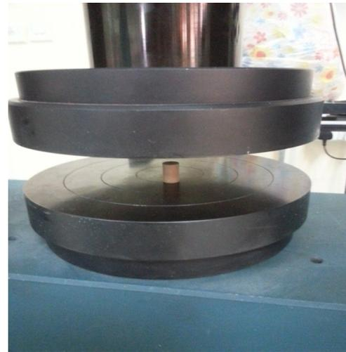
Figure 3. Shape memory effect test.
