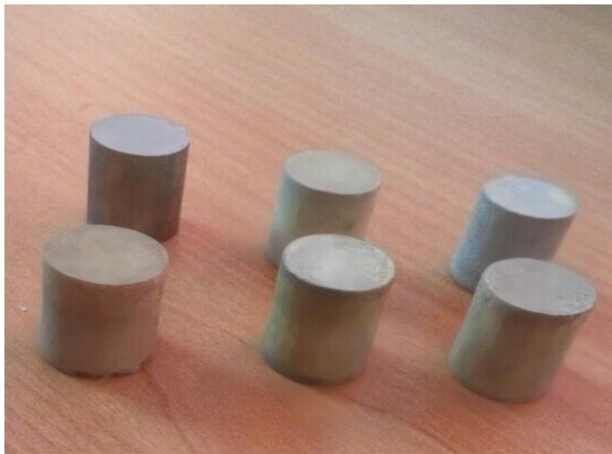
Figure 2. Samples after sintering.
