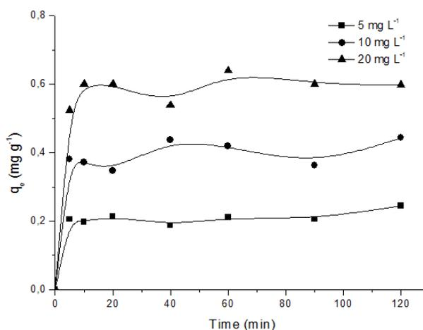
Figure 9. Effect of agitation time in the RB adsorption capacity by SMZBA ( $T = 25 \pm 2^\circ\text{C}$ ).
