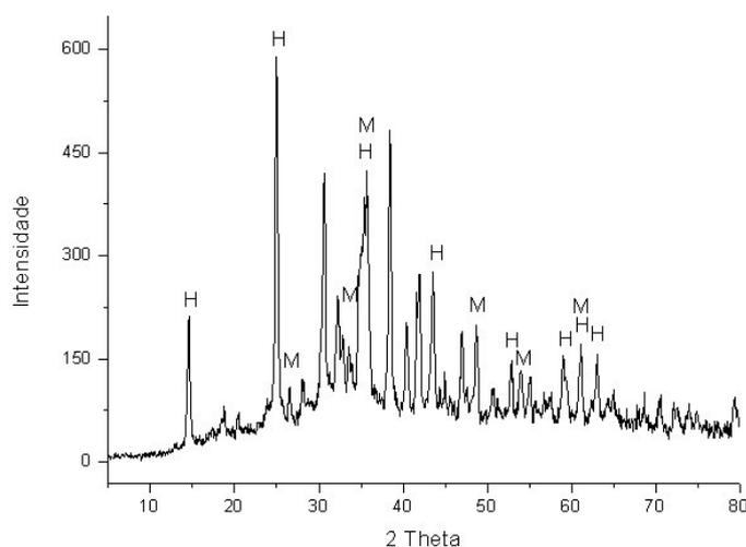
Figure 3. X-ray diffraction patterns of the zeolite from remaining solution (M = Mullite; H = Hydroxysodalite).
