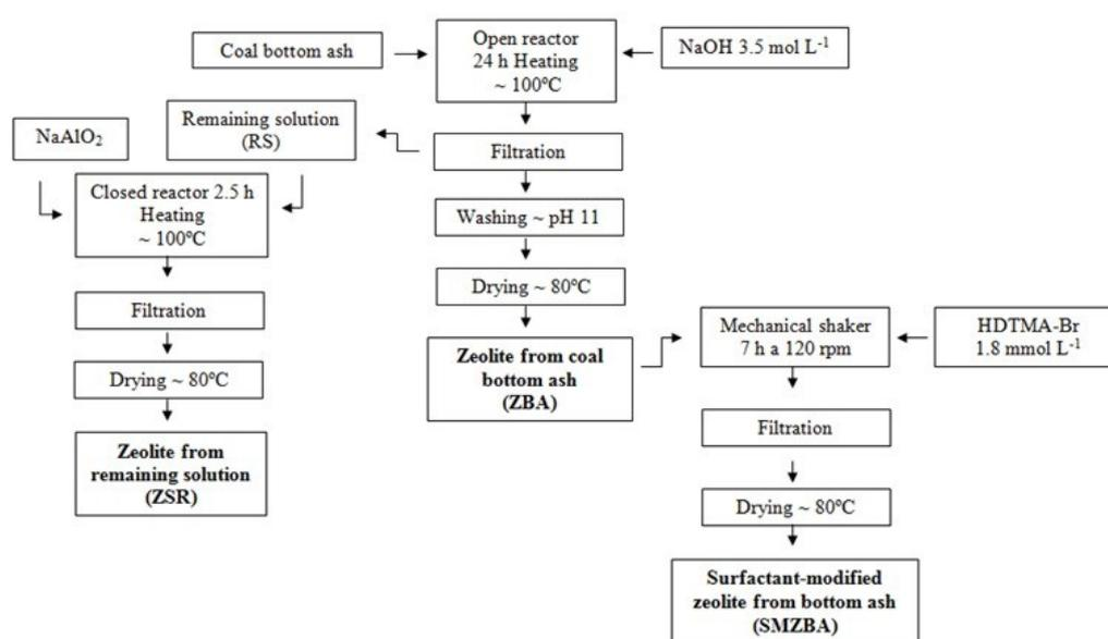
Figure 2. Synthesis scheme of zeolites.
