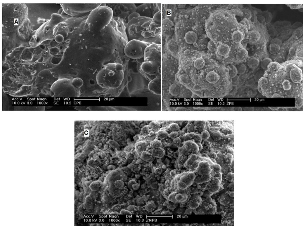
Figure 5. SEM photographs of (a) CBA; (b) ZBA; (c) SMZBA. Magnification 1000x.
