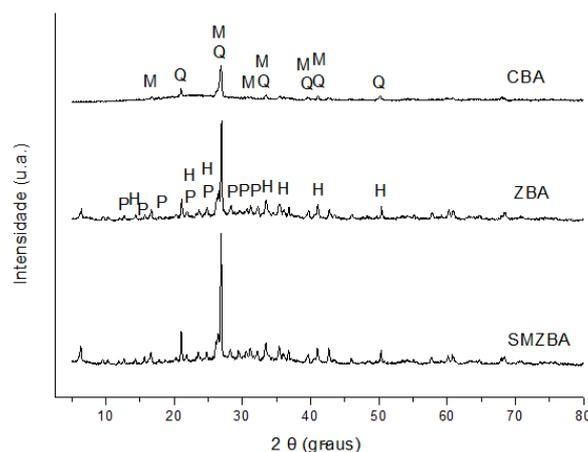
Figure 8. X-ray diffraction patterns of CBA, ZBA and SMZBA (M = Mulinite; Q = Quartz; H = Hydroxysodalite; P= NaP1).
