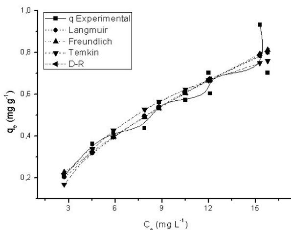
Figure 10. Adsorption isotherm of RB onto SMZBA (T =25 ± 2°C).
