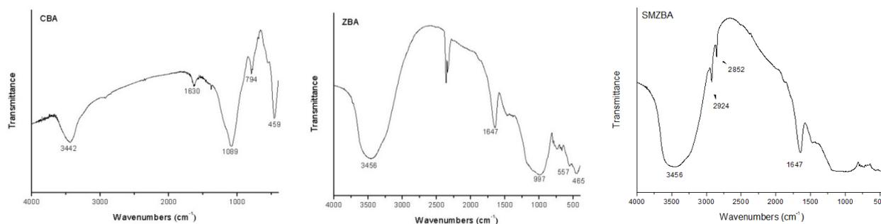
Figure 7. FTIR Spectra of raw coal bottom ash (CBA), unmodified zeolite (ZBA) and surfactant-modified zeolite (SMZBA).
