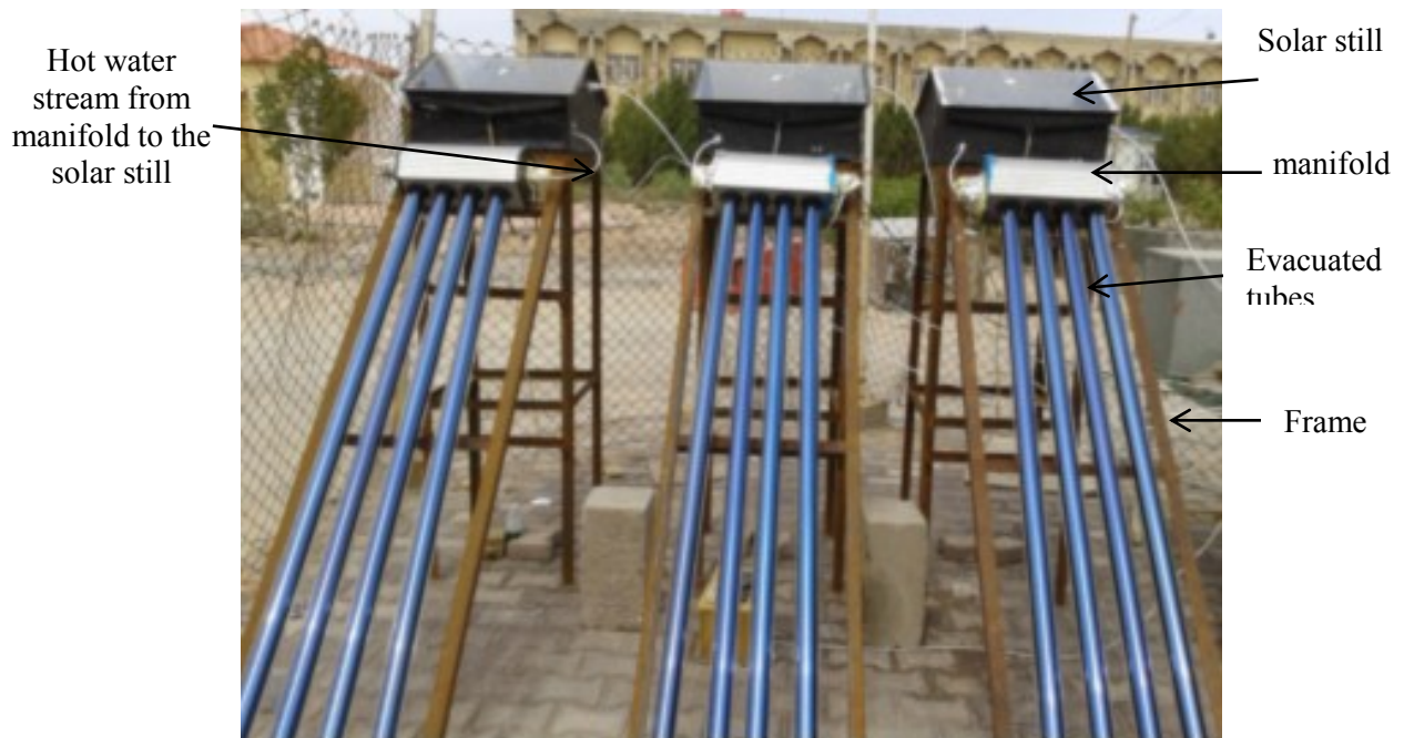
Figure 1. System of the work of solar still.
