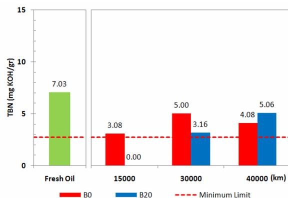
Figure 5. TBN for the vehicle B.
