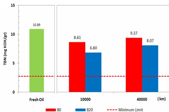
Figure 4. TBN for the vehicle A.
