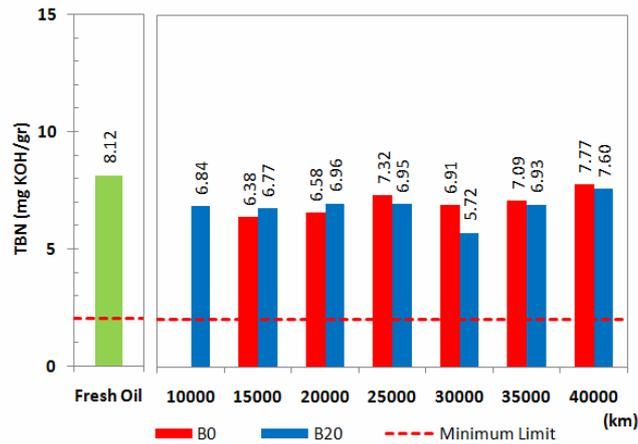
Figure 6. TBN for the vehicle C.
