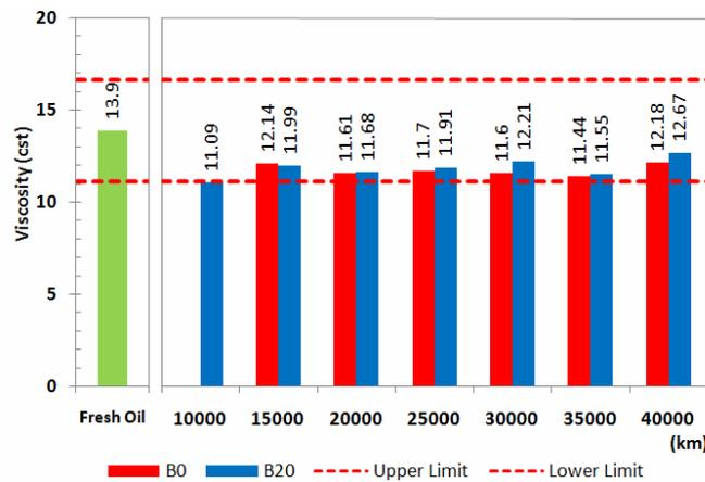
Figure 3. Viscosity of the vehicle C.
