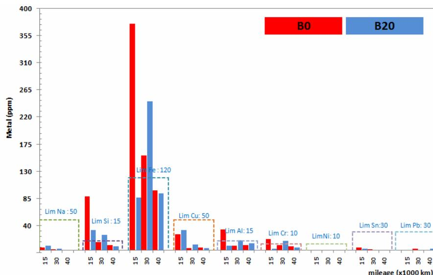
Figure 8. Wear metals analysis of the vehicle B.
