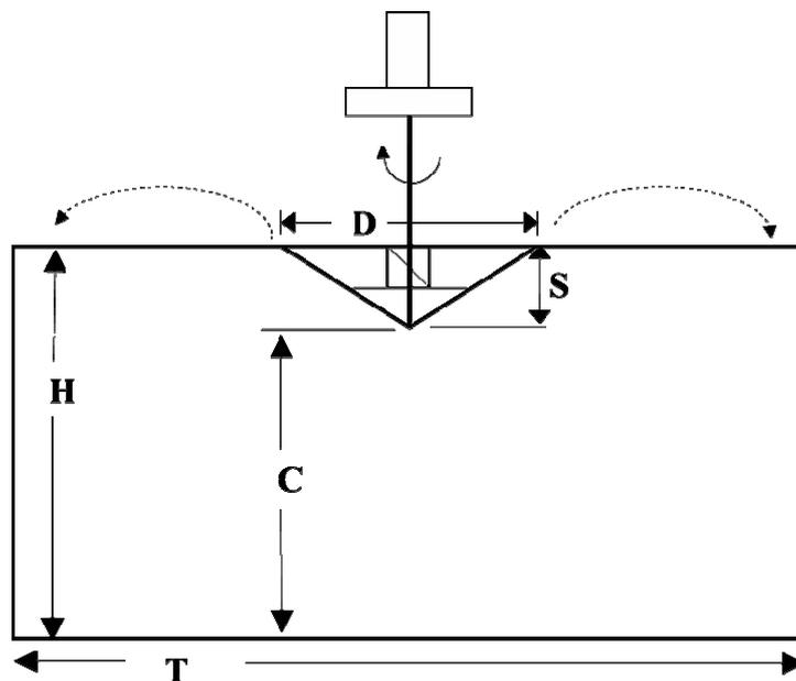
Figure 1. The schematic diagram of the surface aerator system.
