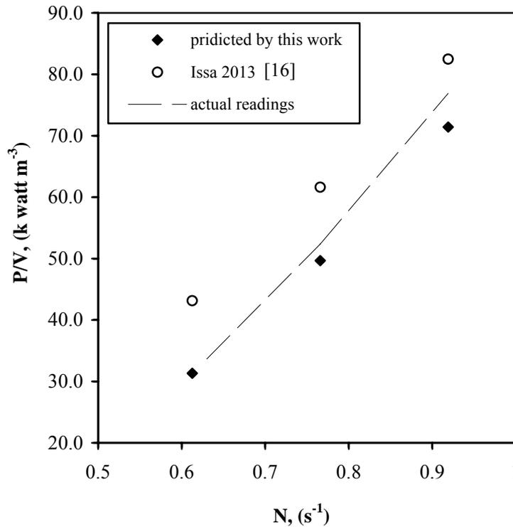
Figure 2. Comparison of predicted volumetric power consumption P/V and the actual P/V.
