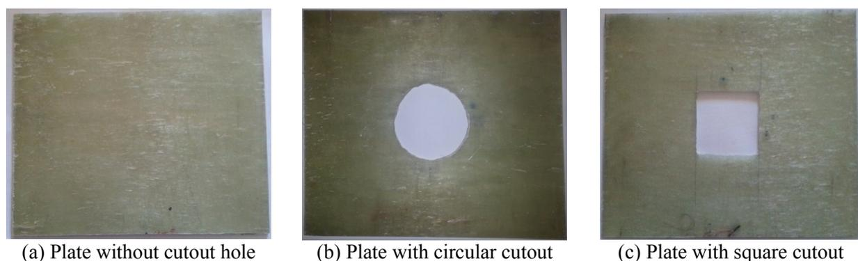
Figure 1. Plate samples of experimental work with and without cutouts.
