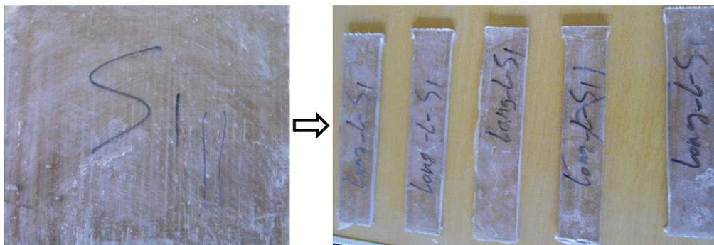
Figure 3. Tensile test samples used in experimental work.
