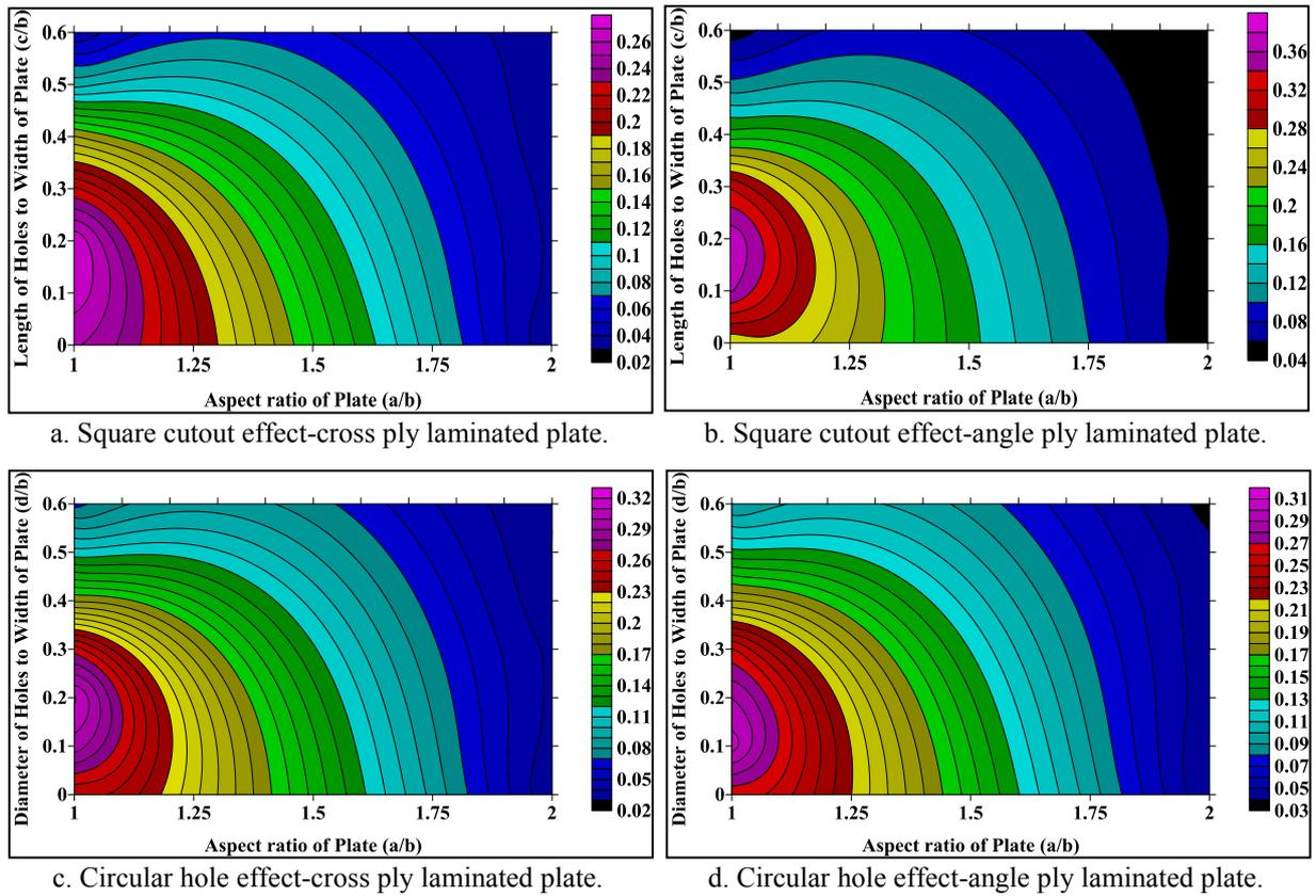
Figure 12. Maximum deflection  $W$  (mm) of clamped supported cross-ply and angle ply plate with various cut outs.
