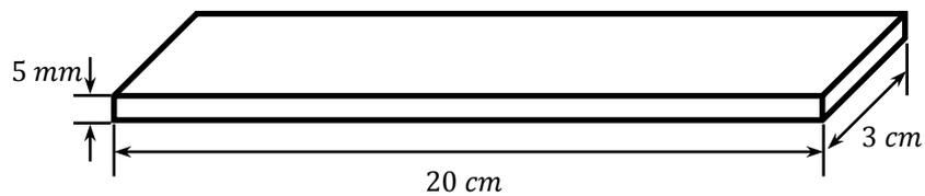
Figure 4. Dimensions of tensile test samples.
