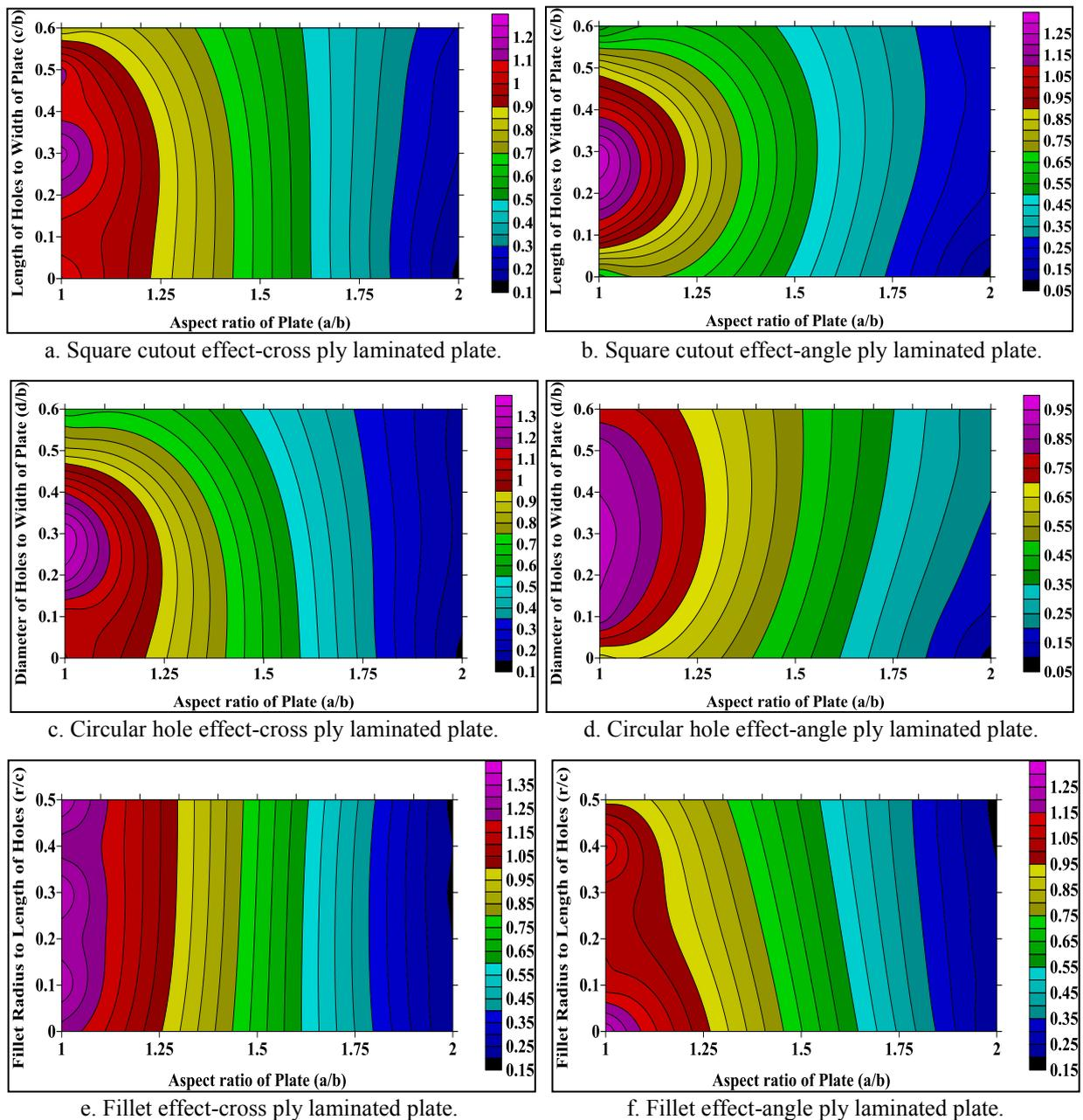
Figure 11. Contours of deflection  $W$  (mm) of simply supported cross-ply and angle ply plate with different types cut outs.
