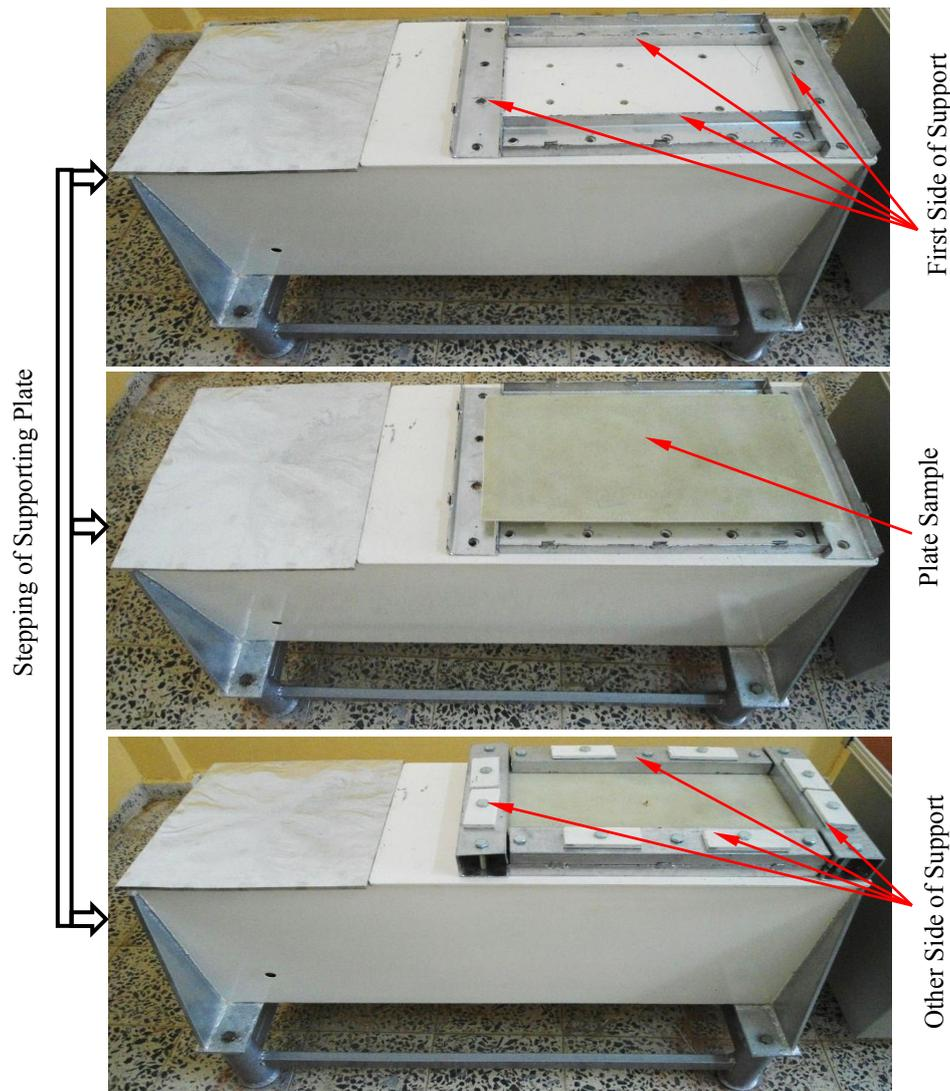
Figure 5. Test rig of the supported plate.
