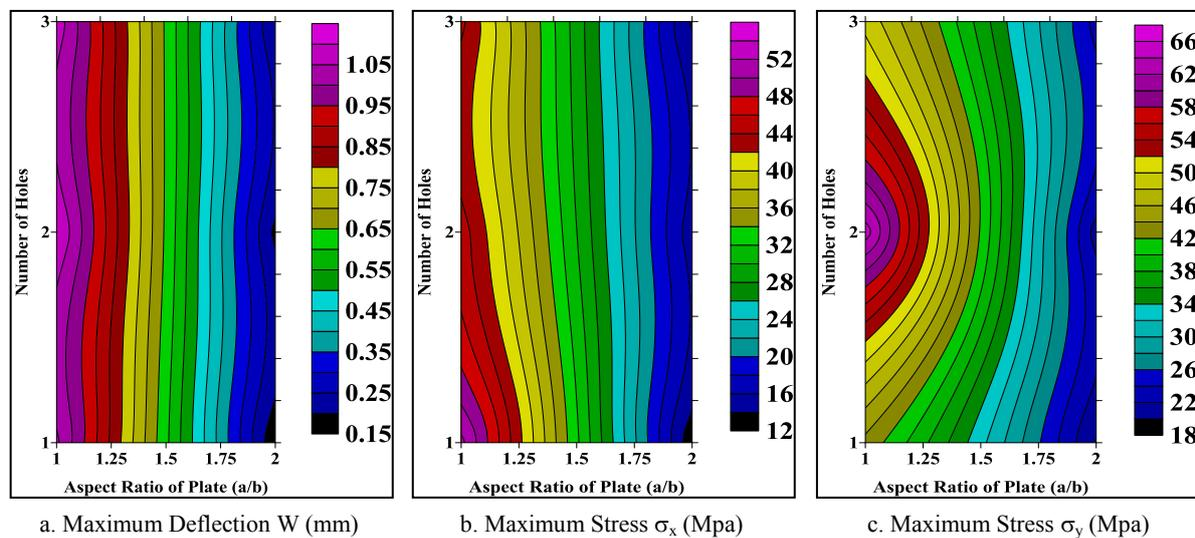
Figure 17. Contours of maximum deflection and stresses in x and y-directions of simply supported cross-ply laminated plate with various number of circular holes, size  $d/b=0.1$  and  $N=4$ .
