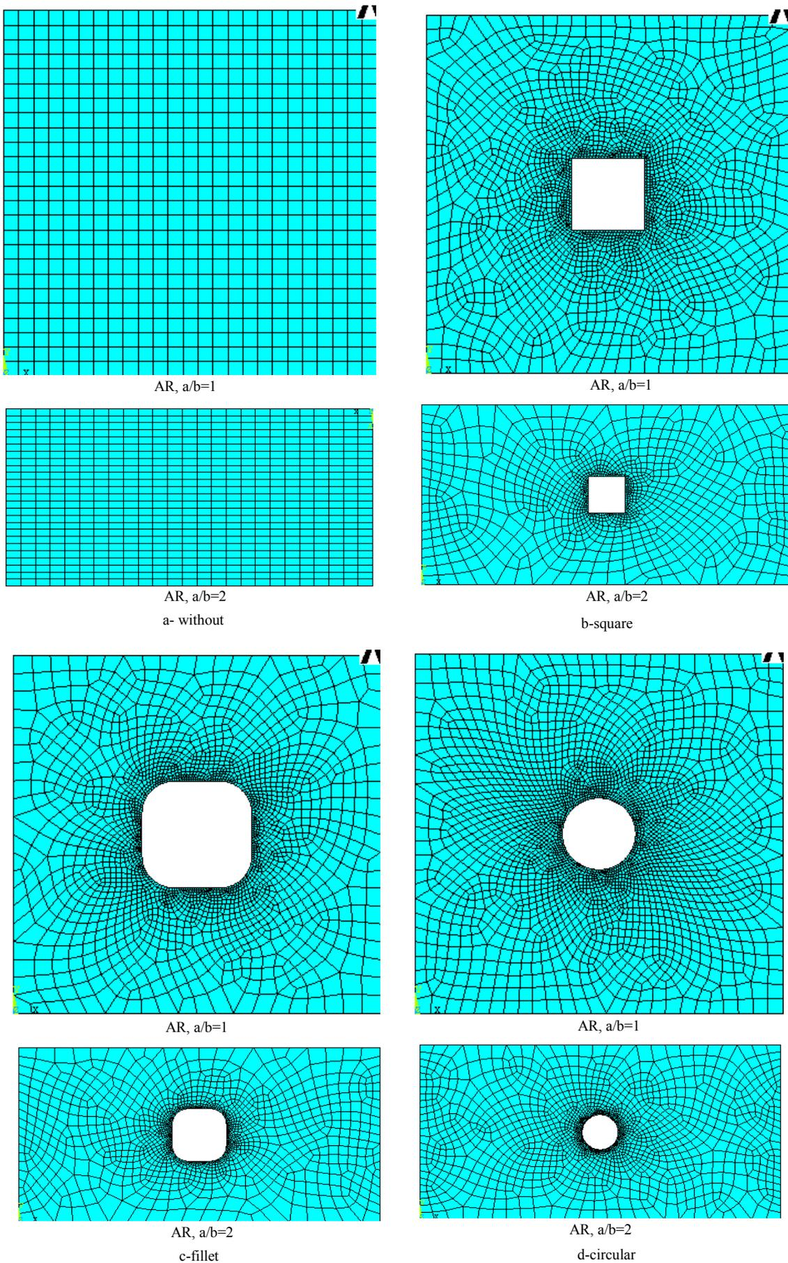
Figure 8. Finite element meshes of laminated plate with cut outs (AR =1,2).
