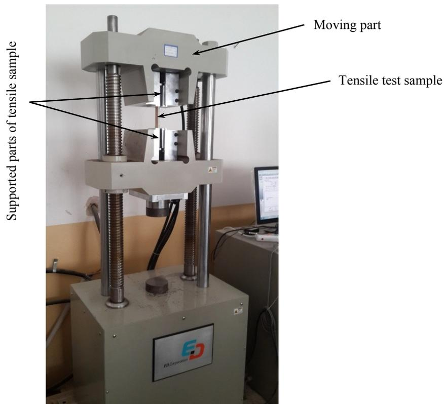
Figure 2. Tensile test machine.
