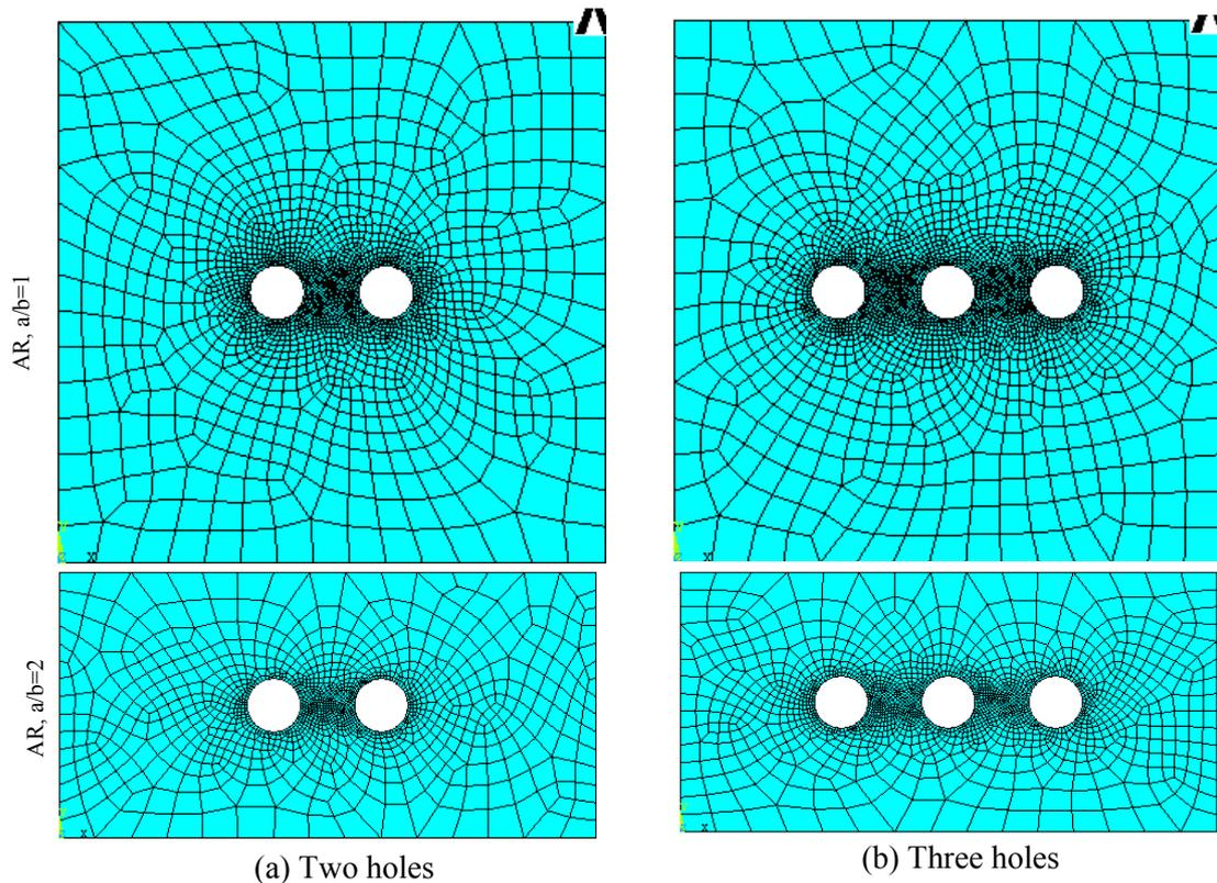
Figure 9. Finite element meshes of multi cut outs in laminated plate (AR=1,2).
