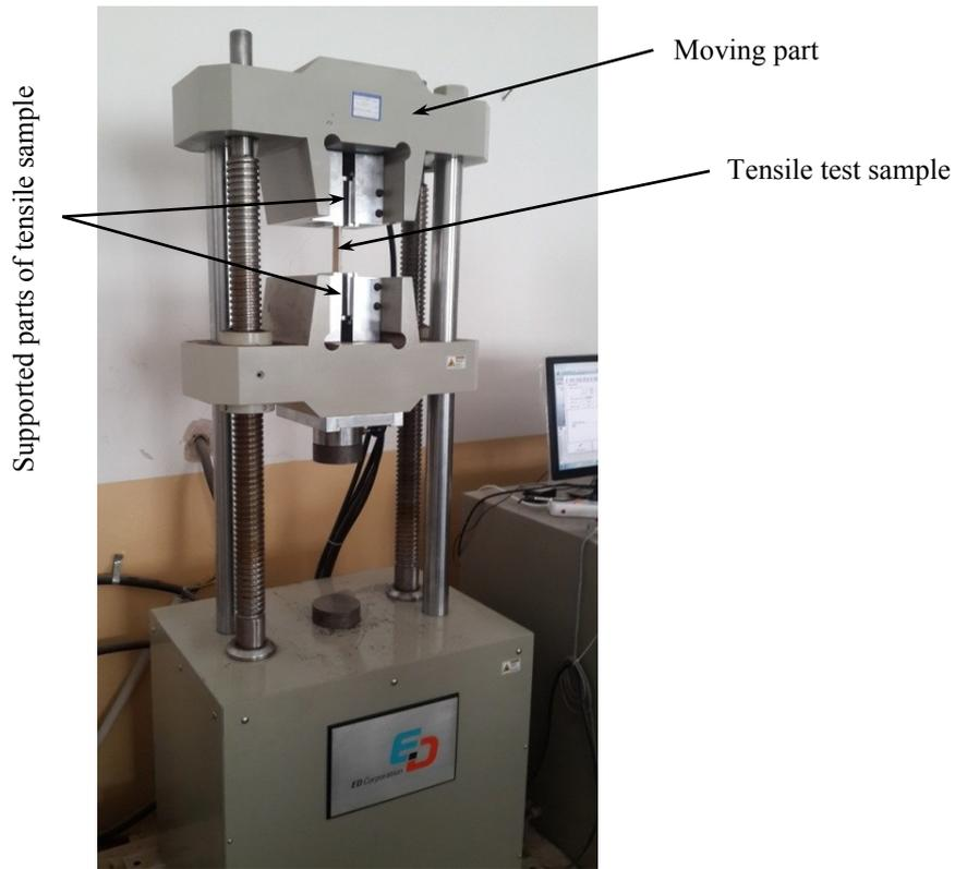
Figure 2. Tensile test machine.
