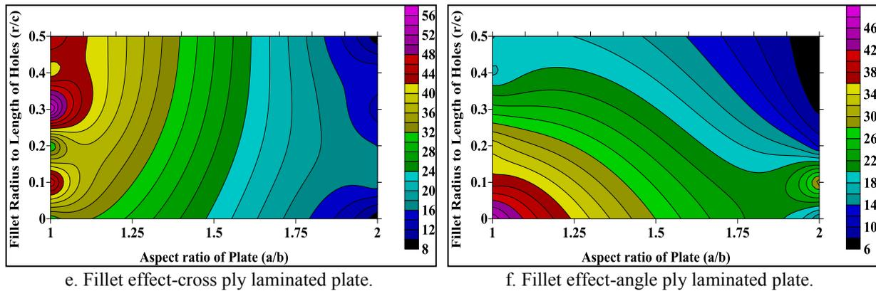
Figure 13. Maximum Stress  $\sigma_x$  (Mpa) of simply supported cross-ply and angle ply plate with different cut outs effects.
