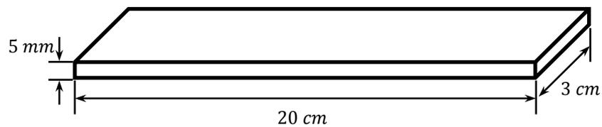
Figure 4. Dimensions of tensile test samples.
