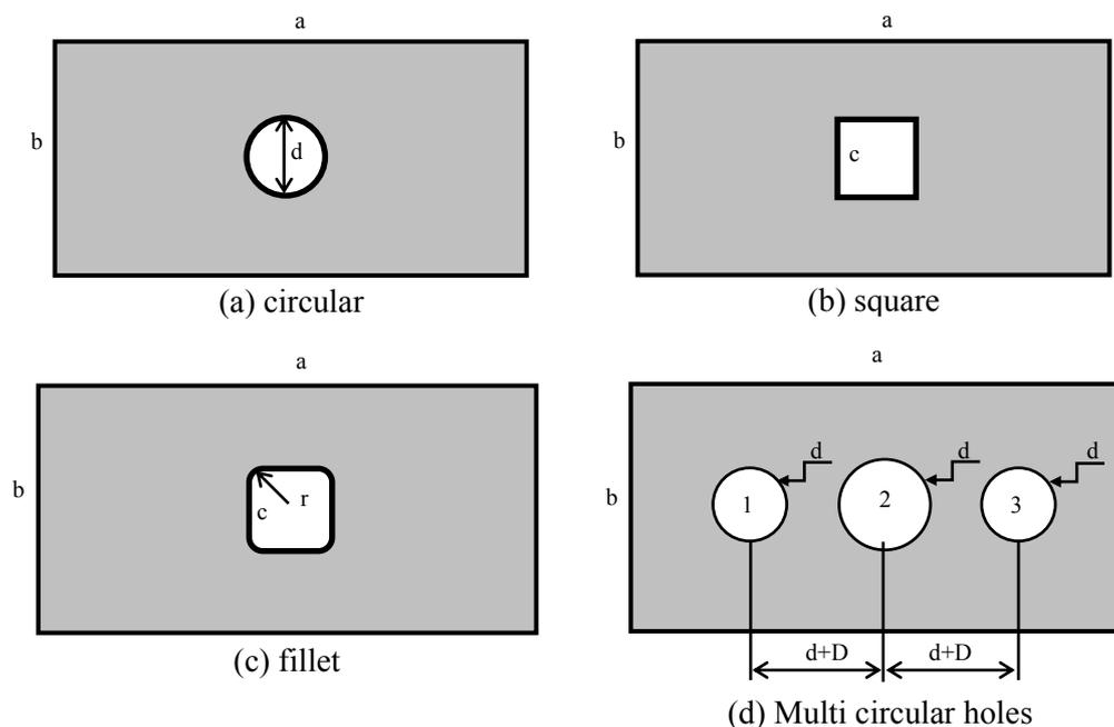
Figure 10 . Dimensions and shapes of cut outs in composite laminated plate.
