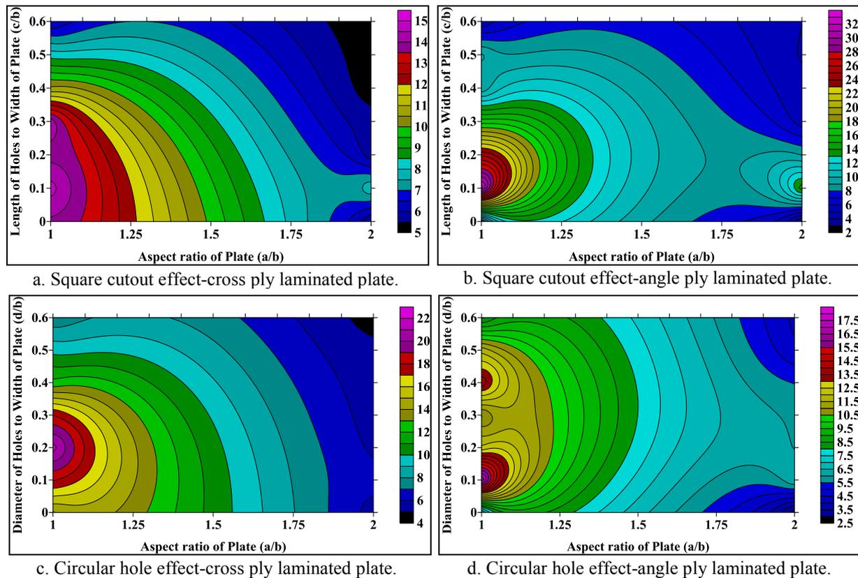
Figure 16. Contours of Stress  $\sigma_y$  (Mpa) of clamped supported cross-ply and angle ply plate with different cut outs.
