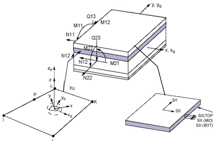
Figure 7. Shell 281 stress output.
