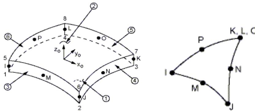
Figure 6. Shell 281 geometry.
