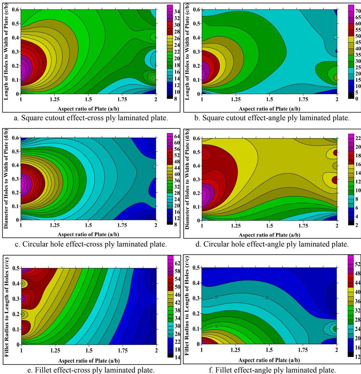
Figure 15. Contours of Stress  $\sigma_y$  (Mpa) of simply supported cross-ply and angle ply plate with different cut outs.
