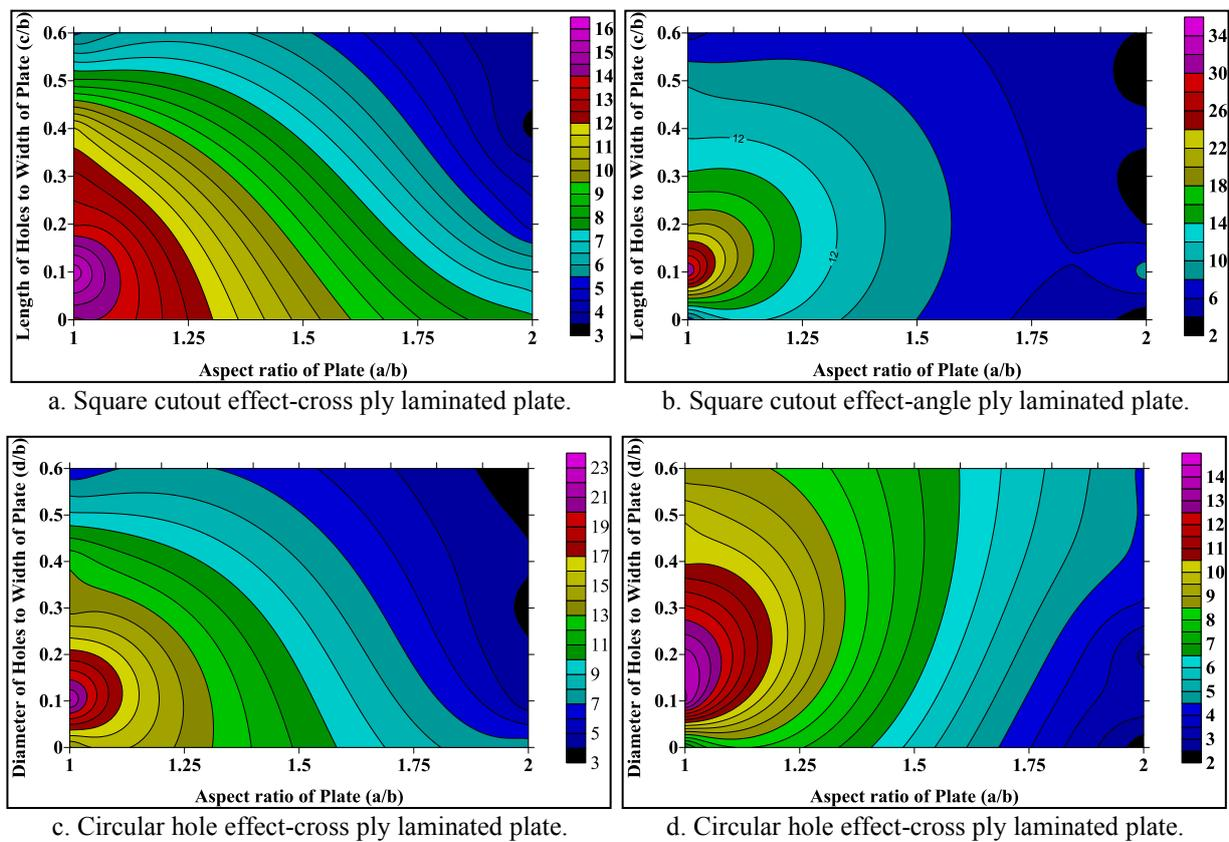
Figure 14. Contours of Stress  $\sigma_x$  (Mpa) of clamped supported cross-ply and angle ply plate with different cut outs.
