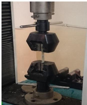
Figure 2. Tensile test machine
