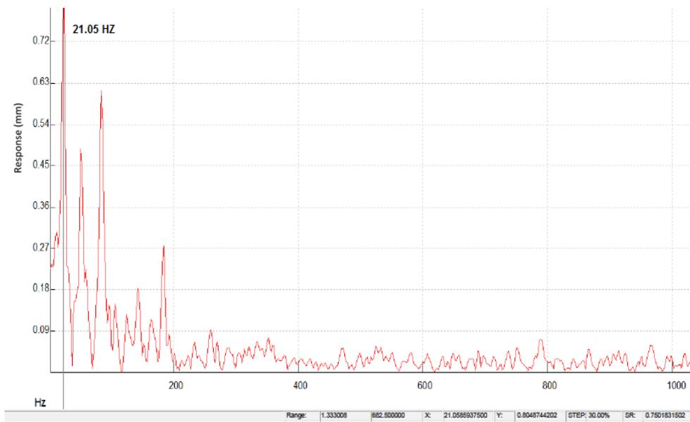
Figure 5. Experimental response (displacement) spectrum of the cantilever skew angle 0°.
