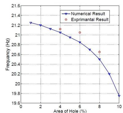
Figure 8. Effect of hole area percentage on the natural frequency for a cantilever skew plate.
