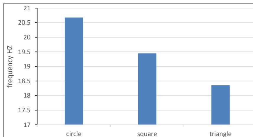
Figure 9. Effect of hole shape on the fundamental frequency for a cantilever skew plate.
