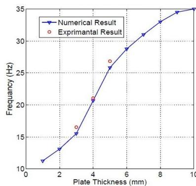
Figure 7. Effect of the plate thickness on the fundamental natural frequency for a cantilever skew plate.
