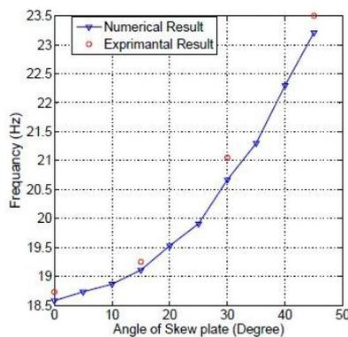
Figure 6. Effect of the skew angle on the natural frequency for a cantilever skew plate.
