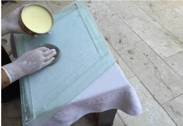
Figure 3. The mold of the composite skew plate.
