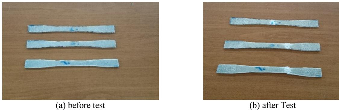
Figure 1. Tensile test specimen.
