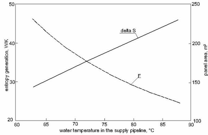
Figure 9. Heating panel area and entropy production v.s. the water temperature (thermal power of 80000 W).
