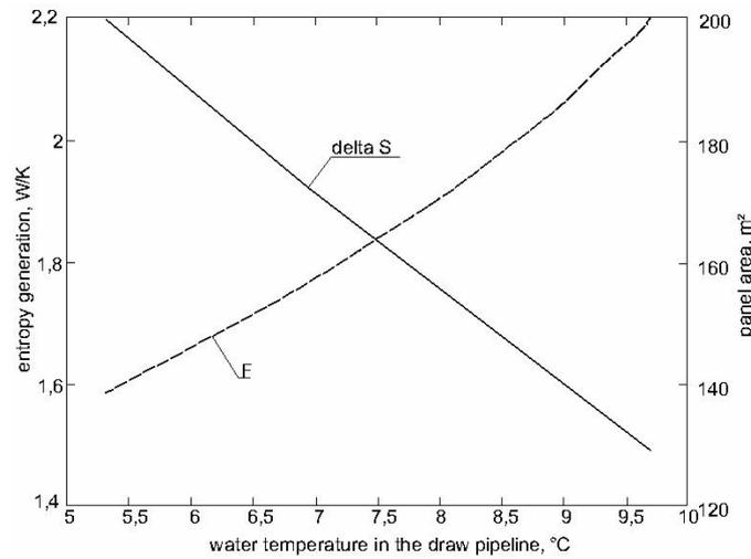
Figure 10. Cooling system area and the entropy production in the function of water temperature (cooling power of 15000 watts).
