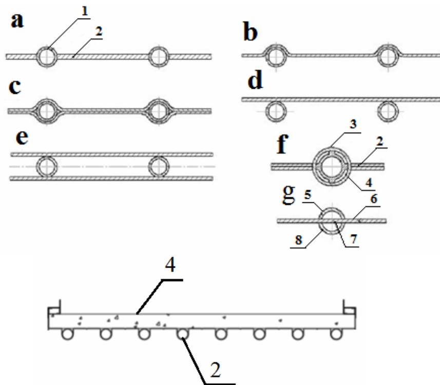
Figure 1. The structural shapes of the radiating planar panel: 1 is a pipe, 2 is a rib, 3 is an inner pipe, 4 is an outer pipe (protective casing), 5 is the upper half-pipe, 6 is an emitting part of the rib, 7 is a convective part of the rib, 8 is a lower half-pipe.
