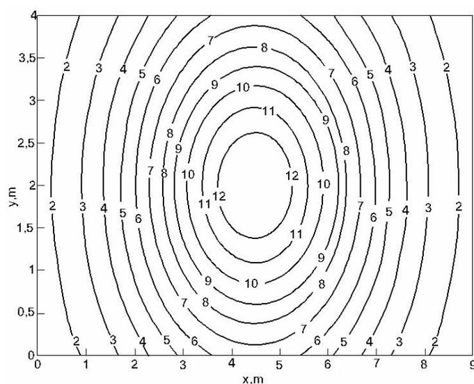
Figure 6. The intensity distribution of the radiation at a distance from the normal under the panel,  $\text{W/m}^2$ .
