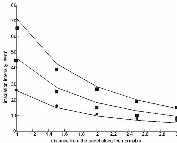
Figure 5. Comparison of the experiment (marker) and calculation at water  $t = 50, 70, 90^{\circ}\text{C}$  [15].
