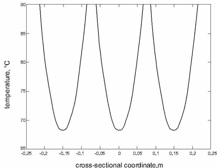
Figure 4. Temperature distribution across the panel at water temperature 90°C, panel width being 0.472m.
