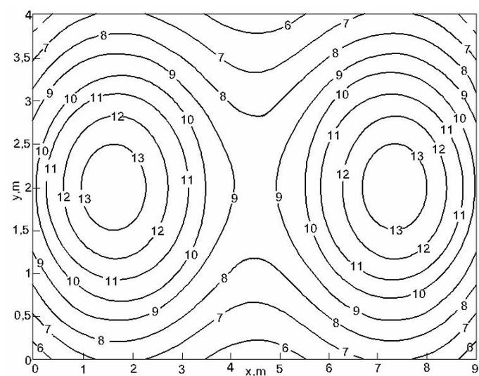
Figure 7. Distribution of irradiance from two panels,  $\text{W/m}^2$ .
