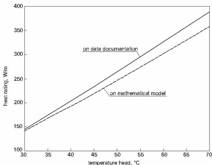
Figure 8. Comparison of thermal Waterstrip series panel (WP2-060) powers.
