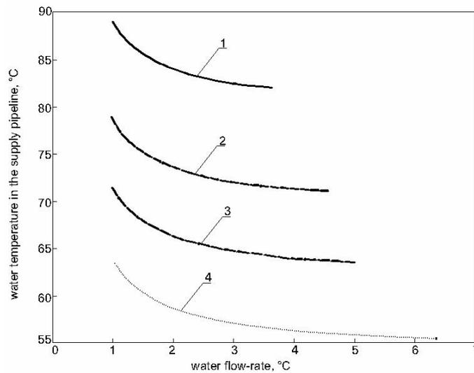
Figure 11. Water temperature in the function of the flow rate for heating systems with a different panel area (heating power 80000 W).
