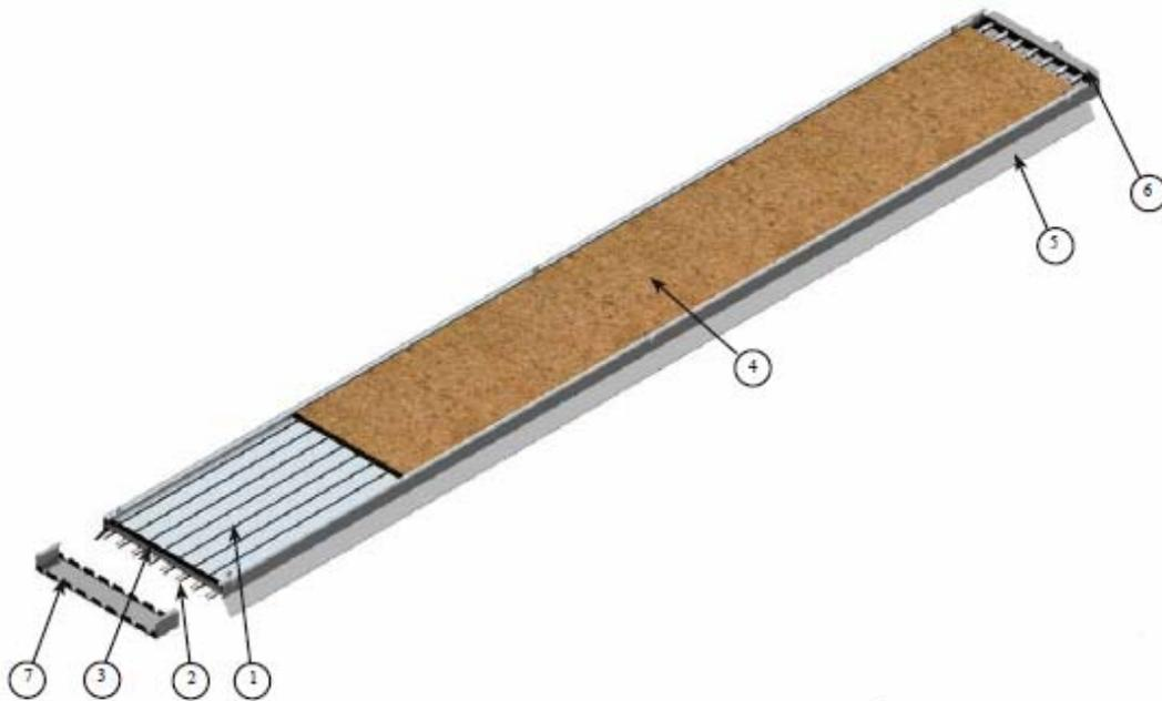
Figure 2. (1) Profiled panel made of coated steel; (2) Pipes of 22mm diameter; (3) Gain traverse; (4) Upper isolating layer; (5) Counter convectional lateral overhang; (6) Square section collector; (7) Waterstrip panel connection element.
