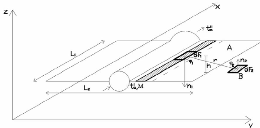
Figure 3. The module design and calculation-model element of the radiating surface.
