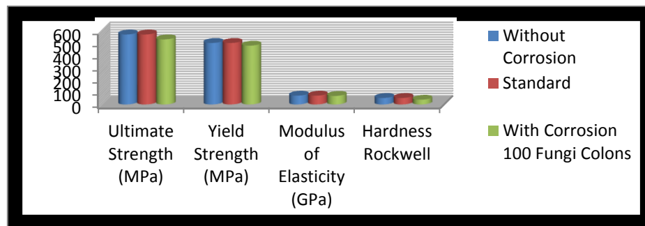
Figure 5. Effect of corrosion on mechanical properties.
