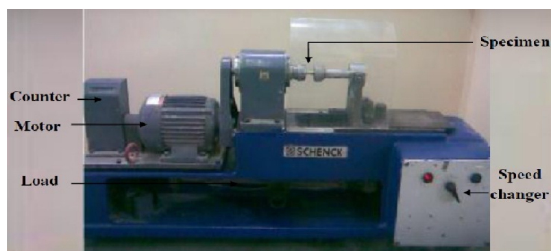
Figure 3. PUNN rotating bending testing machine [10].
