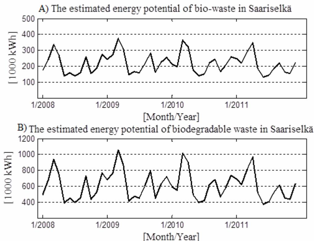
Figure 5. (A) The estimated energy potential of bio-waste, and (B) the estimated energy potential of biodegradable waste collected at Saariselkä.
