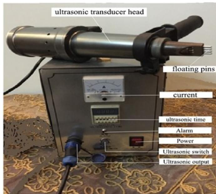
Figure 2. Ultrasonic peening device type HC-S-1.
