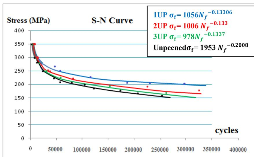
Figure 7. Four cases of fatigue test result with and without UP.
