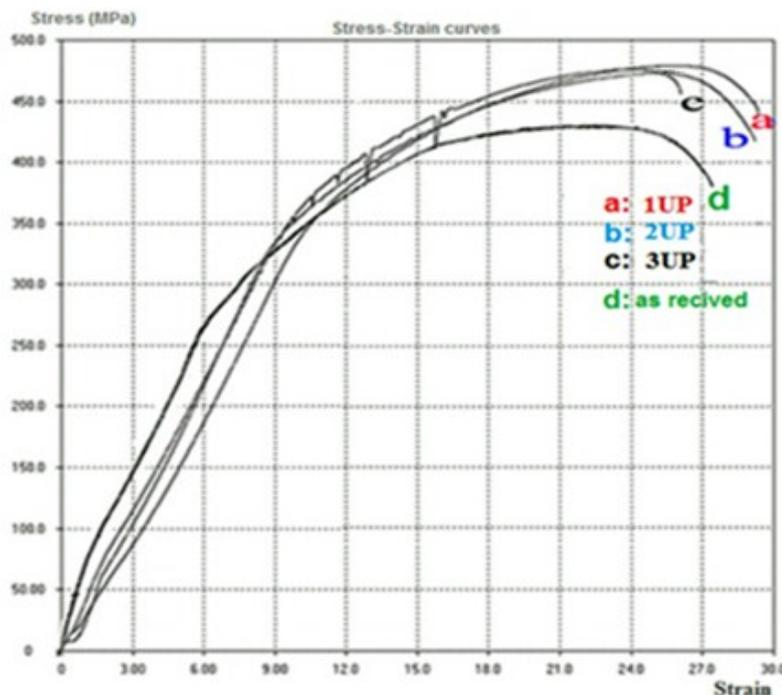
Figure 5. Three conditions of UP stress-strain curves compared with as received data.
