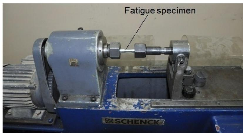
Figure 4. Fatigue testing machine type SCHENCK PUNN.
