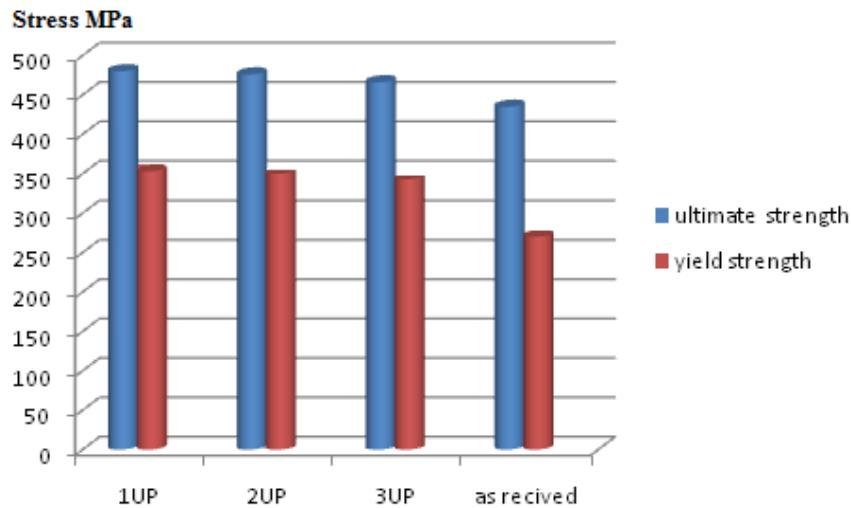
Figure 6. Comparison of four conditions tensile properties.
