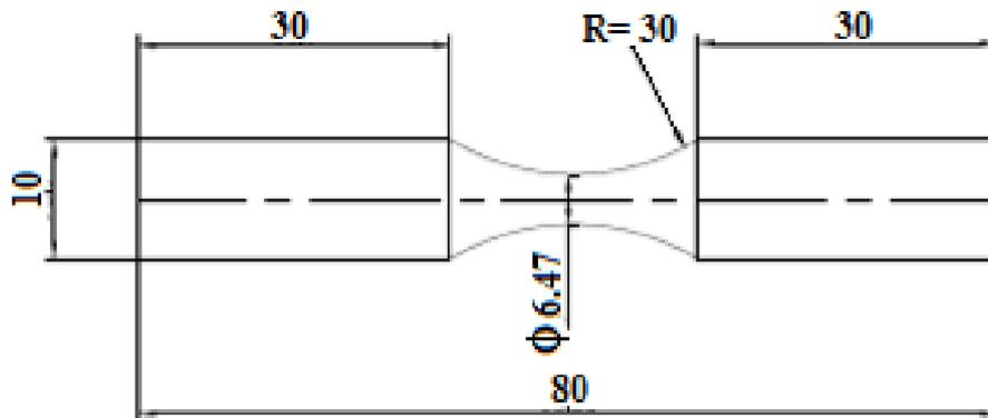
Figure 3. Geometry of fatigue specimen's dimensions in millimeter according to (DIN 50113) used standard specification.
