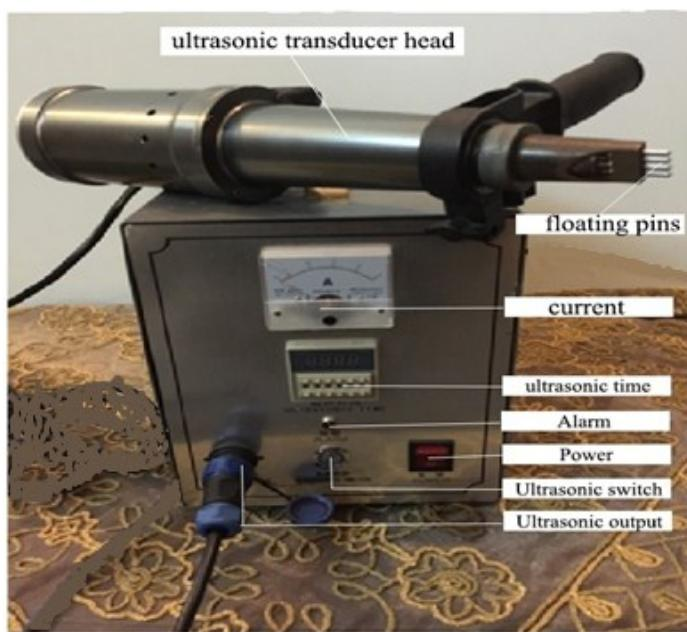
Figure 2. Ultrasonic peening device type HC-S-1.
