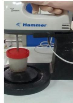
Figure 2. Mechanical mixing method (MM).
