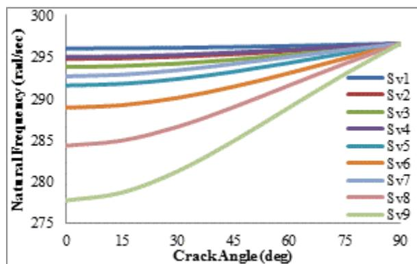
Figure 18. Numerical Results for hyper Composite beam's Natural Frequency with  $V_s = 15\%$ ,  $V_p = 15\%$ ,  $V_{resin} = 70\%$ .
