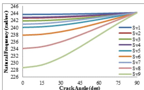
Figure 19. Numerical Results for hyper Composite beam's Natural Frequency with  $V_s = 0\%$ ,  $V_p = 30\%$ ,  $V_{resin} = 70\%$ .
