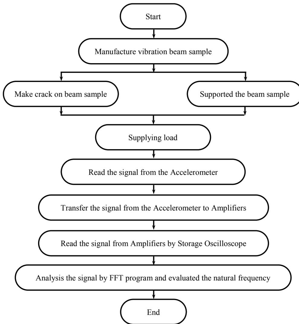
Figure 5. Flow Chart of stepping of vibration test beam.
