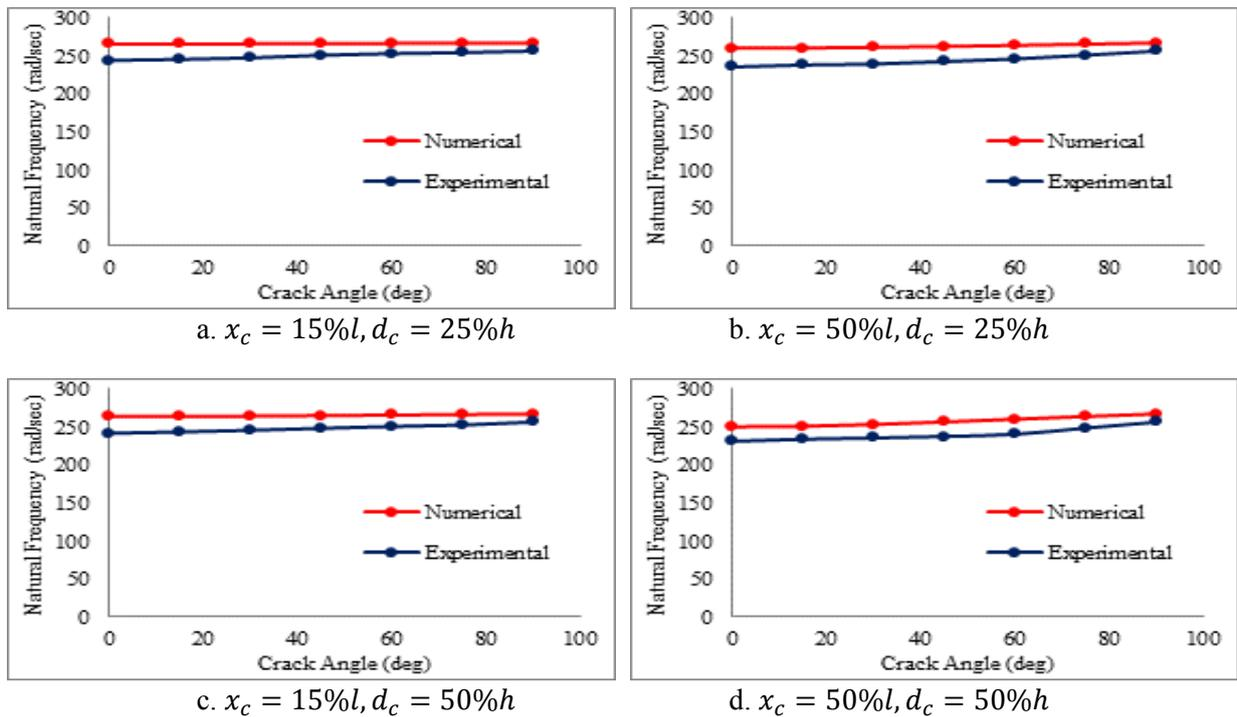
Figure 9. Numerical and experimental results for beam with  $V_s = 10\%, V_p = 10\%, V_{resin} = 80\%$ .
