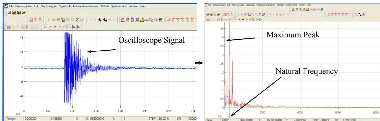
Figure 6. Analysis of storage oscilloscope signal by FFT.
