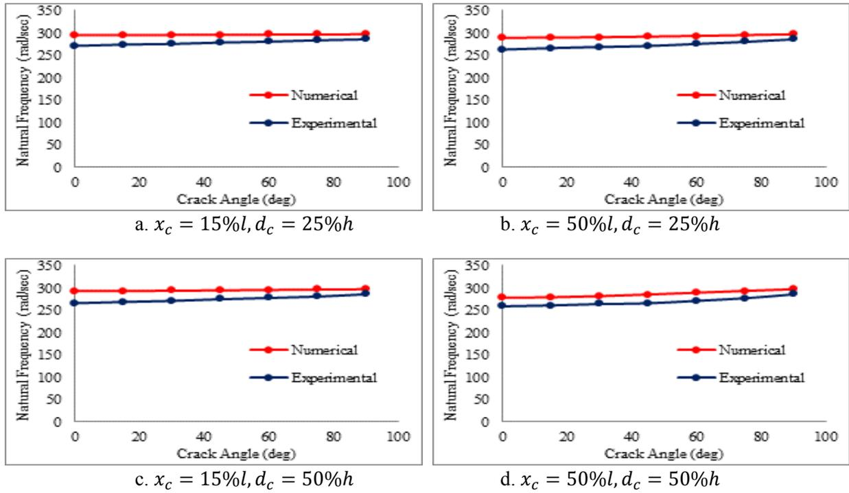
Figure 12. Numerical and experimental results for beam with  $V_s = 15\%, V_p = 15\%, V_{resin} = 70\%$ .
