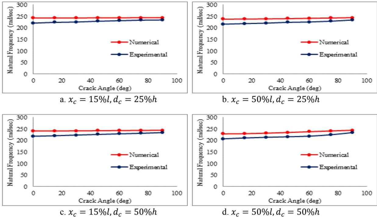
Figure 13. Numerical and experimental results for beam with  $V_s = 0\%, V_p = 30\%, V_{resin} = 70\%$ .
