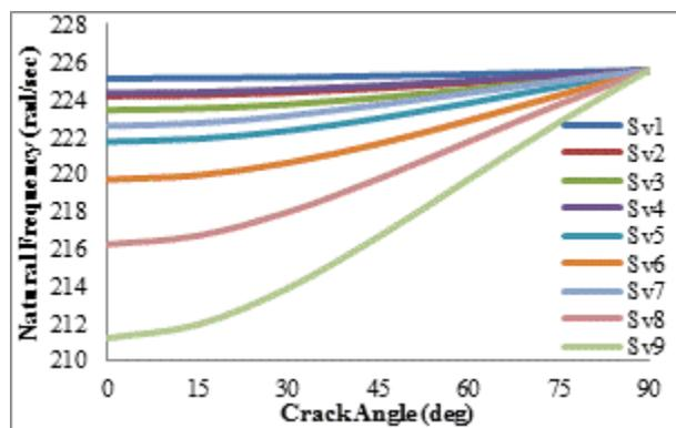
Figure 16. Numerical Results for Natural Frequency of hyper composite beam with  $V_s = 0\%$ ,  $V_p = 20\%$ ,  $V_{resin} = 80\%$ .
