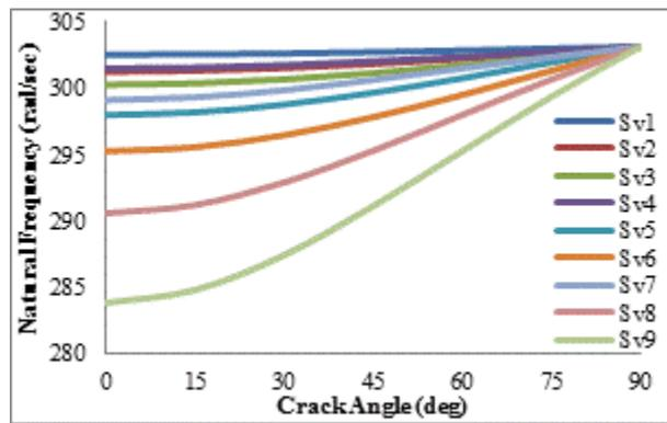
Figure 14. Numerical Results for hyper Composite beam's Natural Frequency with  $V_s = 20\%$ ,  $V_p = 0\%$ ,  $V_{resin} = 80\%$ .
