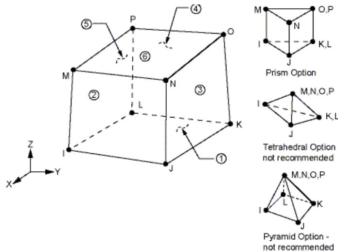
Figure 7. SOLID185 homogeneous structural solid geometry.
