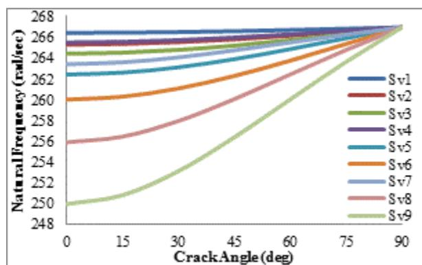
Figure 15. Numerical Results for hyper Composite beam's Natural Frequency with  $V_s = 10\%$ ,  $V_p = 10\%$ ,  $V_{resin} = 80\%$ .
