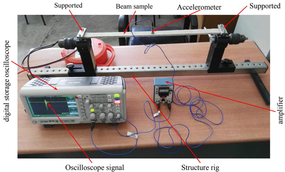
Figure 4. Vibration test machine.
