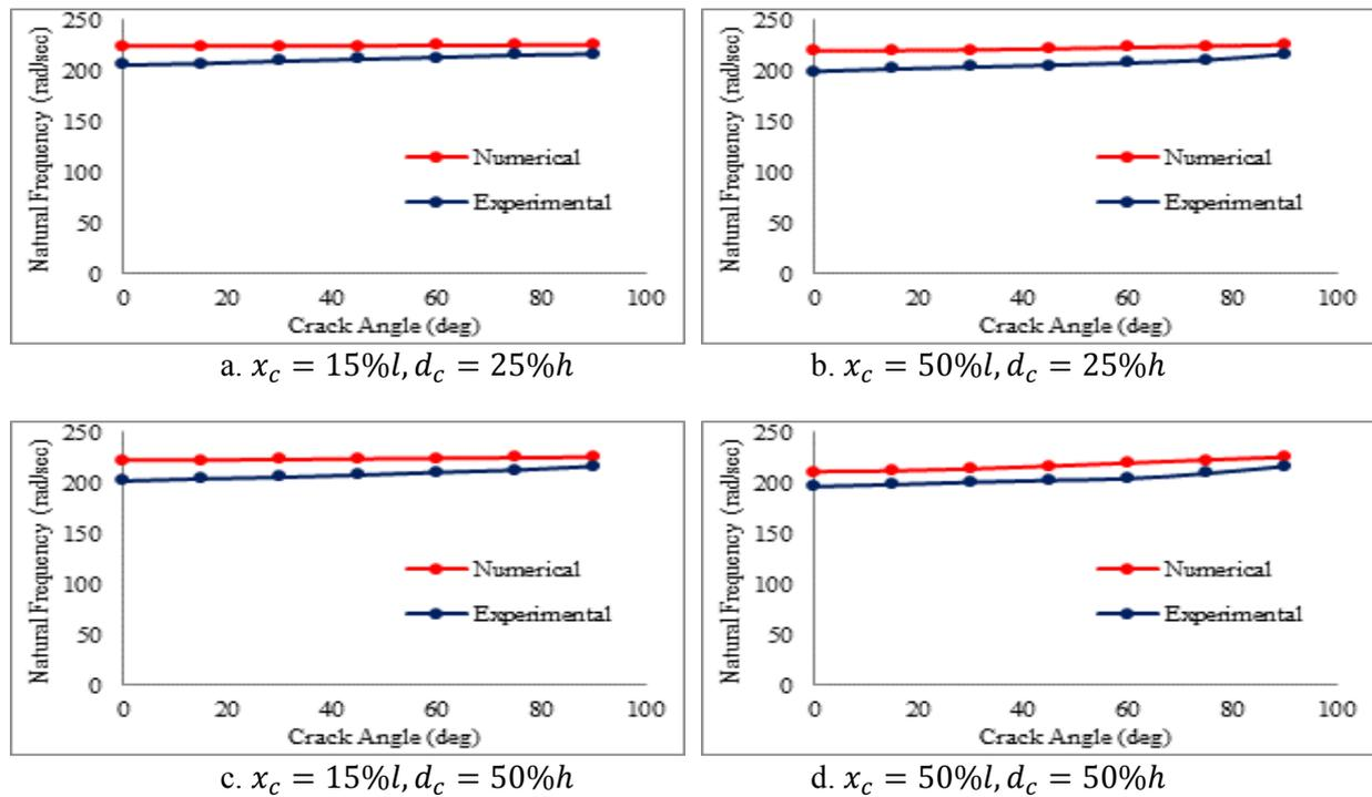
Figure 10. Numerical and experimental results for beam with  $V_s = 0\%$ ,  $V_p = 20\%$ ,  $V_{resin} = 80\%$ .
