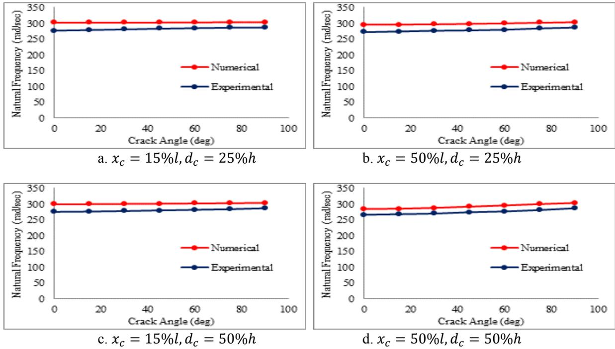
Figure 8. Numerical and experimental results for beam with  $V_s = 20\%, V_p = 0\%, V_{resin} = 80\%$ .
