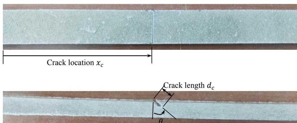
(b) Beam with crack effect.
