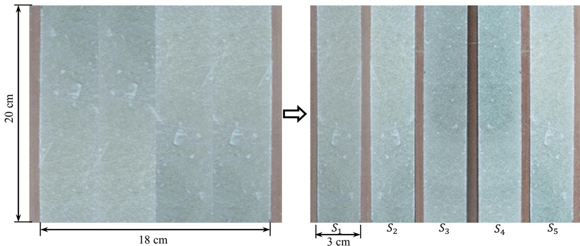
Figure 1. Tensile test sample.
