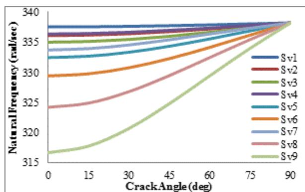
Figure 17. Numerical Results for Natural Frequency of hyper composite beam with  $V_s = 30\%$ ,  $V_p = 0\%$ ,  $V_{resin} = 70\%$ .
