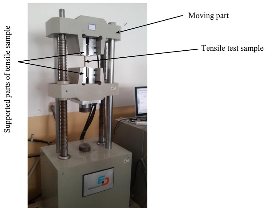
Figure 2. Tensile test machine.
