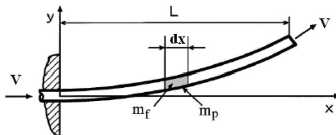
Figure 1. Cantilever pipe conveying fluid.
