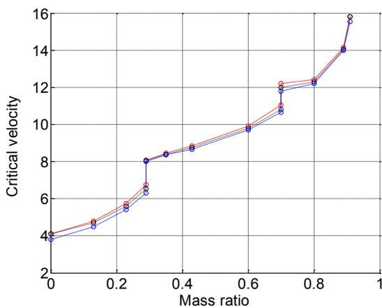
Figure 4. Stability map of cantilever pipe at different values of  $\gamma$ .
