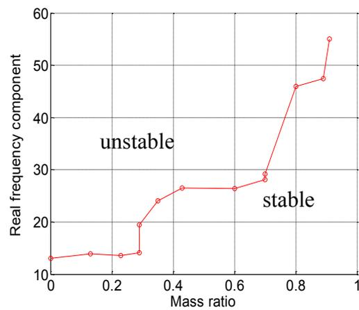
Figure 3. Real frequencies at critical velocities,  $\gamma = 0$ .
