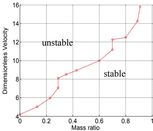
Figure 2. Stability map for cantilever pipe,  $\gamma = 0$ .
