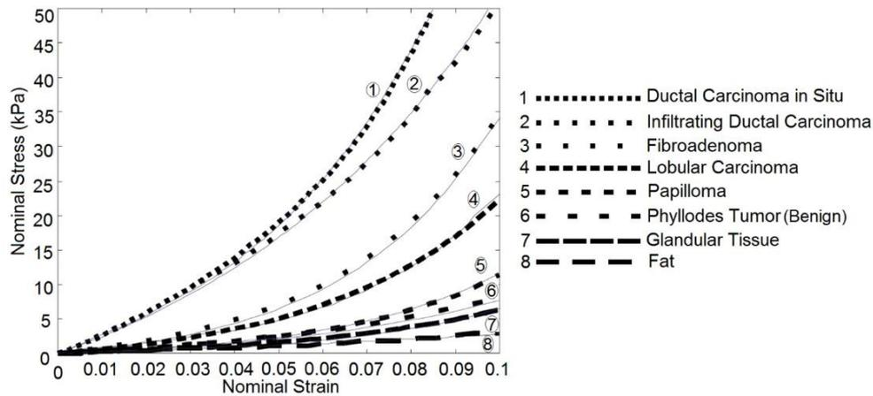
Figure 5. Experimental stress-strain curve [9].
