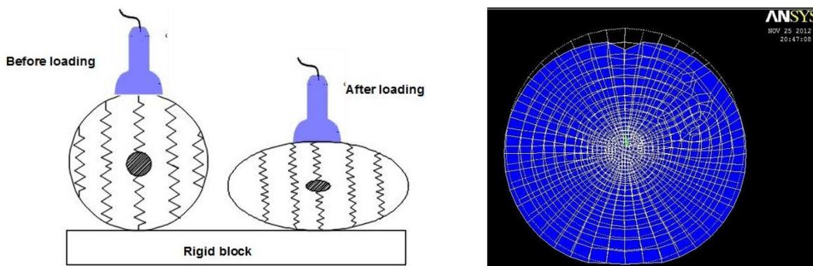
Figure 4. Finite element representative of the proposed model.
