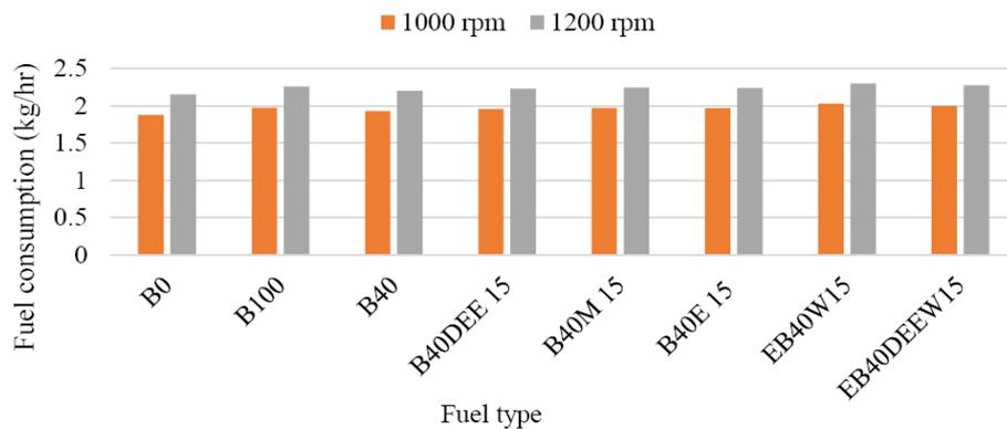
Figure 2. Fuel consumption of various fuel blends at different engine speeds.
