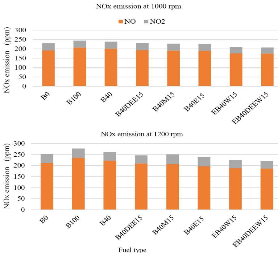
Figure 4. NOx emissions of various fuel blends at different engine speeds.
