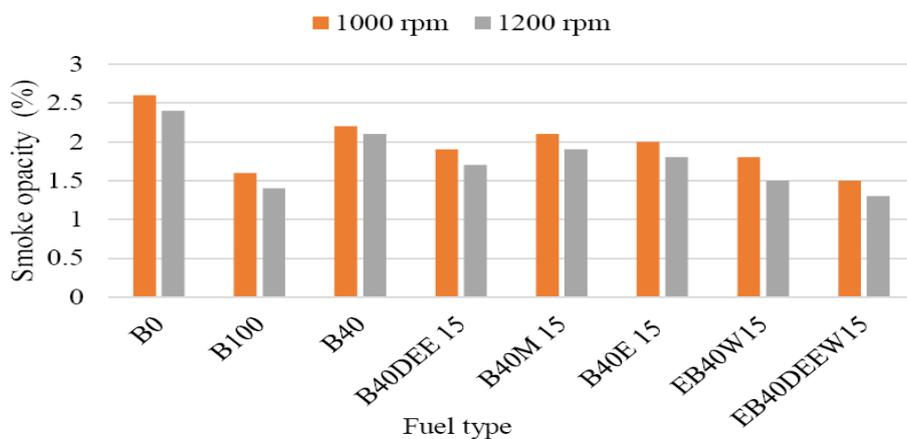
Figure 7. Smoke emissions of various fuel blends at different engine speeds.
