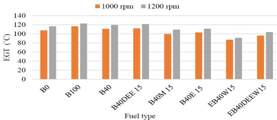
Figure 3. EGT of various fuel blends at different engine speeds.
