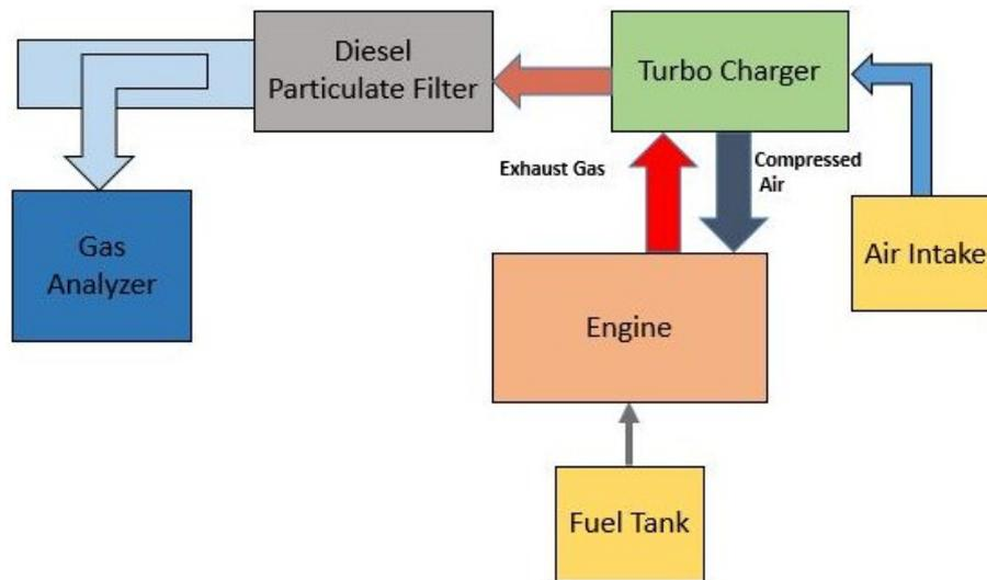
Figure 1. Schematic diagram of engine test.
