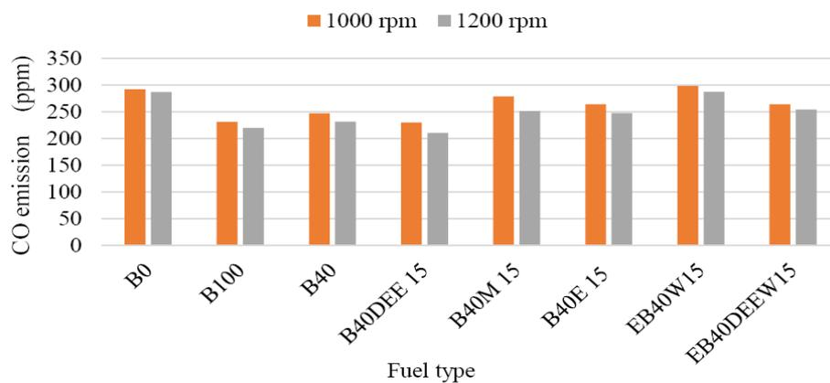
Figure 5. CO emissions of various fuel blends at different engine speeds.
