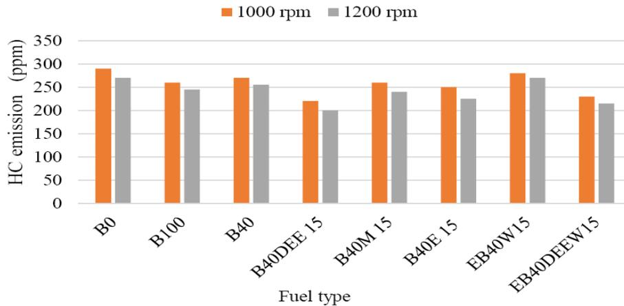
Figure 6. HC emissions of various fuel blends at different engine speeds.
