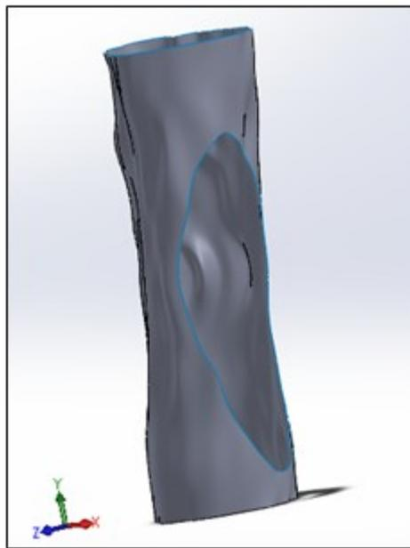
Figure 5. Syme's socket with elliptical cut-out.
