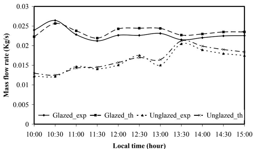
Figure 6. Comparison of experimental and theoretical air mass flow rate for both glazed and unglazed types.
