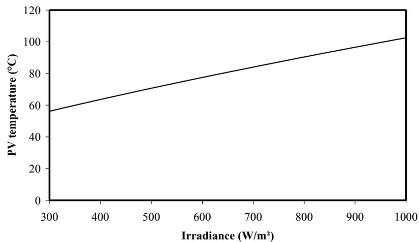
Figure 13. Variation of PV panel temperature with irradiance.
