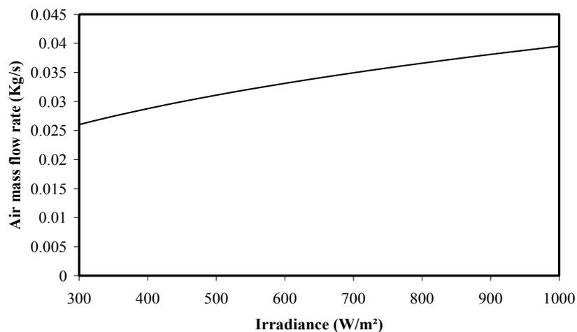
Figure 14. Variation of air mass flow rate with irradiance.
