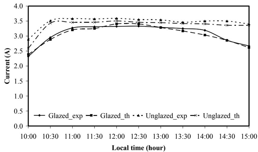
Figure 8. Comparison of experimental and theoretical operating current of the PV panels for both glazed and unglazed types.
