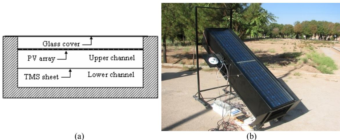
Figure 1. The studied PV/T air collector (a) a Cross-sectional schematic view; (b) Photograph of experimental setup.
