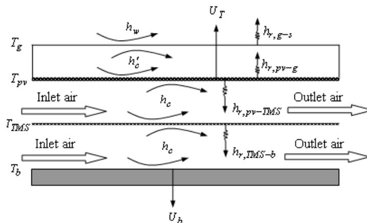
Figure 2. Schematic of the studied PV/T air system with heat transfer coefficients.
