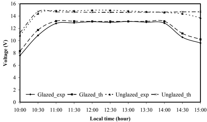
Figure 7. Comparison of experimental and theoretical operating voltage of the PV panels for both glazed and unglazed types.
