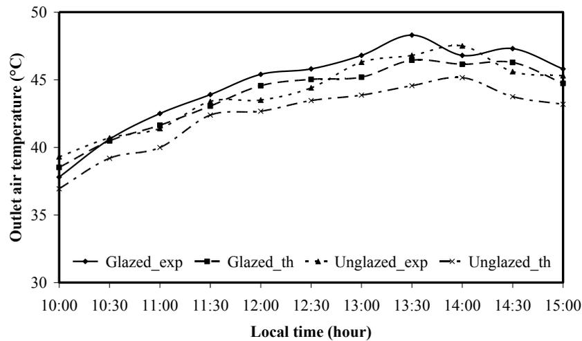
Figure 4. Comparison of experimental and theoretical outlet air temperature for both glazed and unglazed types.
