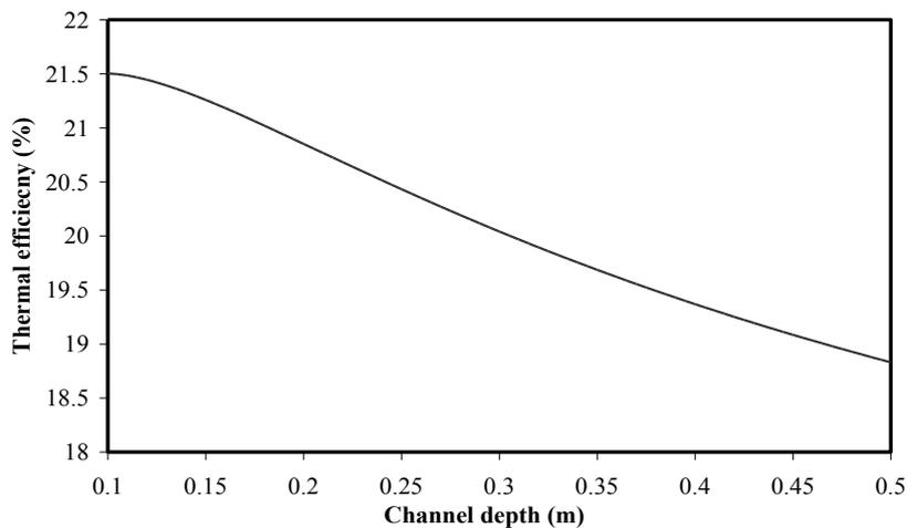
Figure 16. Effect of channel depth on the thermal efficiency.
