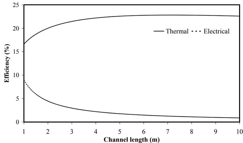
Figure 18. Effect of channel length on the thermal and electrical efficiency.
