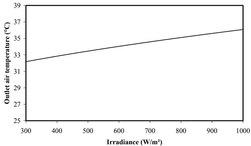
Figure 12. Variation of outlet air temperature with irradiance.
