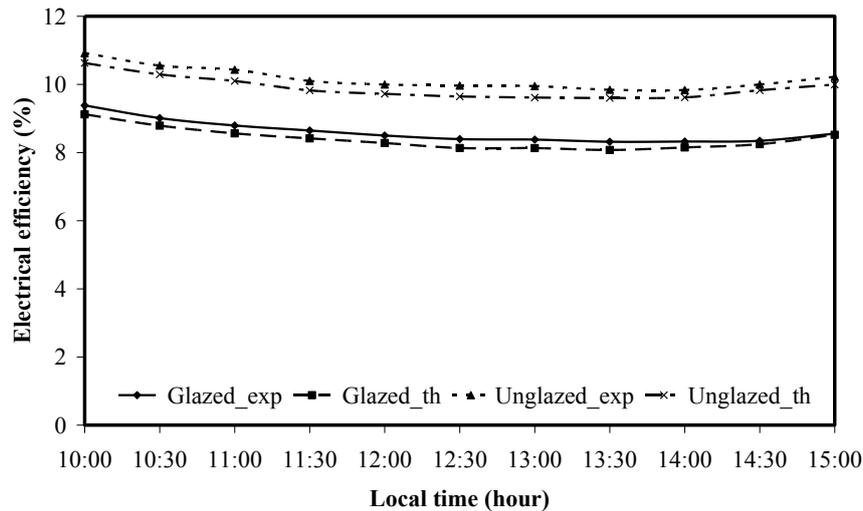
Figure 10. Comparison of experimental and theoretical electrical efficiency for both glazed and unglazed types.
