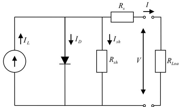
Figure 3. The equivalent circuit for a PV generator.
