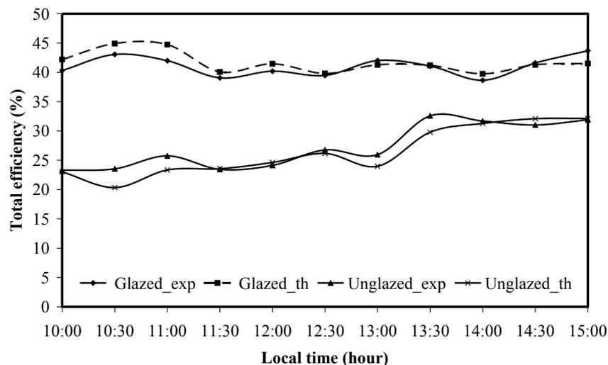
Figure 11. Comparison of experimental and theoretical total efficiency for both glazed and unglazed types.
