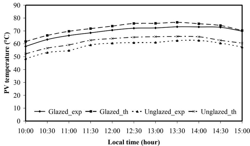
Figure 5. Comparison of experimental and theoretical PV panel temperature for both glazed and unglazed types.
