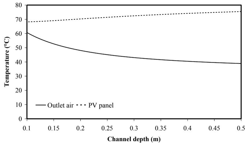
Figure 15. Effect of channel depth on the outlet air and PV panel temperature.
