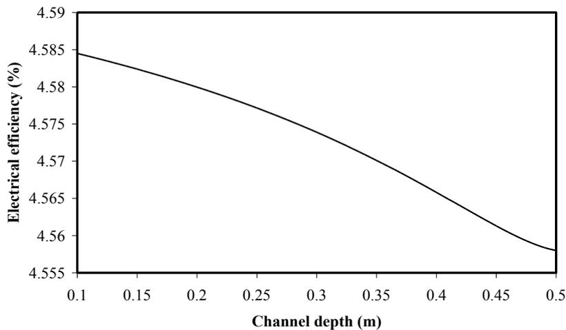
Figure 17. Effect of channel depth on the electrical efficiency.
