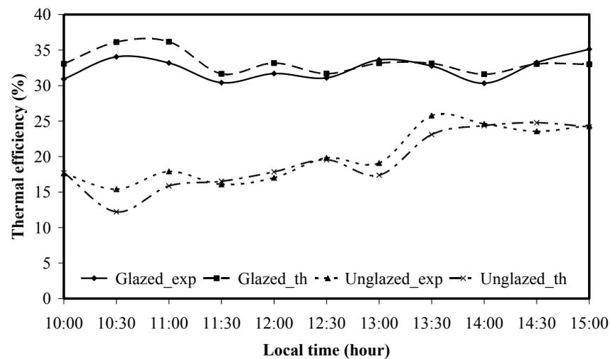
Figure 9. Comparison of experimental and theoretical thermal efficiency for both glazed and unglazed types.
