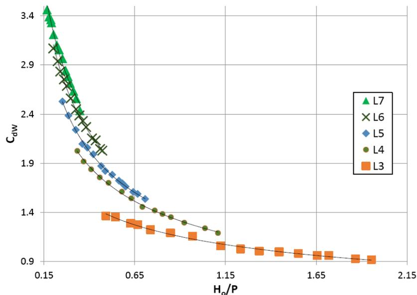
Figure 3. Variation of  $C_{dw}$  vs.  $H_o/P$  for five ratios of  $L/W$ .
