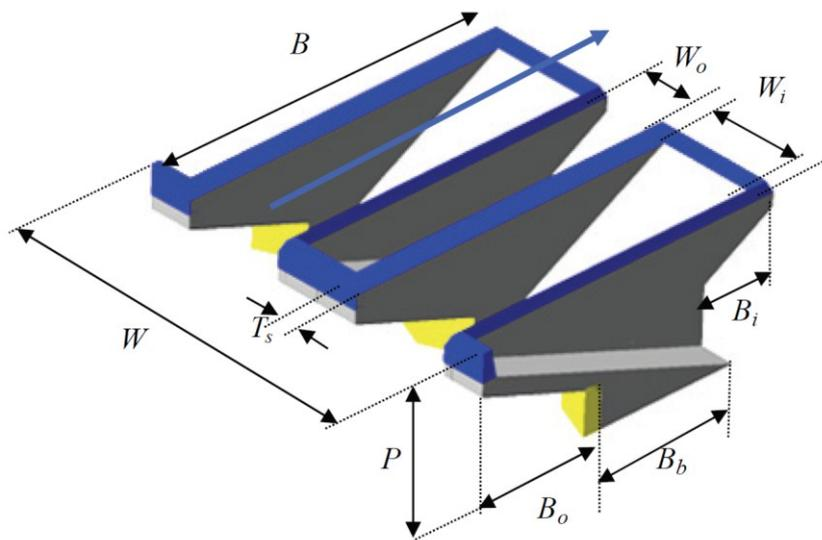
Figure 1. Sketch of PKW geometry [3].
