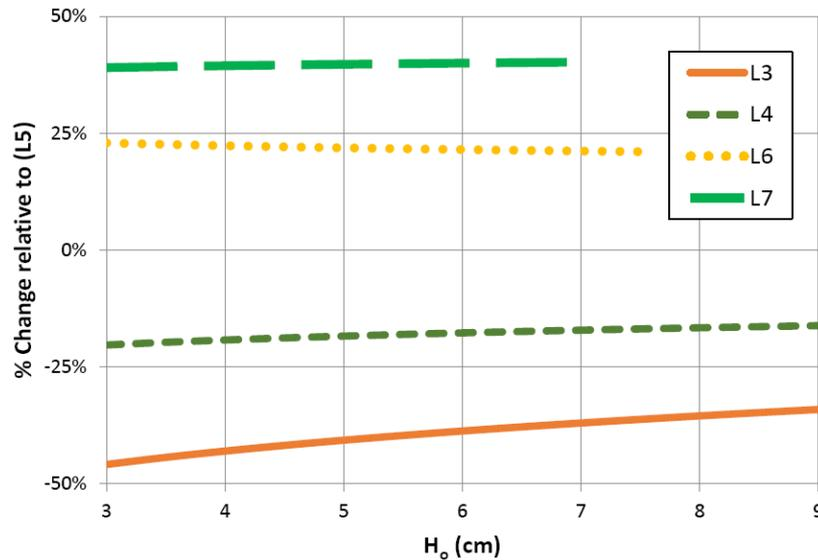
Figure 5. Percentage change of  $C_{dw}$  vs.  $H_o$  relative to model L5.
