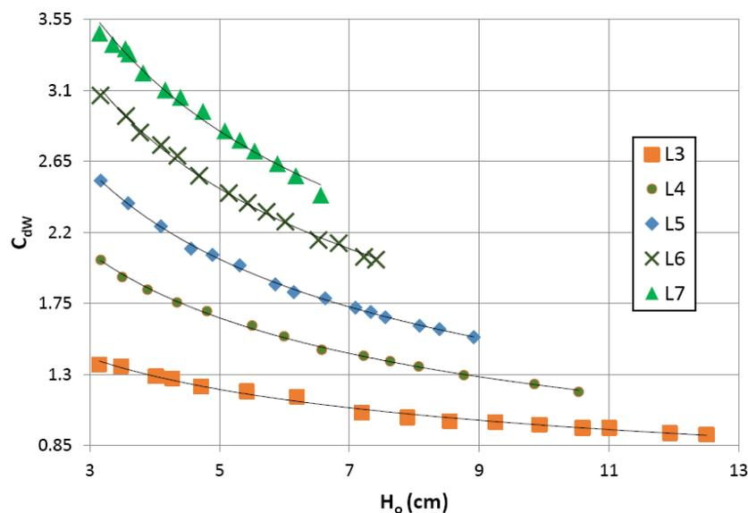
Figure 4. Variation of  $C_{dw}$  vs.  $H_o$  for five ratios of  $L/W$ .
