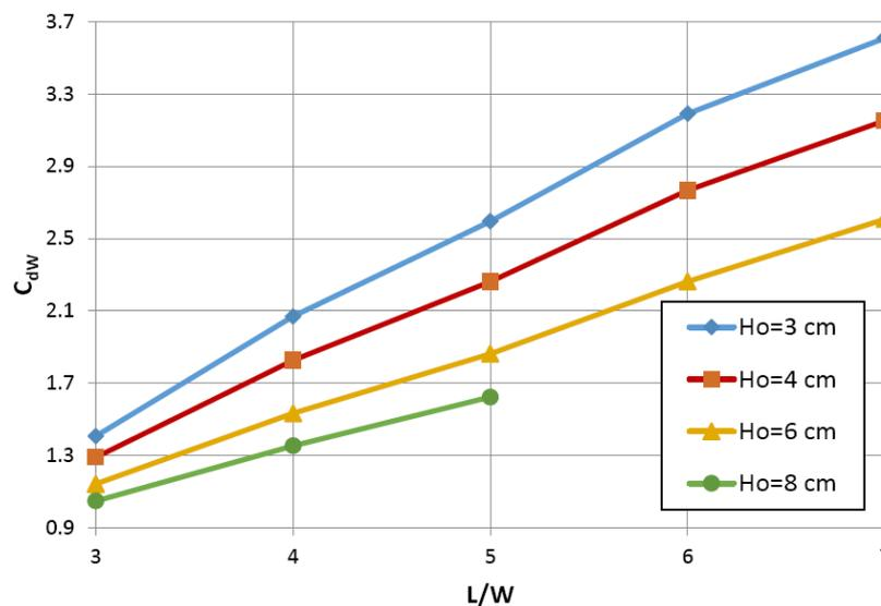
Figure 6. Variation of  $L/W$  vs.  $C_{dw}$  for different values of the head  $H_o$ .
