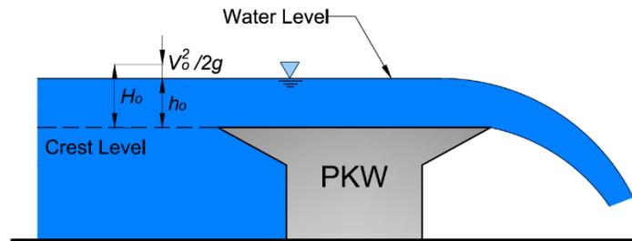
Figure 2. Sketch of the flow over PKW.
