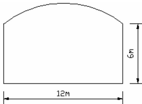
Figure 1. The cross-sectional profile of tunnel
