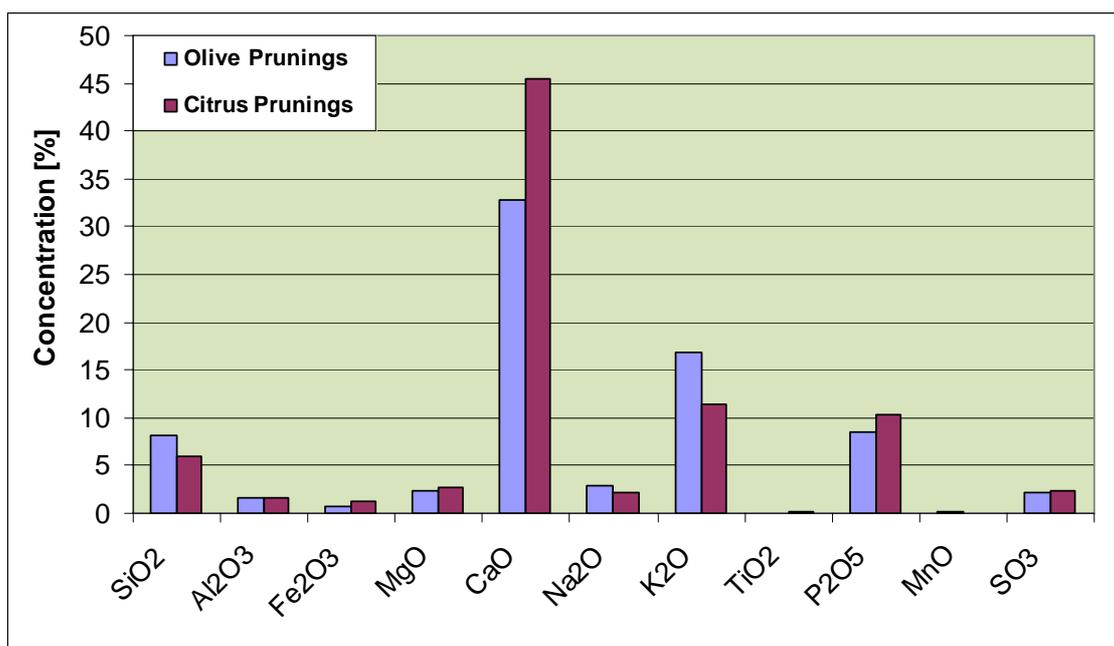
Figure 3. Main components (represented as oxides) of fly ashes of biomass samples
