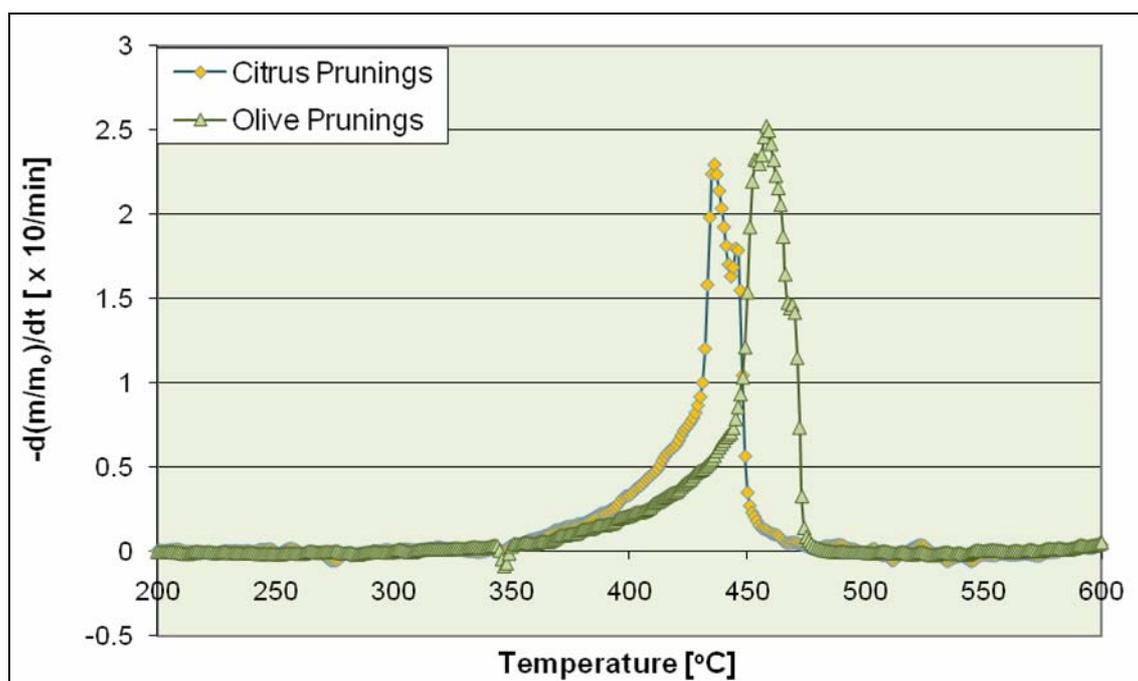
Figure 1. DTG burning profiles of biomass samples
