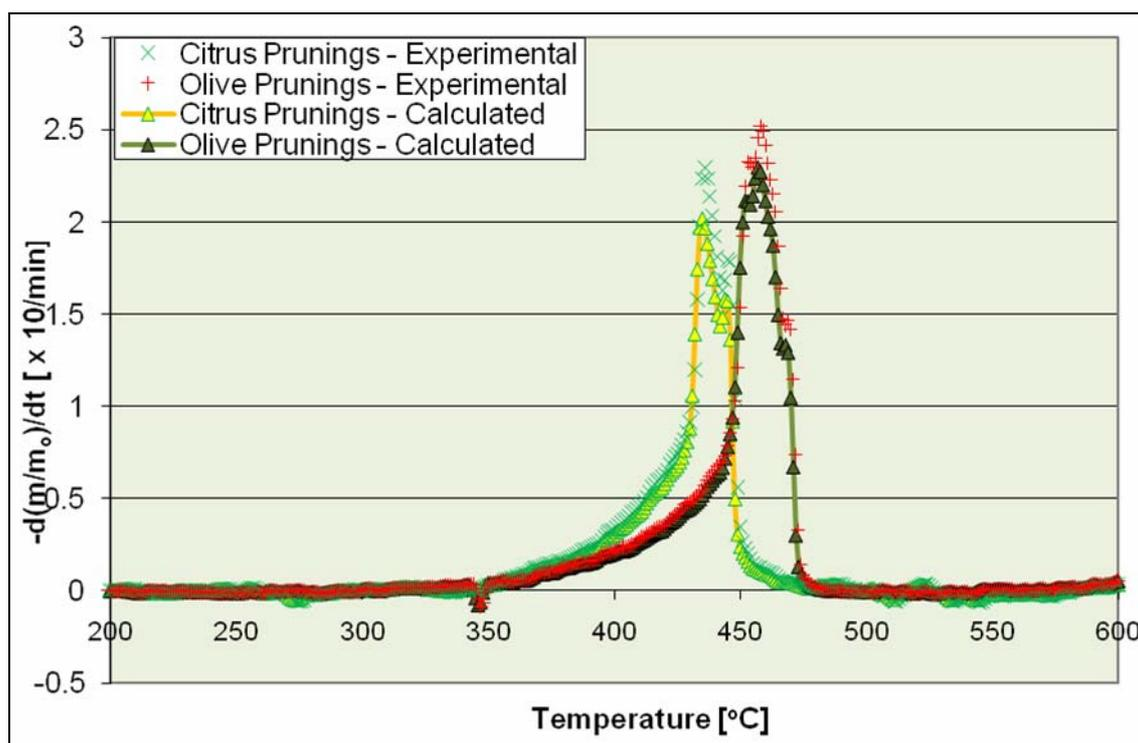
Figure 2. Experimental and calculated DTG burning profiles of biomass samples
