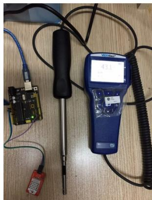
Figure 2. Calibration of DHT22 sensor.
