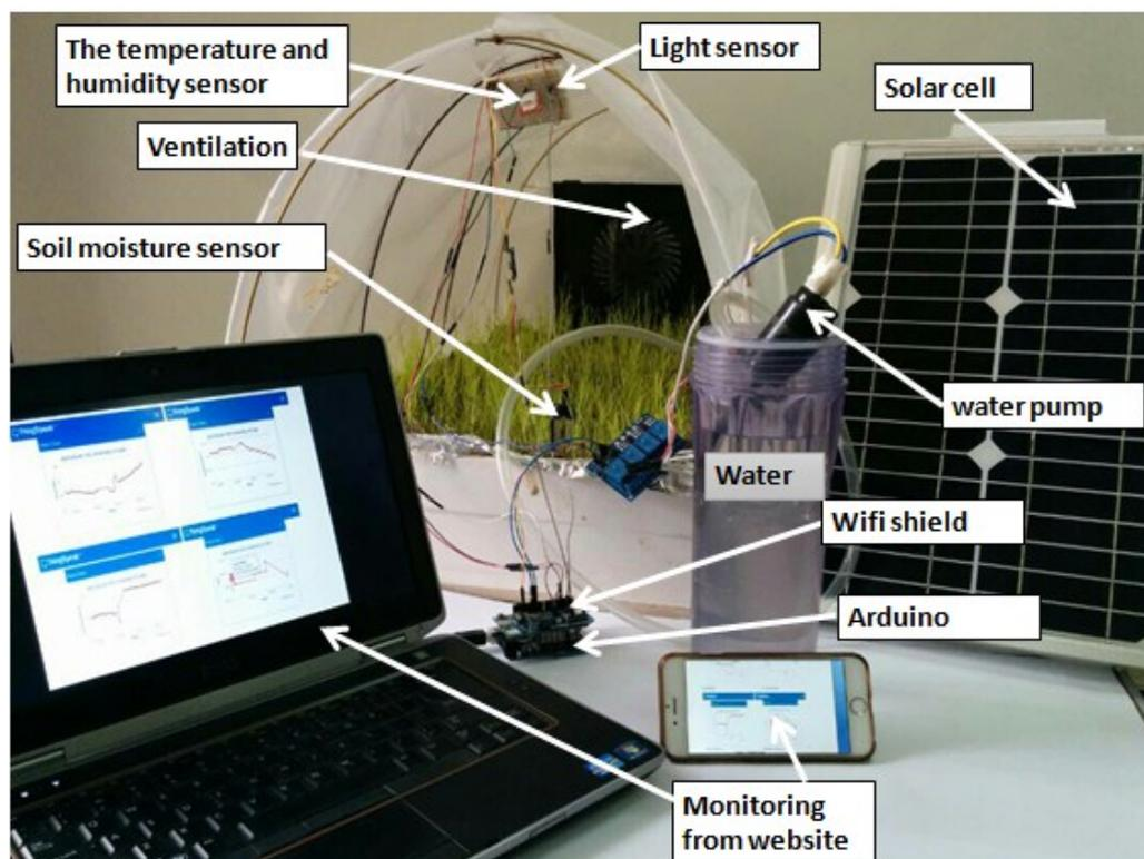
Figure 3. Smart greenhouse prototype.
