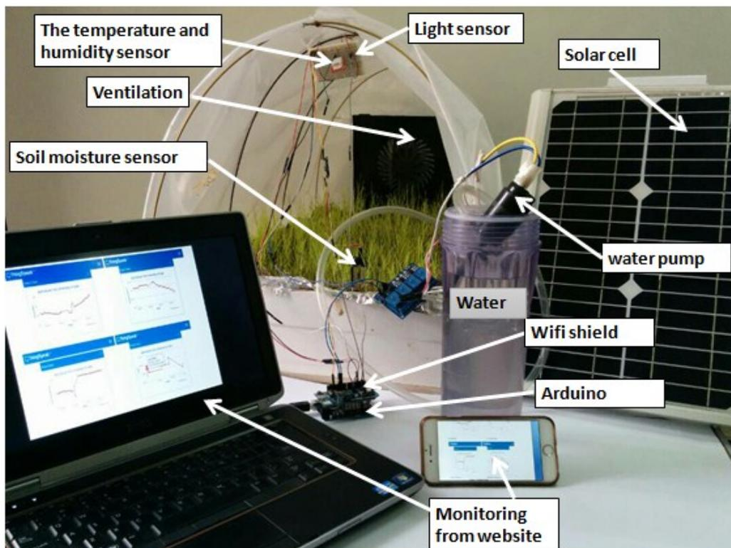
Figure 3. Smart greenhouse prototype.
