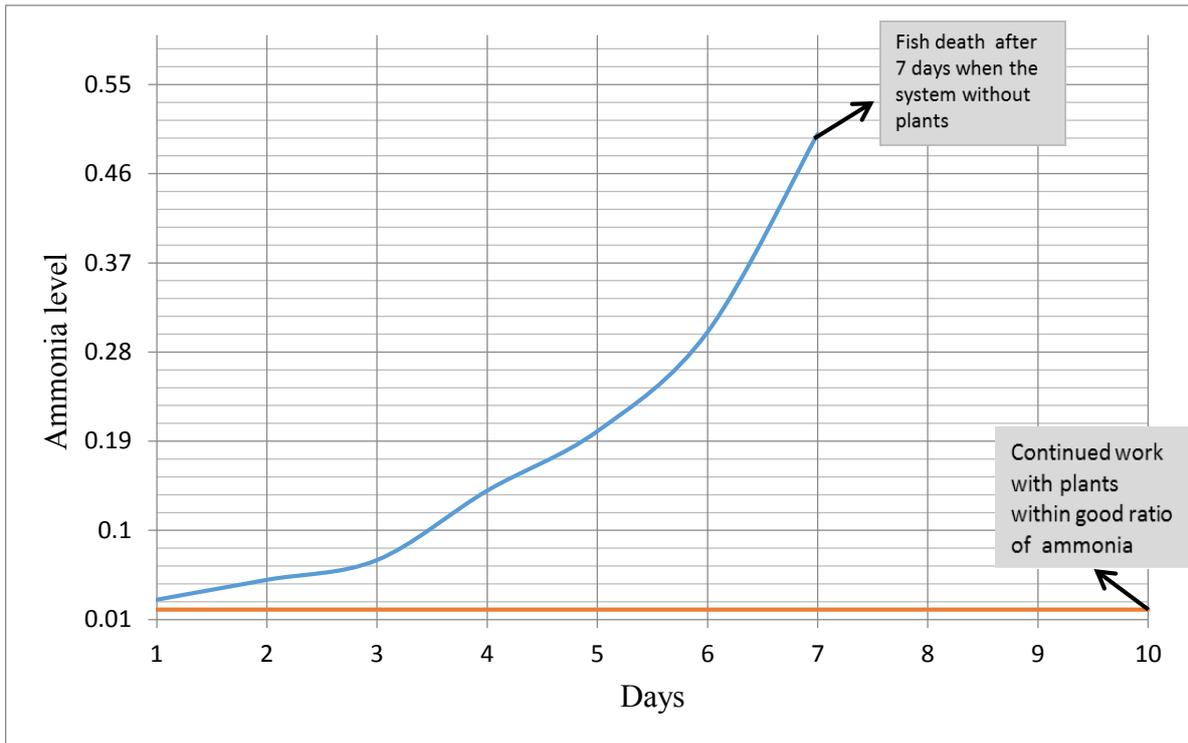
Figure 7. Graph showing ammonia level of the system.
