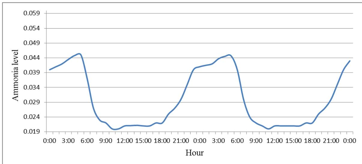
Figure 9. Graph showing ammonia level of the system during the night and day.
