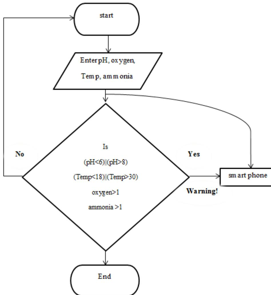
Figure 2. Flow diagram of the proposing system.
