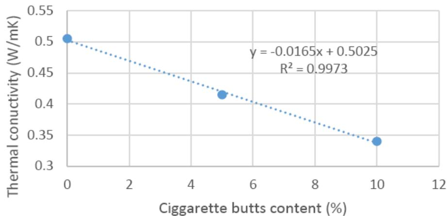
Figure 5. The dependence of the thermal conductivity on butts content.
