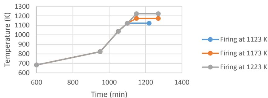
Figure 1. Regime for the firing of samples.
