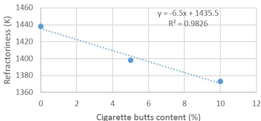
Figure 6. The dependence of the refractoriness on butts content.
