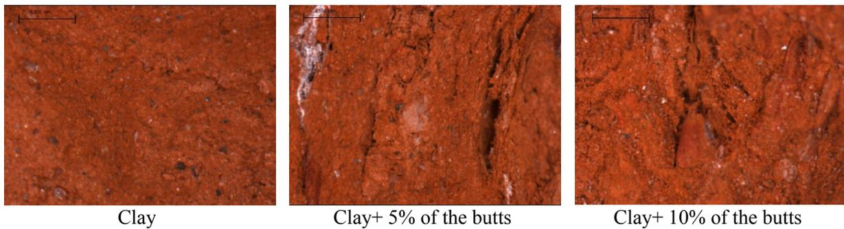
Figure 7. Recordings of clay and clay with cigarette butts on the optical microscope.
