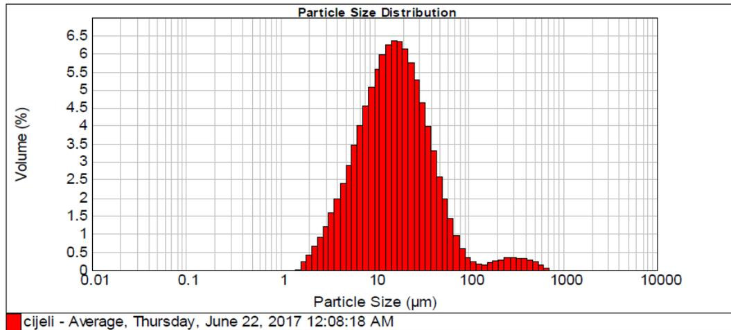
Figure 3. Particle size distribution of the clay “Čavka”.
