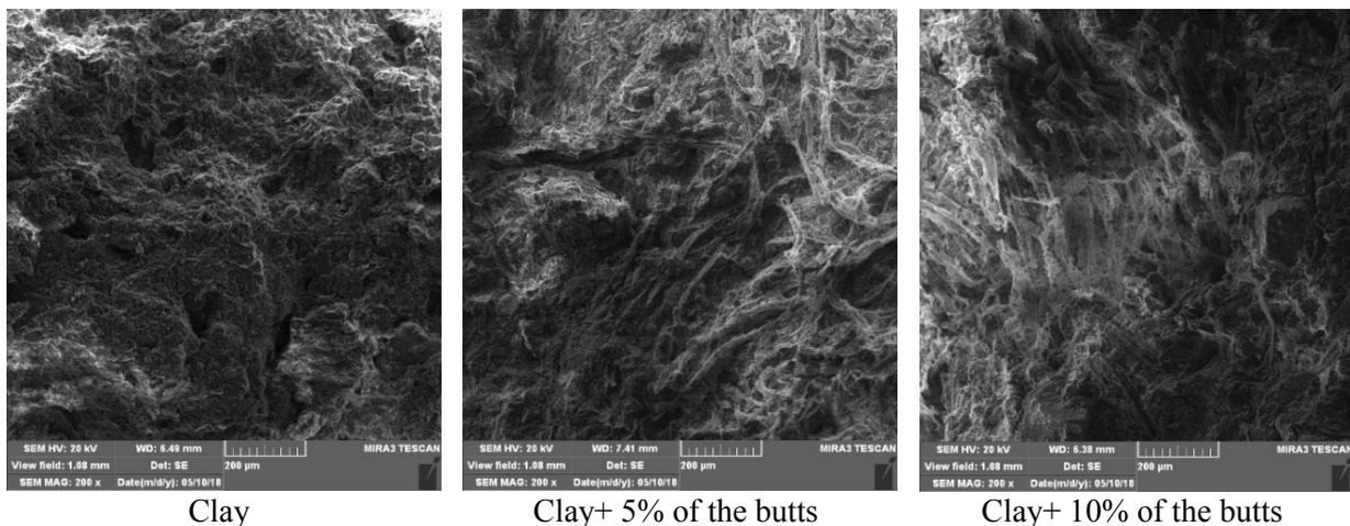
Figure 8. SEM of the clay sample and samples of the clay with butts addition.
