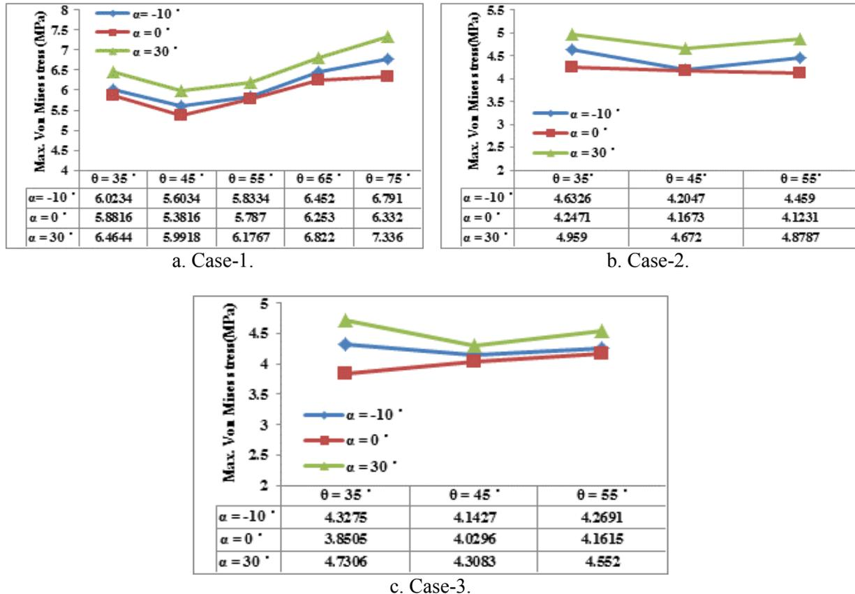
Figure 12. Maximum Von-Mises Stresses (MPa) for Hip Joint System with Different Phase and Inclinations Angle Effect, and Various Hip Cases.
