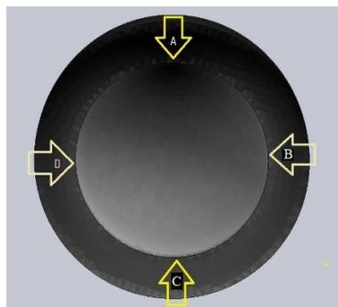
Figure 10. Sensors Positions on the Polyethylene Liner by Solid-Works.
