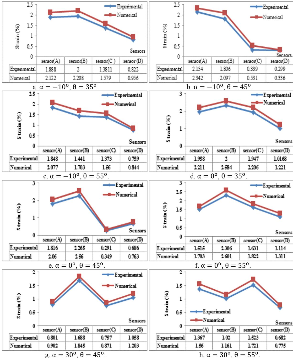
Figure 11. Comparison for Experimental and Numerical Strain Results ( $\times 10^{-1}$ ) for Hip Joint, with Various Phase and Linear Inclination Angle Effect.
