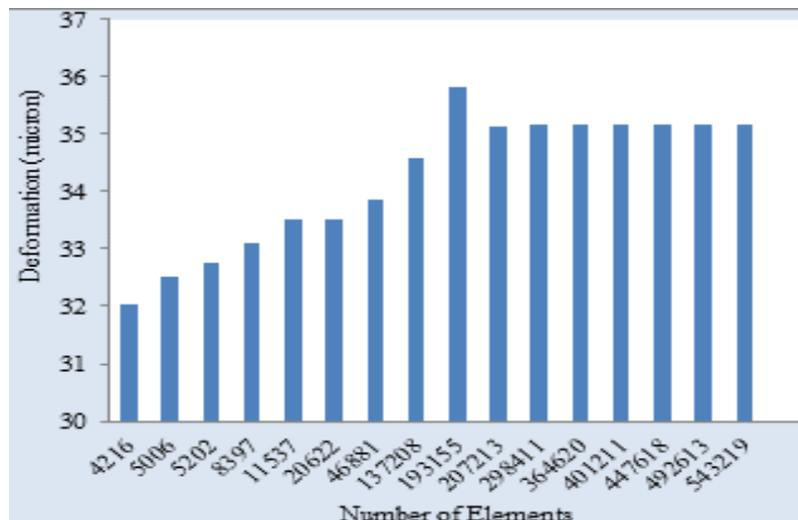
Figure 6. Degree of Freedom Stability with Number of Mesh Elements.
