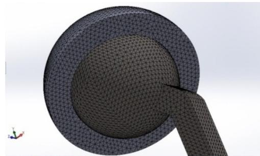
Figure 5. The Ball and Liner Socket Mesh Element.
