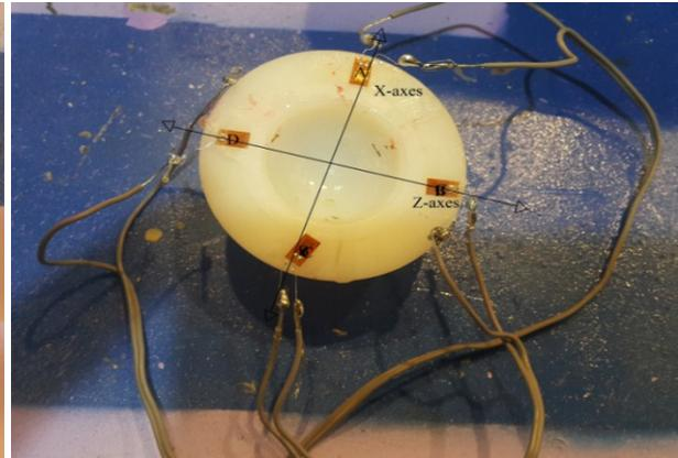
Figure 9. Strain Gauges Directions (x and y-axis).
