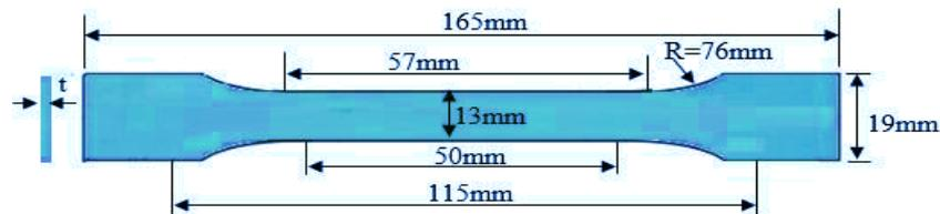
Figure 1. The ASTM D638 dimensions of a tensile specimen.
