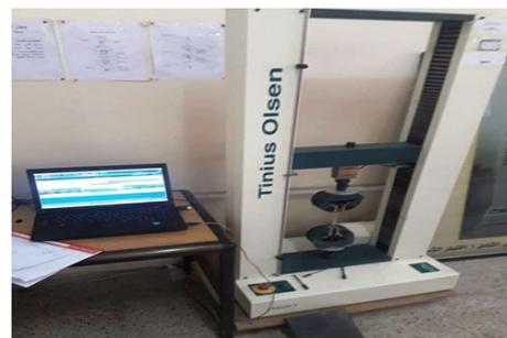
Figure 3. Tensile test setup.
