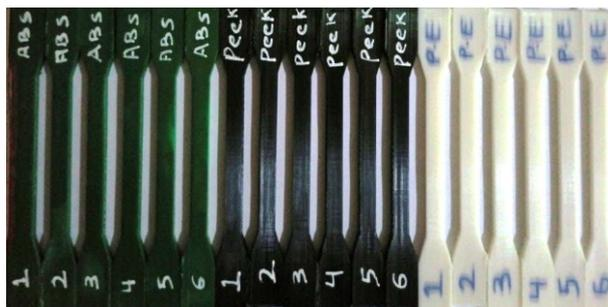
Figure 2. Tensile specimens manufactured by a 3D printing method.
