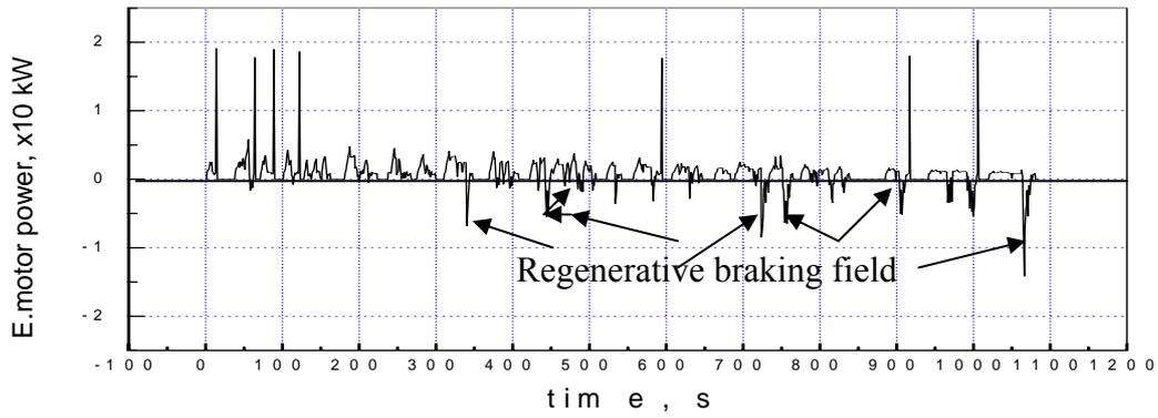
Figure 6. Power of electric motor during the city driving cycle
