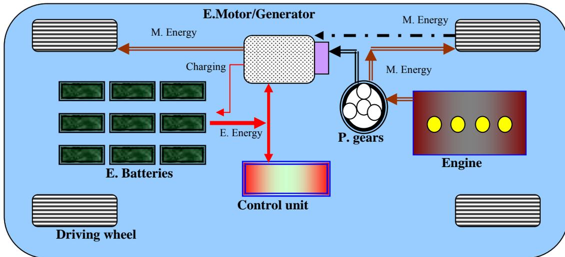
Figure 1. Main mechanical and electric components of hybrid electric vehicle
