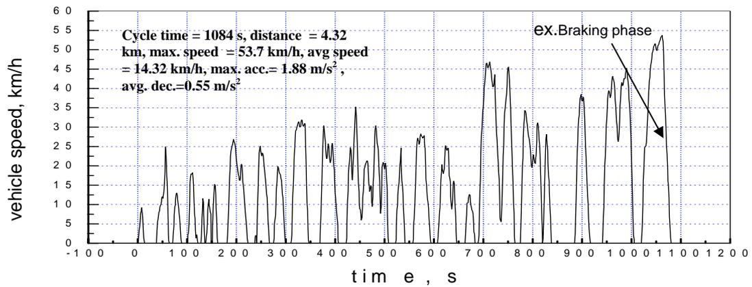
Figure 3. Vehicle speed against time of city cycle
