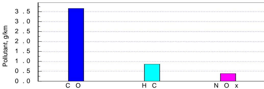
Figure 9. Exhaust emission of HEV during the driving cycle
