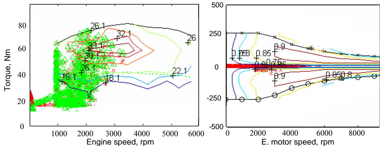
Figure 10. Operating points of hybrid electric vehicle on Engine and Electric motor map
