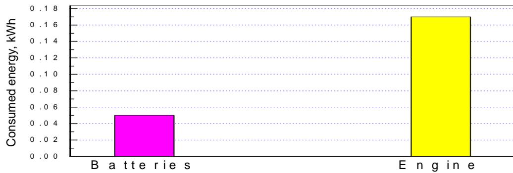
Figure 8. Consumed energy of the traction batteries and the IC engine
