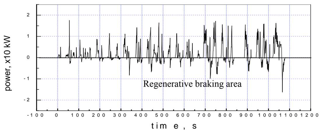
Figure 5. Power of electric controller during the city driving cycle
