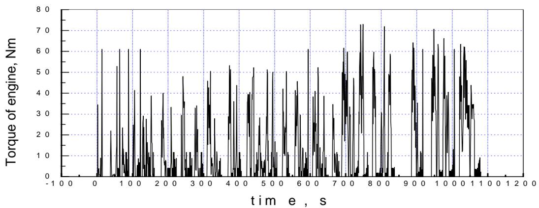
Figure 4. Torque of IC engine during the city driving cycle
