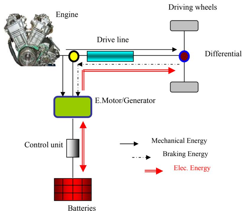
Figure 2. Schematic diagram of HEV configuration
