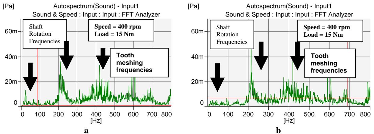
Figure 10. Locations of tooth meshing and shaft rotation frequencies: (a) healthy gear; and (b) faulty gear (g4), 3.0 x 0.5 x 40 mm
