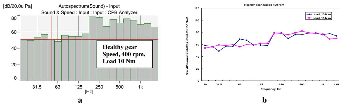
Figure 6. 1/3-Octave sound pressure level spectra: (a) 1/3-octave sound pressure level; and (b) 1/3-octave sound pressure level
