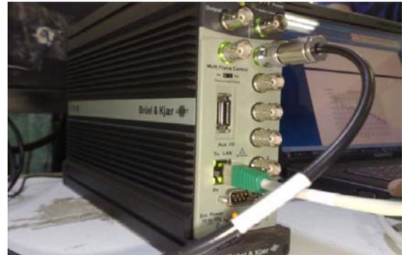
Figure 2. Bruel &amp; Kjaer (B&amp;K) portable and multi-channel PULSE
