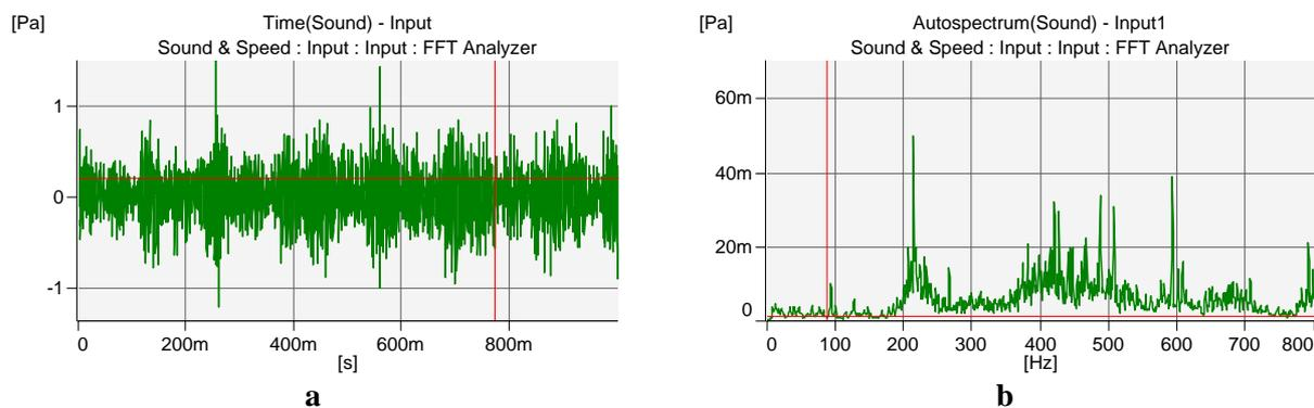
Figure 5. Sound pressure level spectra: (a) time history of sound pressure level; (b) frequency domain of sound pressure level
