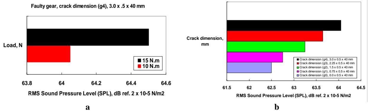
Figure 9. RMS sound pressure level: (a) influence of load; and (b) influence of crack dimension
