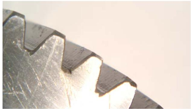
Figure 4. Gear tooth crack
