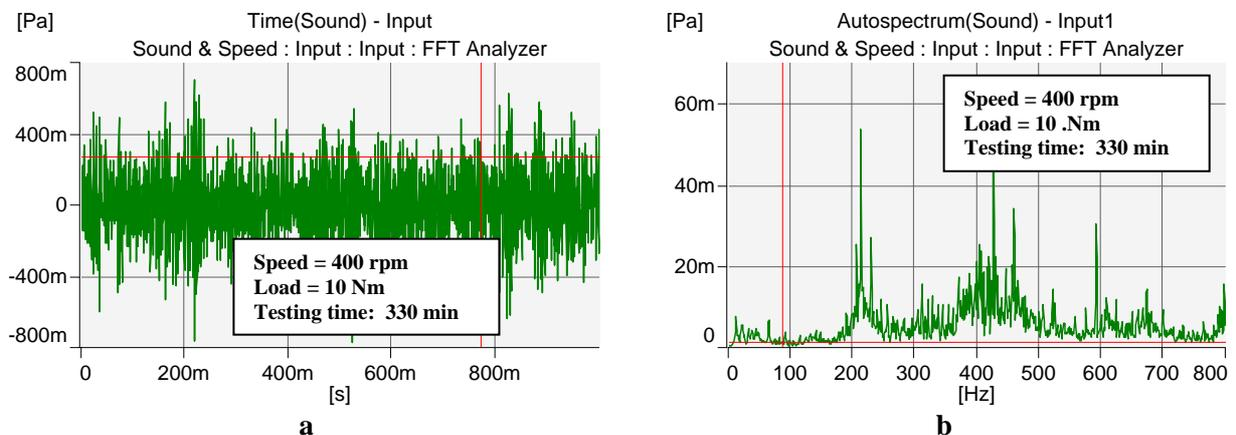
Figure 11. Sound pressure level spectra: (a) time history (g4), 3.0 x 0.5 x 40 mm; and (b) frequency domain (g4), 3.0 x 0.5 x 40 mm
