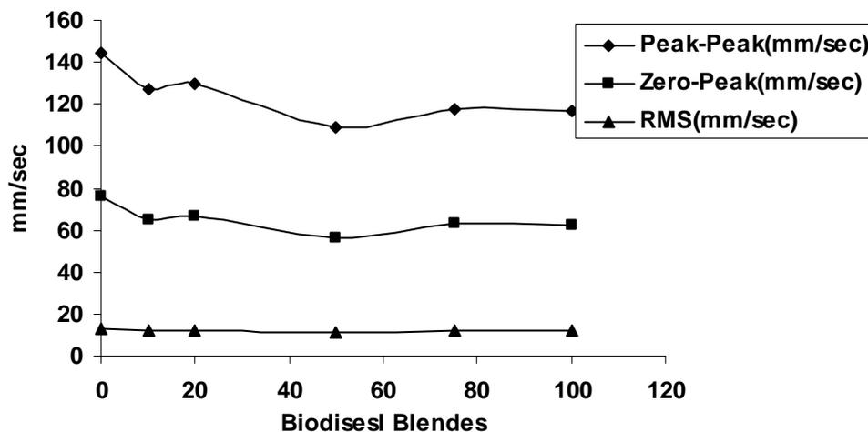
Figure 10. Effect of blend ratio on vibrations (axial)
