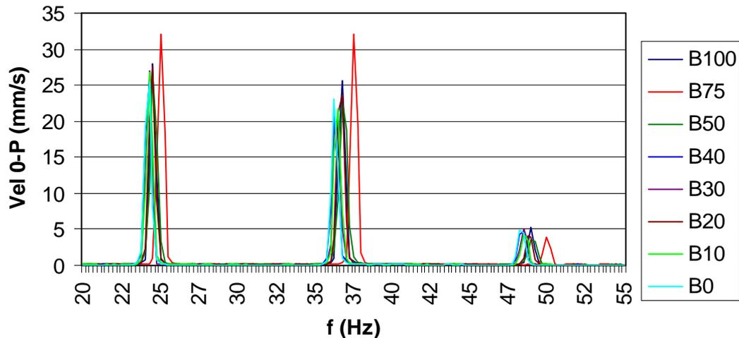
Figure 11. Mechanical spectrum for different blend ratio (lateral)
