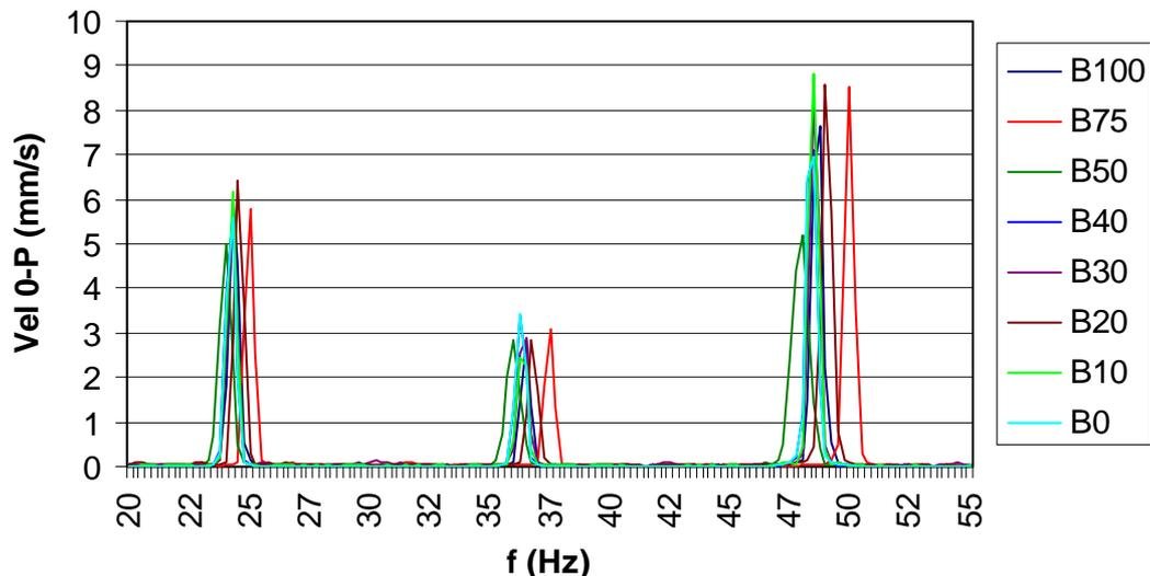
Figure 12. Mechanical spectrum for different blend ratio (axial)
