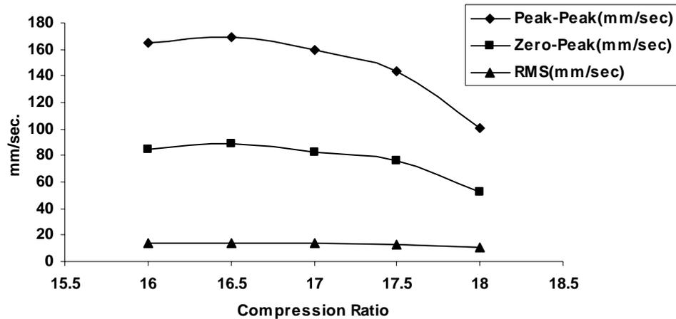
Figure 6. Effect of compression ratio on vibrations (axial)
