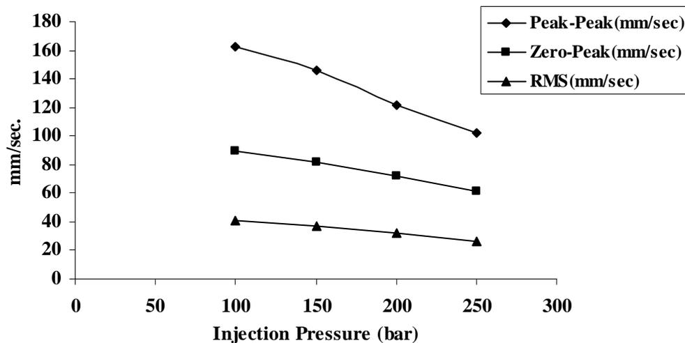
Figure 7. Effect of Injection pressure on vibrations (lateral)
