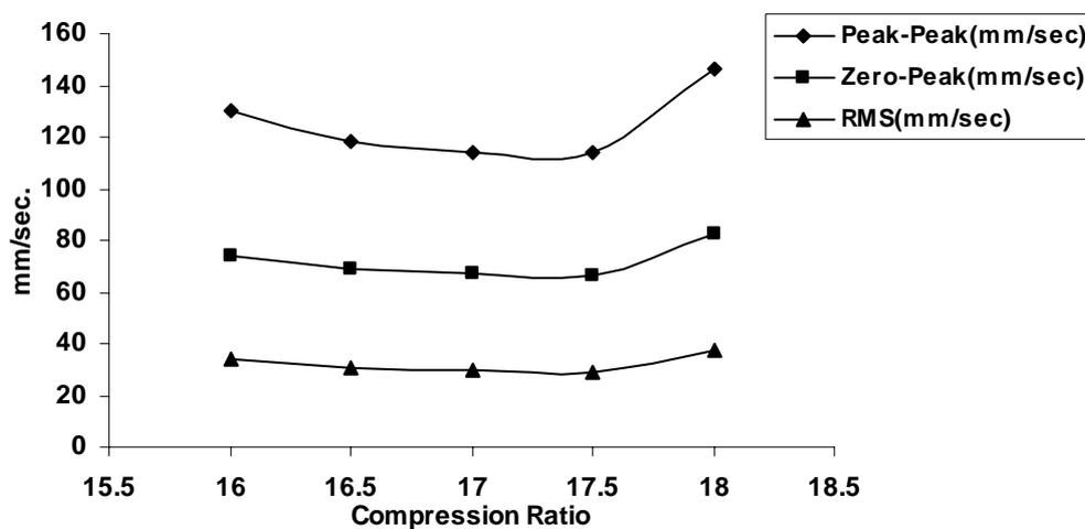
Figure 5. Effect of compression ratio on vibrations (lateral)
