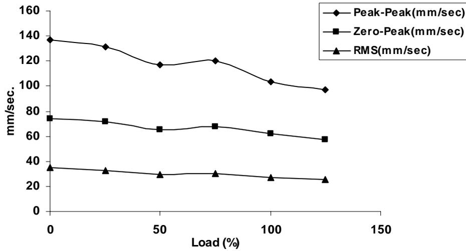
Figure 3. Effect of brake load on vibrations (lateral)
