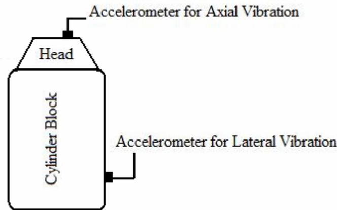
Figure 1. Positions of accelerometer
