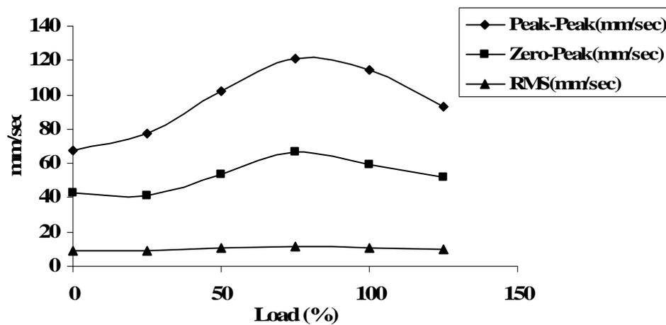
Figure 4. Effect of brake load on vibrations (axial)
