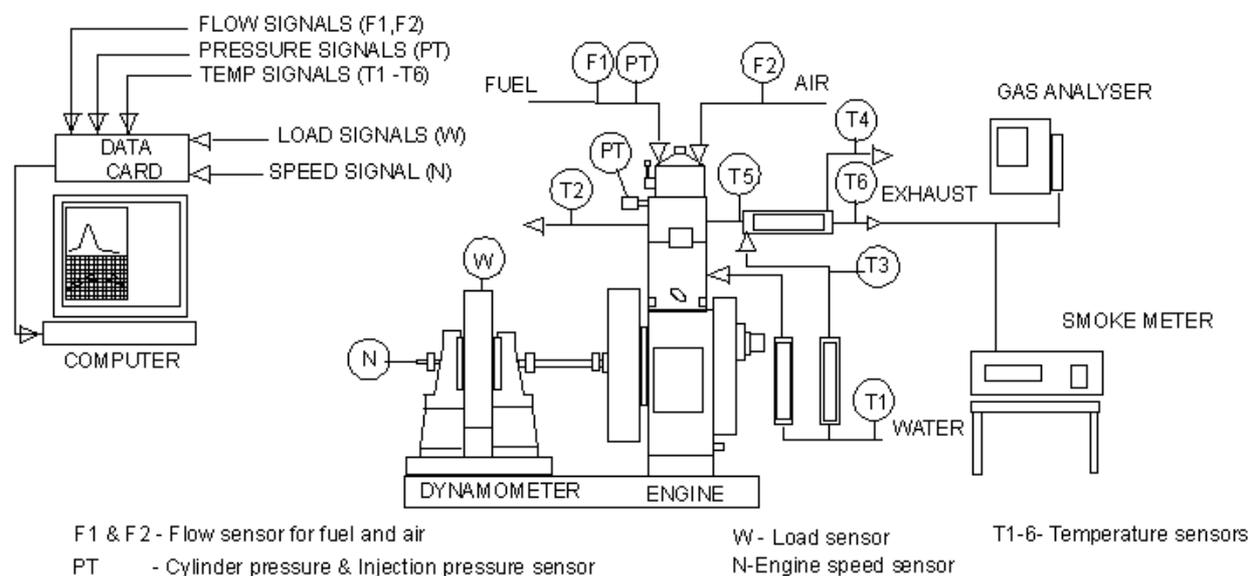
Figure 2. Engine test setup
