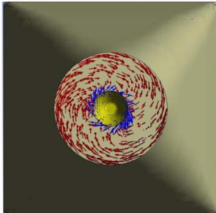
Figure 2. Boundary conditions in the inlet of the draft tube, where in red there are the exported data of the numerical simulation of the runner, and in blue the rotation of the machine. The intensity of the vectors is not being considered in that illustration
