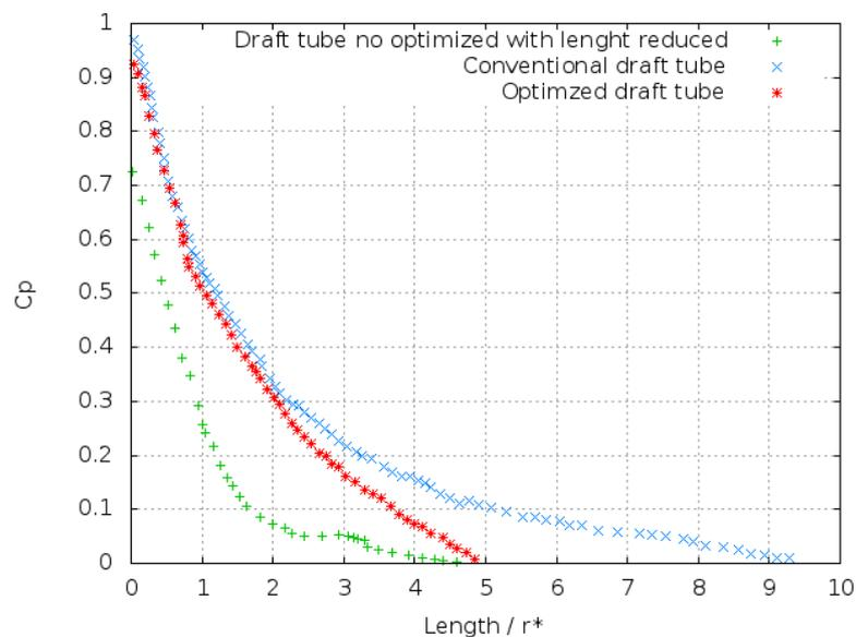
Figure 9. Comparison among  $C_p$ 's, where  $r^*$  is the ray of the inlet of the draft tube
