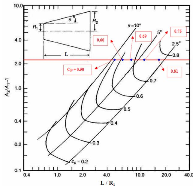
Figure 3. Comparison between  $C_p$  recovered numerically and experimental data [14]
