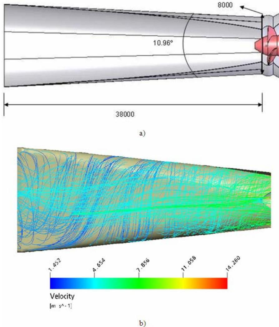
Figure 4. Dimensions of the draft tube, in mm (a) and the stream line (b)
