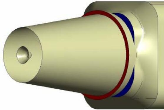
Figure 7. Illustration of the secondary inlets, where the first is shown in red color and the second in blue color
