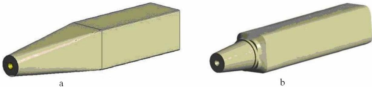
Figure 1. Conventional draft tube (a) and Optimized draft tube (b)
