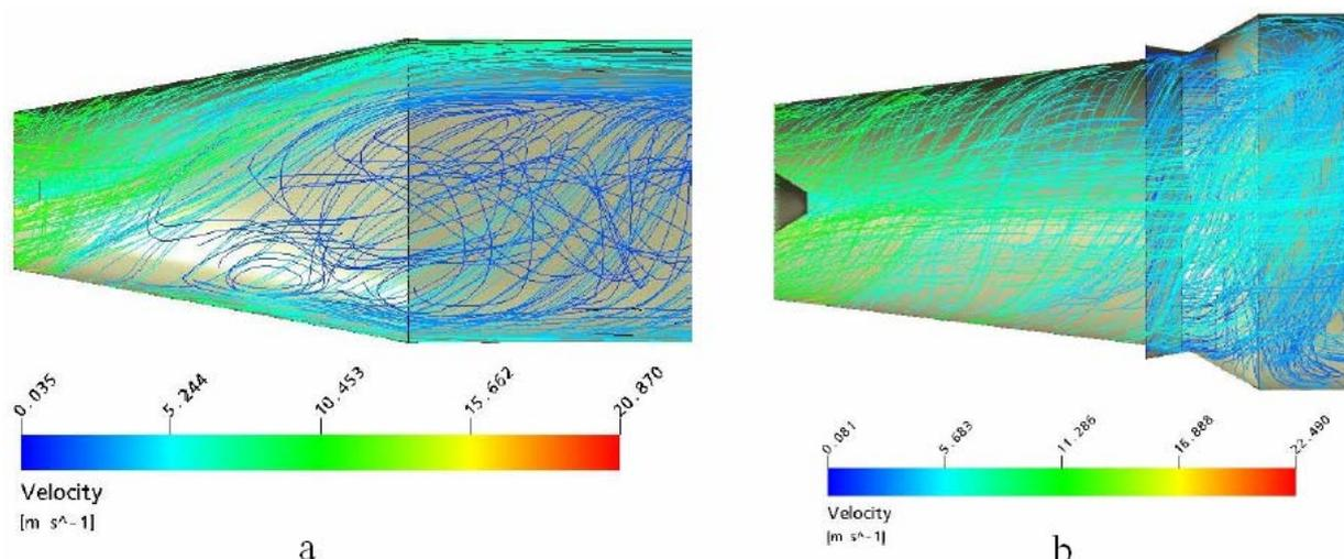
Figure 6. Stream line in the draft tube without secondary entrances and length equal of the optimized (a) and stream line in the optimized draft tube (b)
