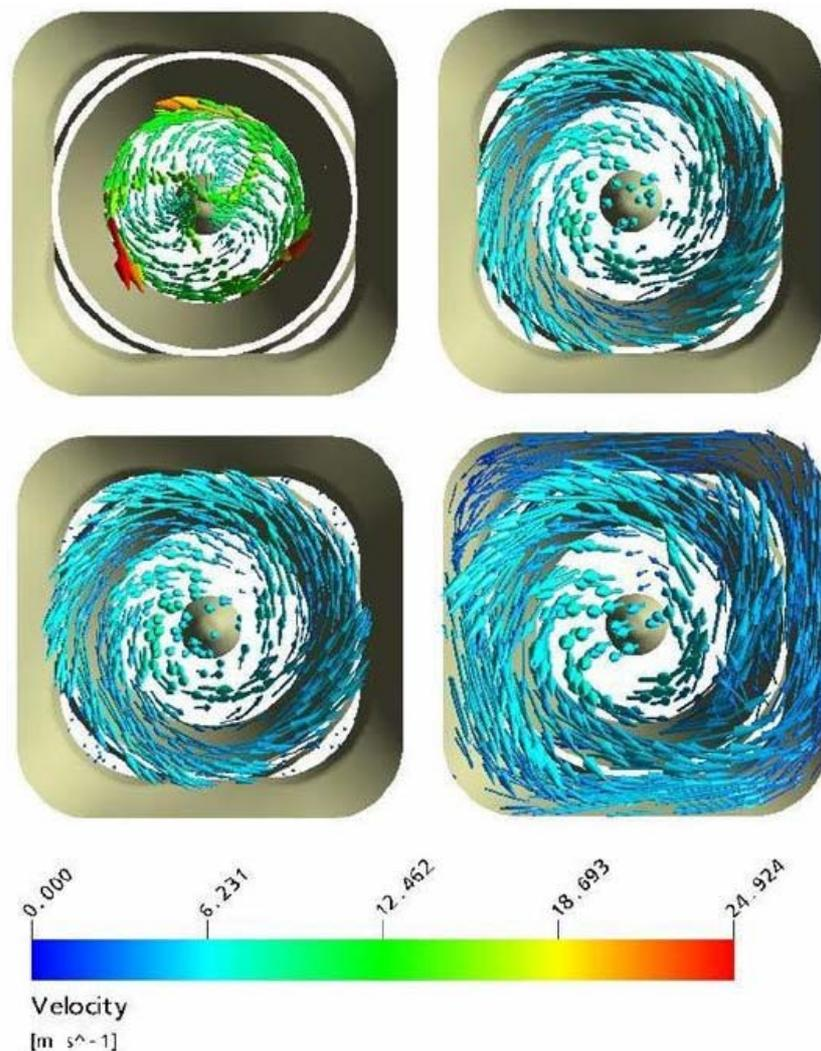
Figure 8. Evolution of the flow of the optimized draft tube, in the inlet, to 15m, to 17m and 20m
