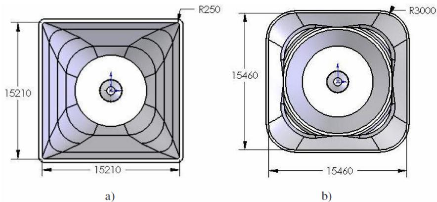
Figure 5. Comparison among the conventional outlet the draft tube (a) and the outlet used in the optimization of the same (b). The values are in mm
