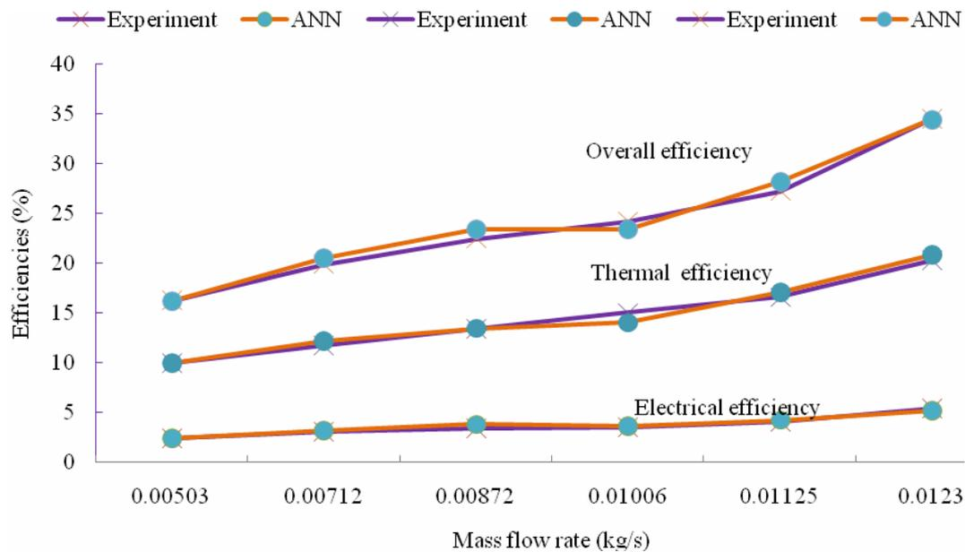
Figure 13. Comparison of electrical, thermal, and overall efficiencies (Experimental and ANN predicted)
