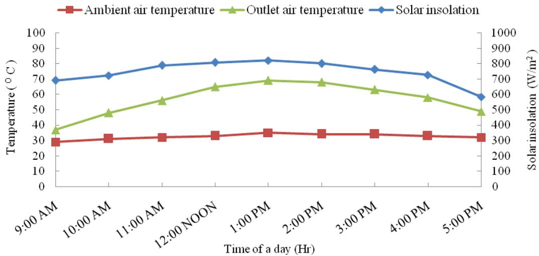
Figure 7. Hourly variations of solar radiation, ambient air and outlet air temperatures (1<sup>st</sup> February 2011)
