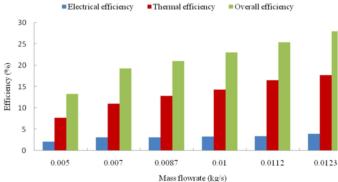
Figure 12. Typical variations of electrical, thermal and overall efficiencies with mass flow rate of air
