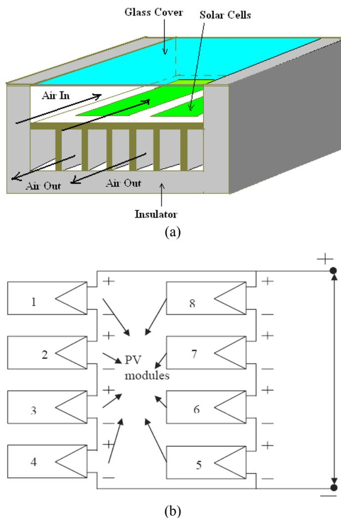
Figure 1. (a) Schematic diagram of DPHSAH with slats; (b) Schematic representation of PV module connections
