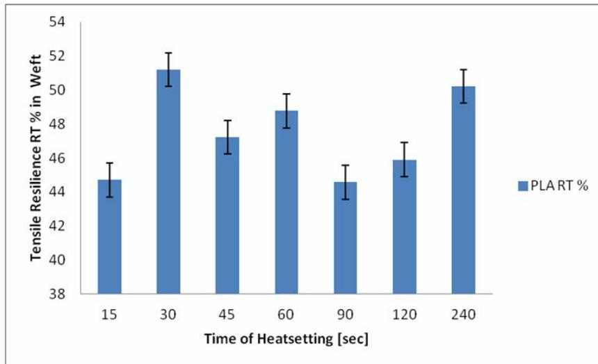
Figure 13. Effect of time of heatsetting on tensile resilience RT [%] in weft direction
