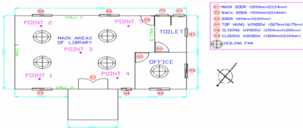
Figure 2. Building plan and the node points for instrumentation
