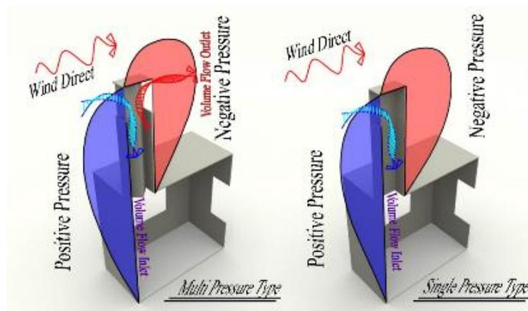
Figure 13. The utilization of Multi pressure type and Single pressure type of traditional wind catcher of high pressure areas around cage
