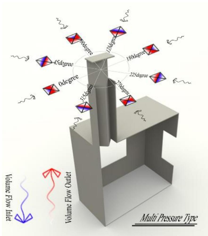
Figure 11. Direction of the airflow inside the multi pressure type of wind catcher in different angles blowing
