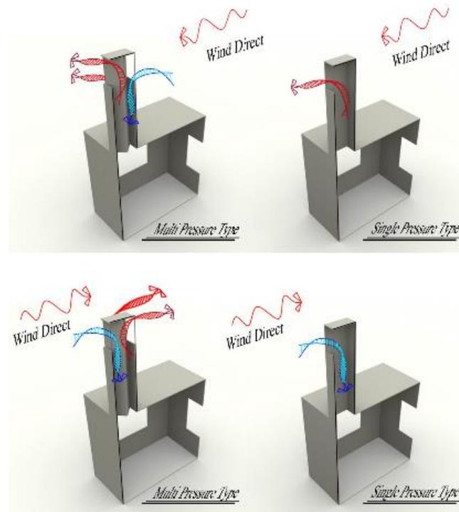
Figure 12. Behaviors of Multi pressure type and Single pressure type of traditional wind catcher in different angles blowing
