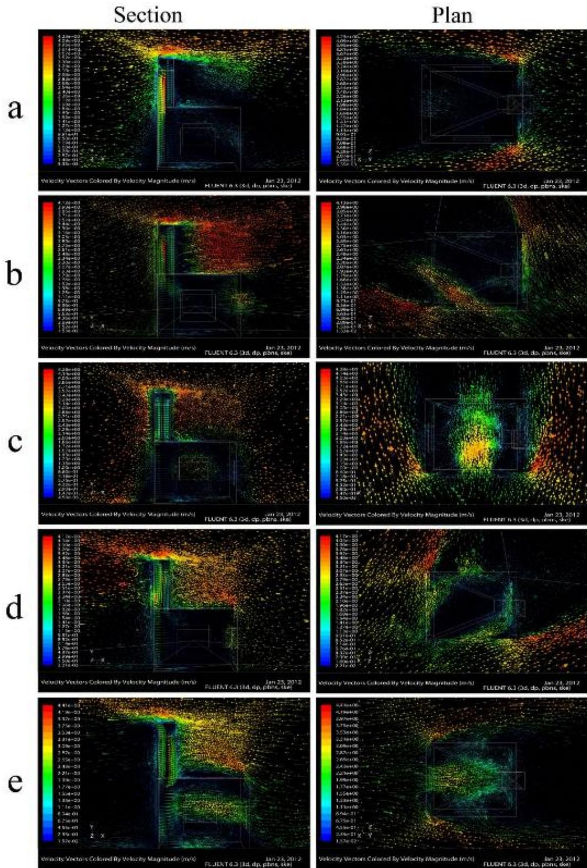
Figure 10. Sections and plans of vectors of velocity magnitude of multi pressure wind catchers in different directions blowing
