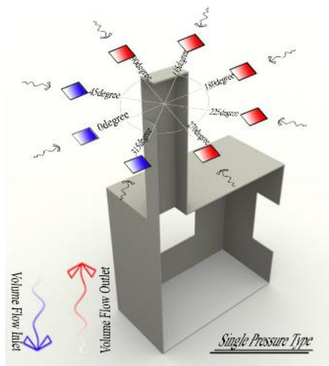
Figure 9. Direction of the airflow inside the single pressure type of wind catchers in different angles blowing
