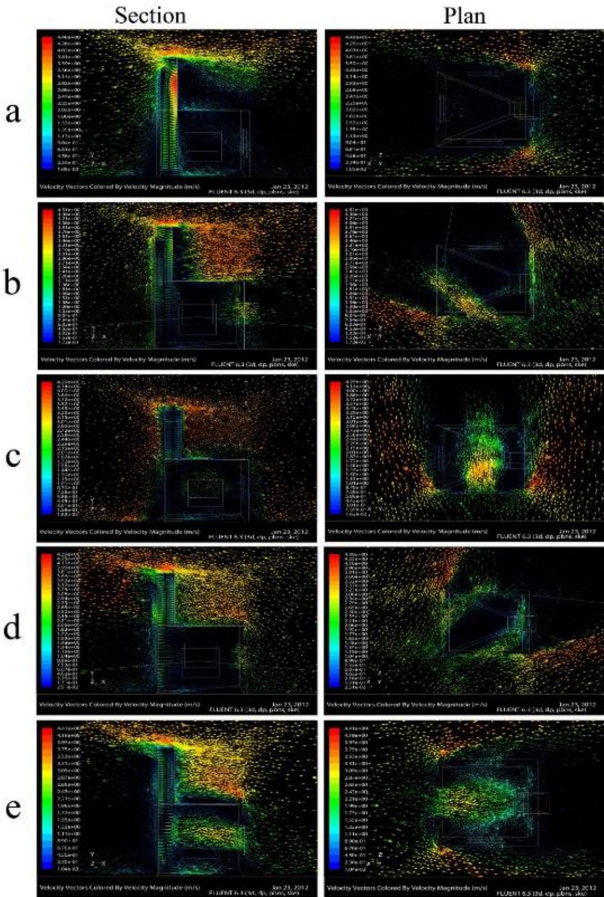
Figure 8. Sections and plans of vectors of velocity magnitude of single pressure wind catchers in different directions blowing
