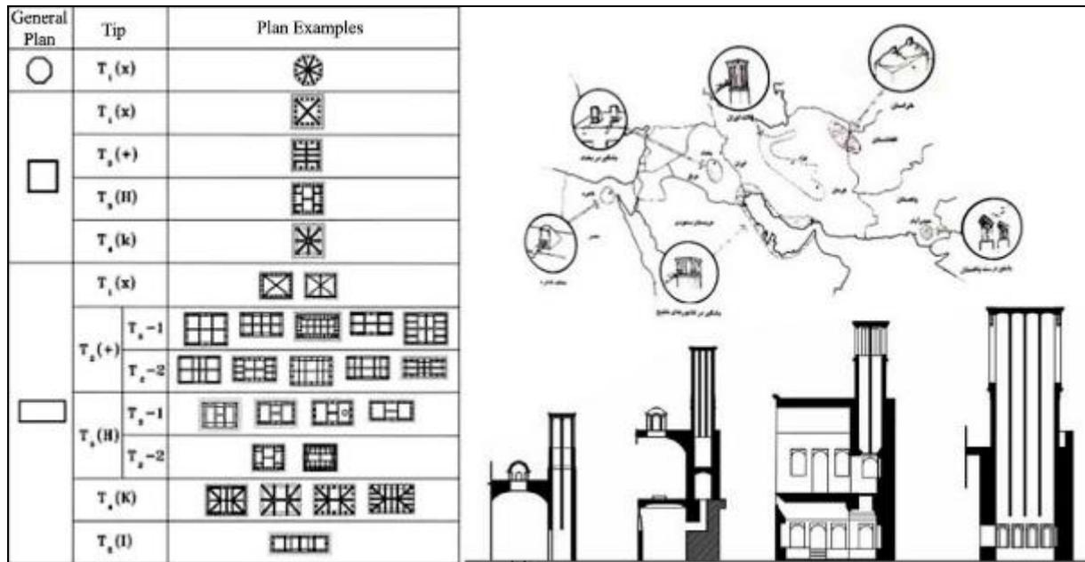
Figure 2. wind catchers' dispersal [10] and cross-section and plan typology of Multi pressure type [20]
