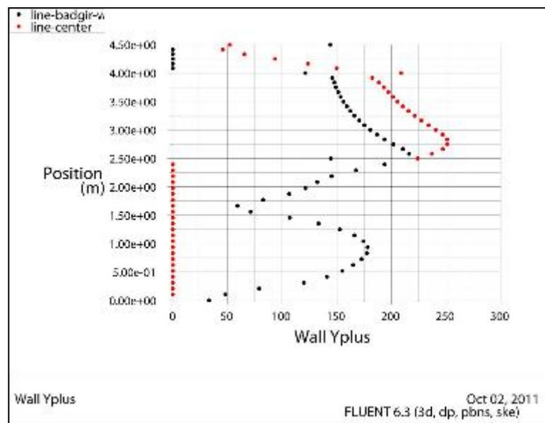
Figure 7.  $Y^+$  chart near the outer wind catcher wall and the inner blade center
