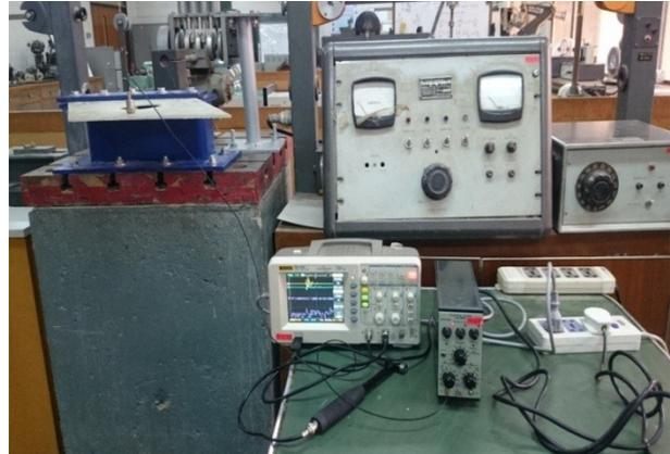
Figure 4. Cantilever skew plate test rig.
