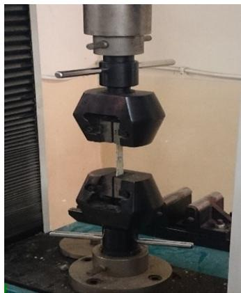
Figure 2. Tensile test machine
